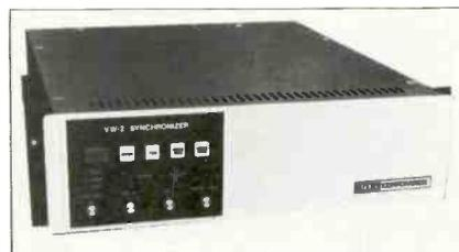
processing; vertical blanking control adjustable between 15 and 21 lines; horizontal blanking fixed at 10.8  $\mu$ sec; and velocity compensation in the synchronize and heterodyne TBC mode. The unit is capable of delaying non-synchronous video feeds by as much as a full frame to make them synchronous with the station reference. In TBC mode it can perform simultaneous time base correction and synchronization.
