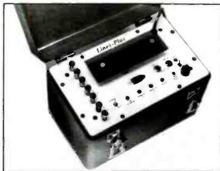
include two-way signalling for cuing or other slow speed data and greatly improved line reliability resulting from patented and patent-pending circuitry. The transmitter unit weighs about 10 pounds. KAHN COMMUNICATIONS.
