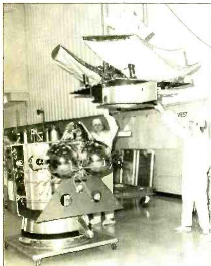
Engineers lower feedhorns and antennas onto RCA's newest commercial communications satellite
