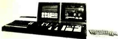
bubble memory (for up to 700 cues) and proportional electronic patching (for 32 to 320 control channels and 32 to 9216 dimmers). Two Color Graphic monitors provide an interactive display of patch and playback information in a clear, concise layout. Features include level setting by keypad or encoder and cue command functions of fade times, fade delay, auto-sequence, dimmer slope, and operator messages. KLI EGL BROTHERS.
