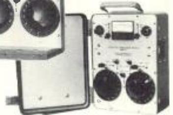
The **Operating Impedance Bridge** measures the impedance of networks, radiators, and the like while they operate under full power. VSWR as well as complex impedances of up to  $400 \pm j300$  ohms can be measured.
