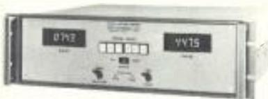
The **Digital Antenna Monitor** couples pushbutton ease of operation with digital accuracy. The DAM-1 will accept RF samples from up to 12 towers (with an auxiliary panel) and features  $\pm 1^\circ$  phase and  $\pm 2\%$  current ratio accuracies. Remote panels and other accessories are available.
