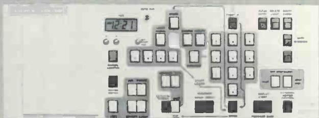
Model 7200 AUTO DRIVE™ Computer controller. Plug compatible option for 6112 and 6124 switchers stores 255 events which can be grouped into any number of sequences. Each event has a maximum duration of 99 minutes: Frame accurate. Production tool which enables complex effects to be run in rapid sequence. Drastically cuts down editing time. It also interfaces with editors. Price N.T.S.C. \$12,500. PAL \$13,500.
