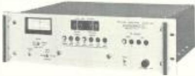
The **Amplitude Modulation Controller** is the only modulation controlling system that provides a completely closed loop around the transmitter. The sampling of actual modulation levels after the PA output network assures precise adjustment for optimum modulation levels. The AMC-1 also keeps a digital count of positive and negative overmodulation bursts for both present and previous one minute periods.
