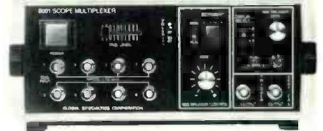
view a single channel by switching to manual mode and choosing the desired display. In operation the signal which is to serve as the trigger is connected to channel one. Trigger level is variable.
