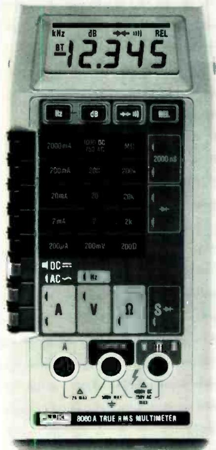
measurements for ac signals to 100 Hz, frequency to 200 kHz, and resistance measurements to 300 megohms. It also has the ability to store any measurement as a positive or negative relative reference value. Voltage is displayed in dBm, referenced to 600 ohms or in relative dB. Continuity testing, conductance, and constant current source diode testing functions are also included.
