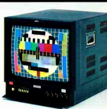
And you can choose from medium, standard or high resolution delta dot tubes. All models are fully modular. The medium resolution CM-33 HRB offers a phosphor triad pitch of .43 millimeters and the CM-51 HRB .47 millimeters. Other features include switch selectable scan/overscan and an RG off switch for easy set-up.
