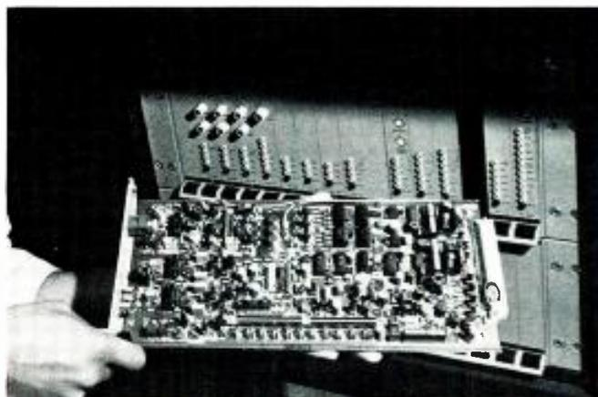
A servo control board from the Bosch FDL-60 film-to-tape transfer system.
