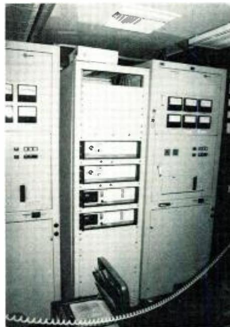
Control area of the truck where transmit/receive functions are executed.
