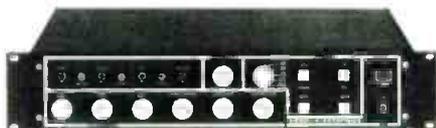
ment. Picture coring for luminance noise reduction and RGB decoding and re-encoding for correction of optical color errors are also standard, as is a built-in switcher fader for adding camera titling. The unit is priced under \$4000.
