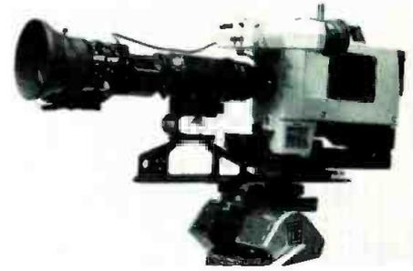
white phosphors for contrast resolution. It combines the features of a 25 mm format and high-gain, second generation image intensification into a compact unit. It is compatible with most major cameras by selecting the appropriate adaptor.
