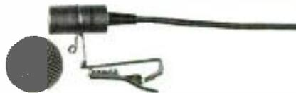
Electret condenser lavalier mics like SONY's ECM-50 have proven useful for on-camera miking situations because of their reduced size. And while many of these mics offer good performance in a compact size, the Beyer MCE5 also provides extended frequency response (20 to 20,000 Hz) and durability in an even smaller format (diameter: 7 mm / length: 23 mm).
