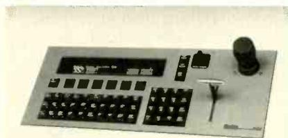
Control panel for new Abekas efx processor.
