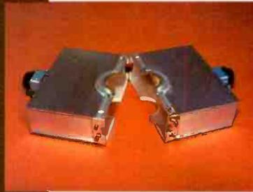
EEV was first to produce a high power (45-58 kW) wide band external cavity klystron to cover the whole UHF TV spectrum. What is more, instead of 6 different tubes, now only one is needed for either water or vapor cooled applications. This also applies to EEV's medium (30 kW) and low power (15 kW) klystrons - which all means a substantial saving in spares inventory!
