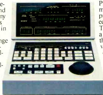
Practices for Digitally Controlled Equipment." Which means the interfacing problems between video, audio and film equipment will be problems of the past. This Sony "Sync Master" synchronizer has a built-in distributed intelligence network that makes it able to talk to an entire universe of diverse machines developed by diverse manufacturers.
