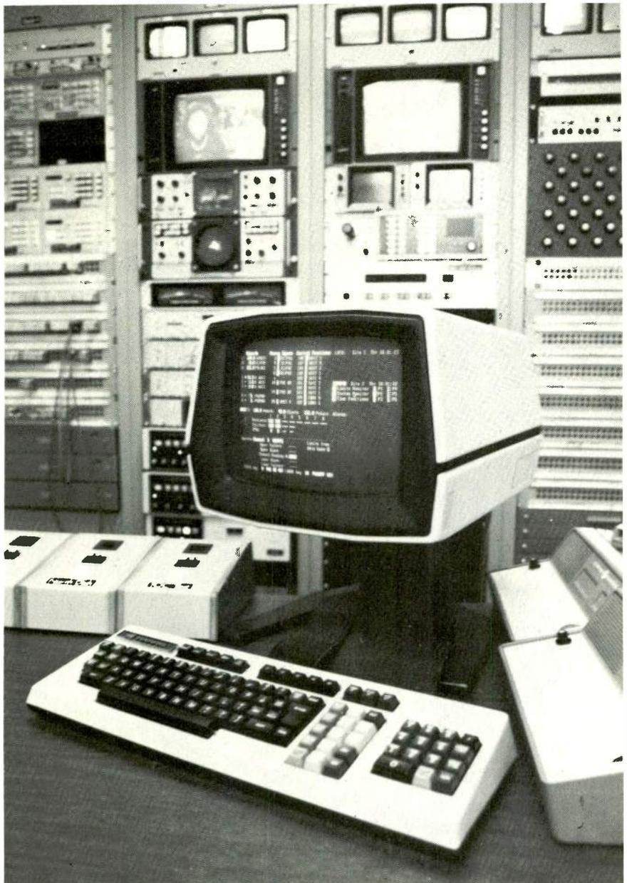
At Metromedia's satellite complex in Hollywood, a Harris 9165 earth station facilities controller runs three separate earth station antennas that serve outside customers as well as Metromedia radio and television stations.
