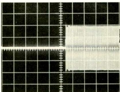
Fig. 1 Cue output with air dashpot set for 105 ms. start delay (Sweep = 20 ms./div.)
