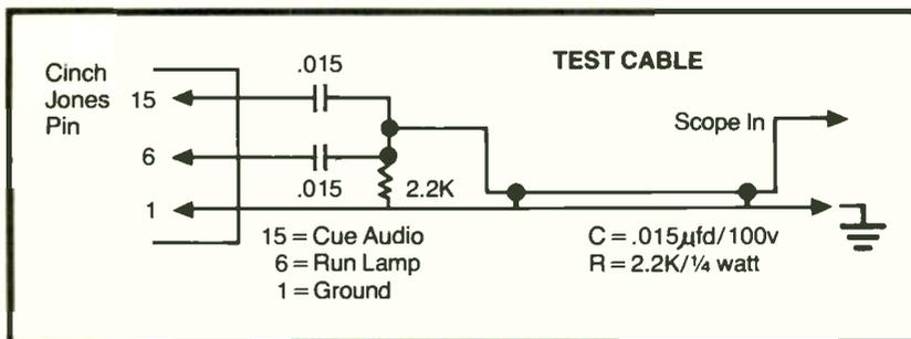
In a large broadcast facility using many cart machines, quite a lot of time is spent in insuring that the operating parameters of the various machines are all consistent. One variable often overlooked, however, because it seems more difficult to measure than others, is the actual pull-in time, or the period that elapses between the time the start command is sent to the cart machine and the time the audio starts.
