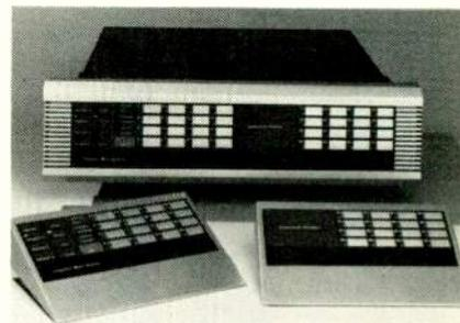
The Model 200 Smart Switcher is a new audio routing/mixing system from Integrated Media Systems. It is configurable in matrixes of eight, such as 32x8, 8x32, 16x16, and so forth, in one 5.25-inch frame including power supply. The matrix configuration can contain up to 256 crosspoints per frame, and it can be expanded up to 128x128, with up to 32 control stations.
