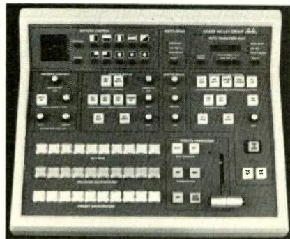
effects system structure in the 100 eliminates much of the button pushing and operator logic required to create the same effects on the current generation of small two mix/effects switchers.
