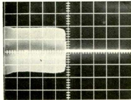
Fig. 3 Cue Output when machine stops. (Sweep = 10 ms./div.)
