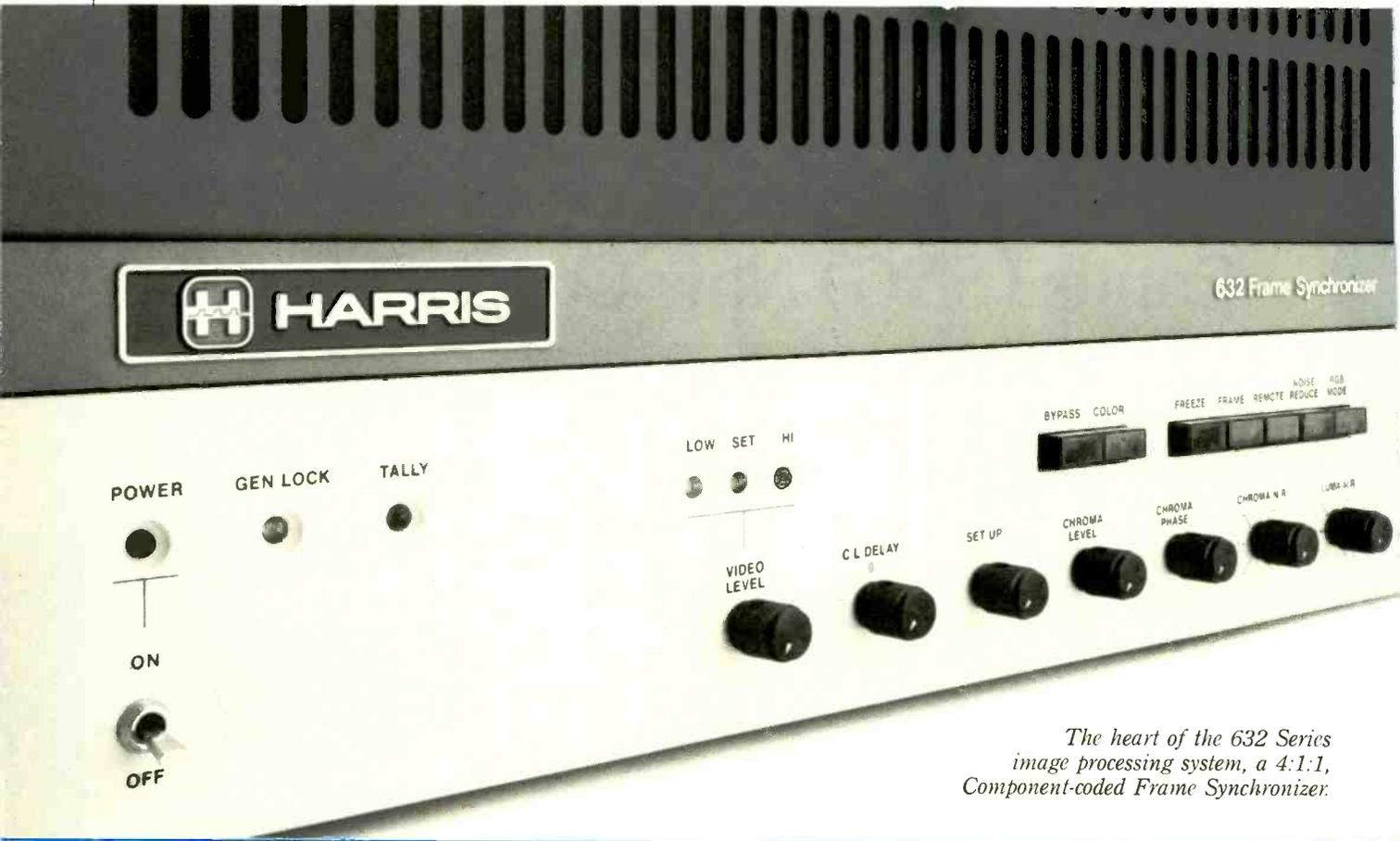
*The heart of the 632 Series image processing system, a 4:1:1, Component-coded Frame Synchronizer.*
