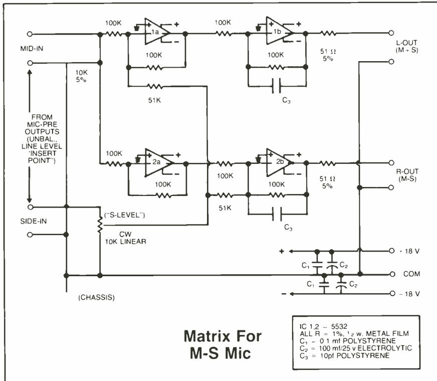
Another flexibility lies in the fact that the M and S outputs can be recorded directly, without going through the matrix. Then the stereo can be produced in post-production, allowing the
