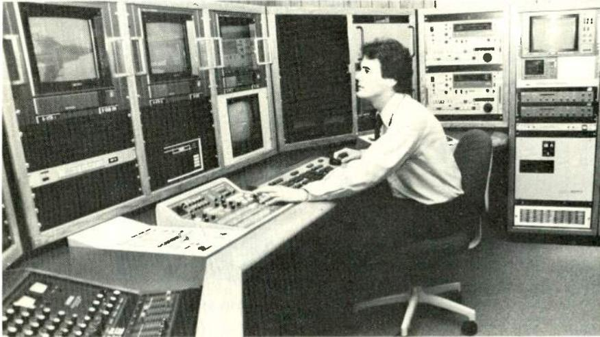
ISC Technologies' new computerized editing suite features the Paltex Editstar computerized editor, Hitachi HR-230 one-inch, two Sony BVU 800s, Chyron RGU-2, Harris HDE-100 digital effects unit, and Yamaha's M512 audio mixer.
