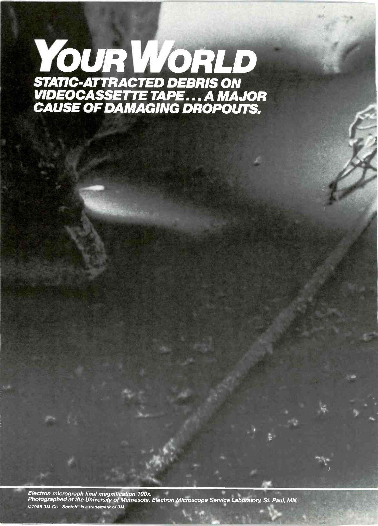
An electron micrograph showing a dark, textured surface, likely a video cassette tape, with various small, bright, irregularly shaped particles (debris) scattered across it. The background is dark and grainy, with some faint, larger-scale patterns visible.
