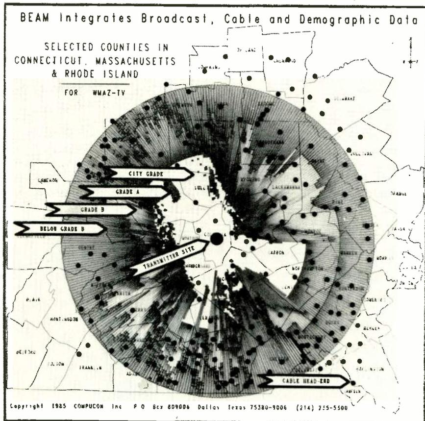
Compucon's BEAM service shows a computer-drawn map detailing broadcast, cable and demographic data.
