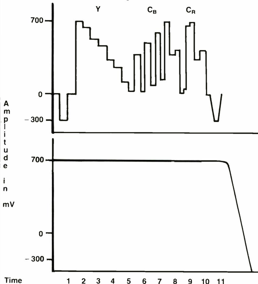
Figure 4. Waveform and spectrum for the time division multiplex (TDM) form of analog components, S-MAC. It consists of Y compressed 2:1,  $C_B$  compressed 4:1, and  $C_R$  compressed 4:1. The  $C_B$  and  $C_R$  portions of the waveforms are derived from  $P_B$  and  $P_R$  by offsetting their baselines to +350 mV. The time compression yields a bandwidth of 11 MHz.
