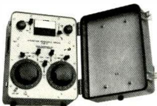
The OIB-3 Operating Impedance Bridge provides extended resistance and reactance ranges, measuring up to 1000 ± j900 ohms. The bridge has a built-in carrying case and RF amplifier for improved nulling.
