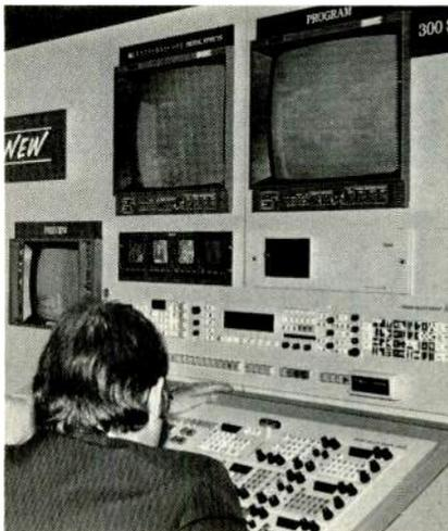
CVG Kaleidoscope installed in 300 switcher.
