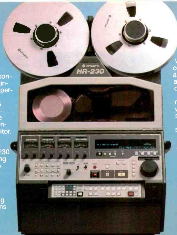
air scanner system dramatically reduce head and tape wear. It's compatible with all major editing systems. And such features as master/slave operation of up to 43 VTRs through its built-in editor, complete autoseup, pre-aligned replacement scanner, and a built-in TBC save you a lot of time and trouble.
