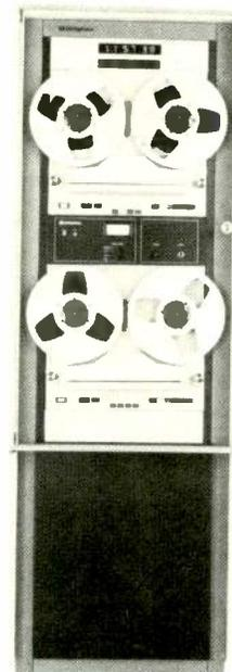
The Dictaphone 5600 Veritrac™ voice communication recording system is a complete broadcast recording-retrieval system that lets your radio station keep its entire broadcast day on the record. In one dependable unit you get around-the-clock verification that you're running your advertiser's spots on schedule and meeting all your FCC requirements. So if they ask for proof, you've got it all there on tape, ready for quick retrieval and replay.
