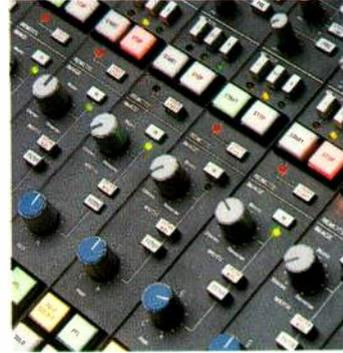
Options include Total Recall™ — an SSL exclusive, completely independent of the audio path, which allows any operator to recreate the most intricate console setups for any programme with rapid accuracy, week after week. Programmable dynamic stereo equalisation and panning may also be added, along with
