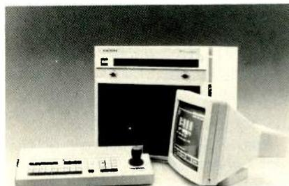
Microtime's RP-1 digital video effects system features rotation with three variable axes and internal key with soft edge.
