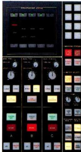
Options include Total Recall™ — an SSL exclusive, completely independent of the audio path, which allows any operator to recreate the most intricate console setups for any programme with rapid accuracy, week after week. Programmable dynamic stereo equalisation and panning may also be added, along with
