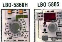
**LBO-5860H** allows selection of lines 7 to 21. **LBO-5865**, designed for camera and pickup device testing offers full 525-line selection with memory preset/recall of any three lines.
