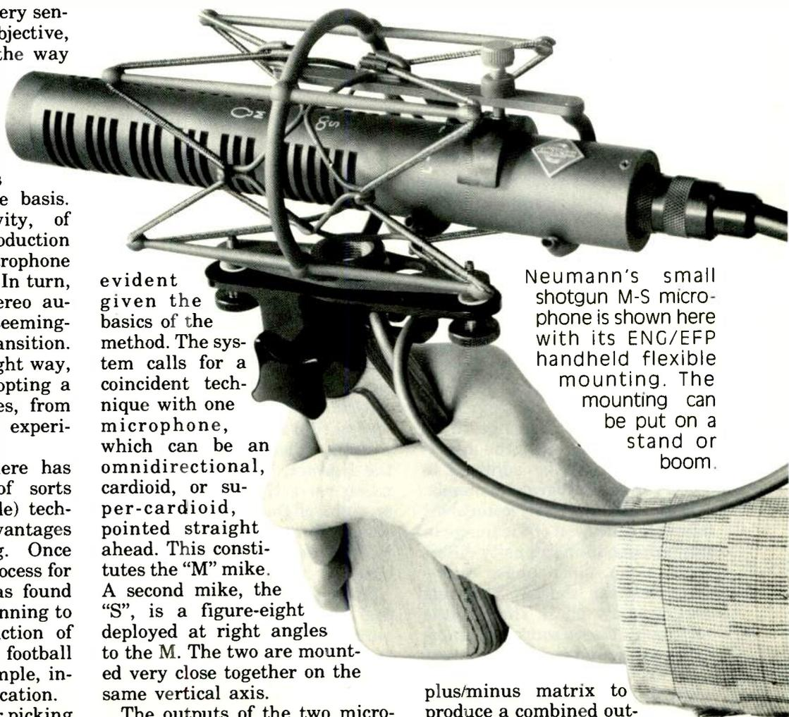
Neumann's small shotgun M-S microphone is shown here with its ENG/EFP handheld flexible mounting. The mounting can be put on a stand or boom.
