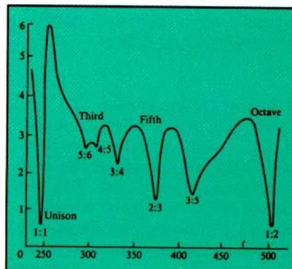
**Figure 5:** Dissonance expected from tone A with  $f = 250$  Hz and tone B with varying frequency.
