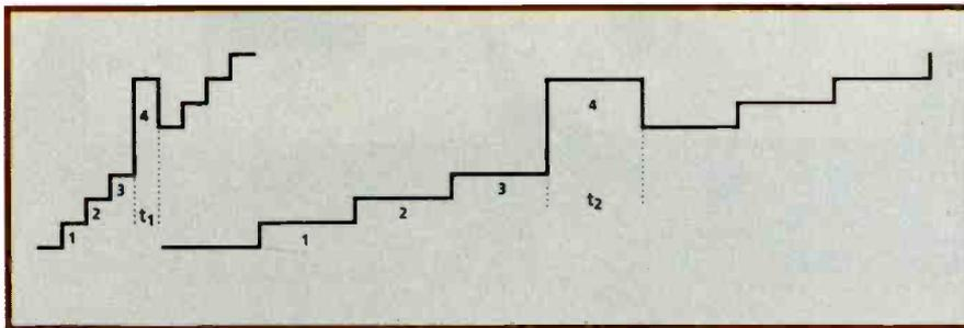
**Figure 10:** Differential nonlinearity at fourth step distorts the step ramp for only a short duration ( $t_1$ ) but distorts the shallow ramp for much longer ( $t_2$ ).
