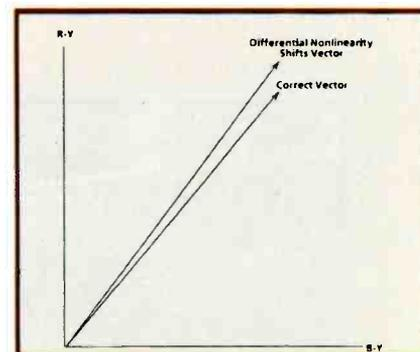
Figure 4: Differential nonlinearity error shifts phase and amplitude of chrominance sine wave. Result: hue and saturation error.
