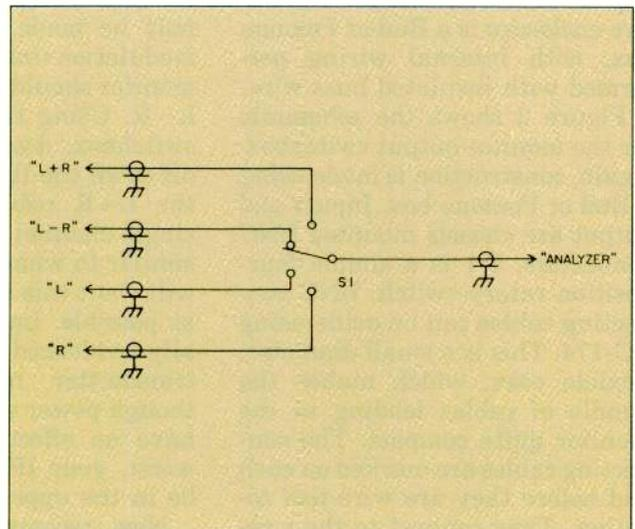
Figure 2: Monitor output select switch.
