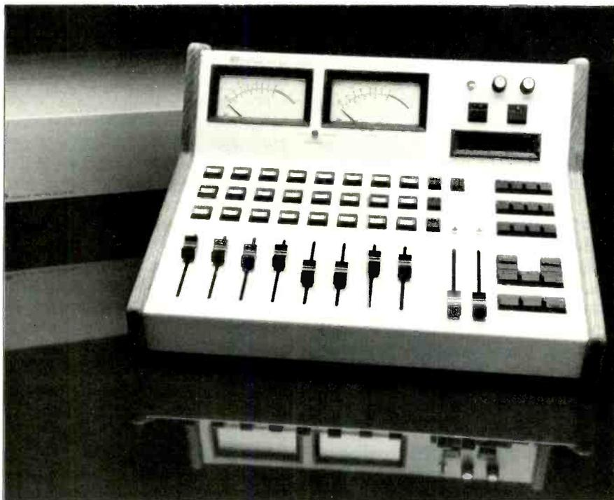
Graham-Patten's new compact 608 edit suite audio mixer houses audio signals in a separate electronics frame and interfaces with most video editors.
