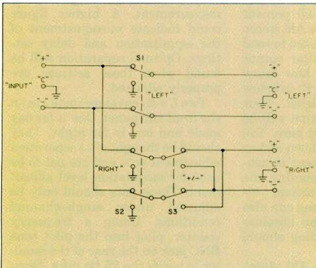
Figure 1: Switchbox schematic: oscillator switching unit.
