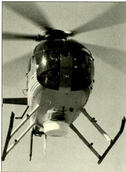
*A microwave-equipped helicopter (shown here with Nurad equipment) can relay signals from a remote site back to the receiver.*
