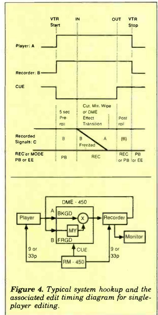
**Figure 4.** Typical system hookup and the associated edit timing diagram for single-player editing.
