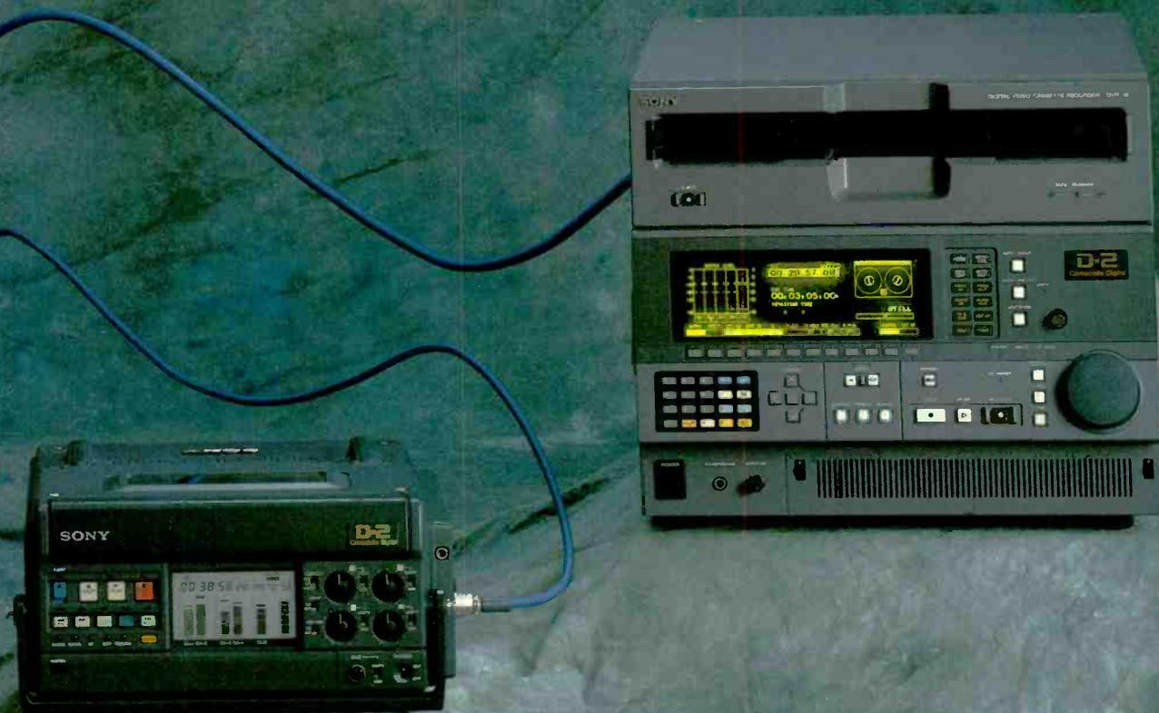
digital dubbing. Four channels of PCM digital audio. And write-after-read editing.
