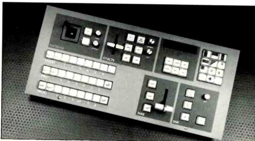
offers color wash and can mix to a wipe and fade DSK to black. Options include an RGB, NTSC or PAL color keyer and a SMPTE serial interface to most editors. List price is \$5995. Reader Service #217
