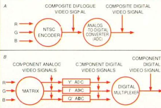
*Component coding is more complicated than composite, but provides greater freedom in signal processing.*
