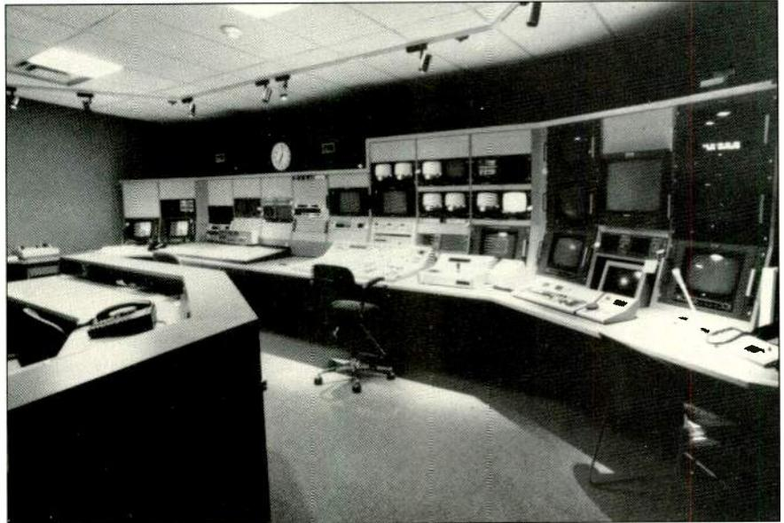
The BET edit room features GVG 200 switcher, 151 edit controller, and Sony MXP 2000 Series audio mixer. The room can function as a control room for studio production.
