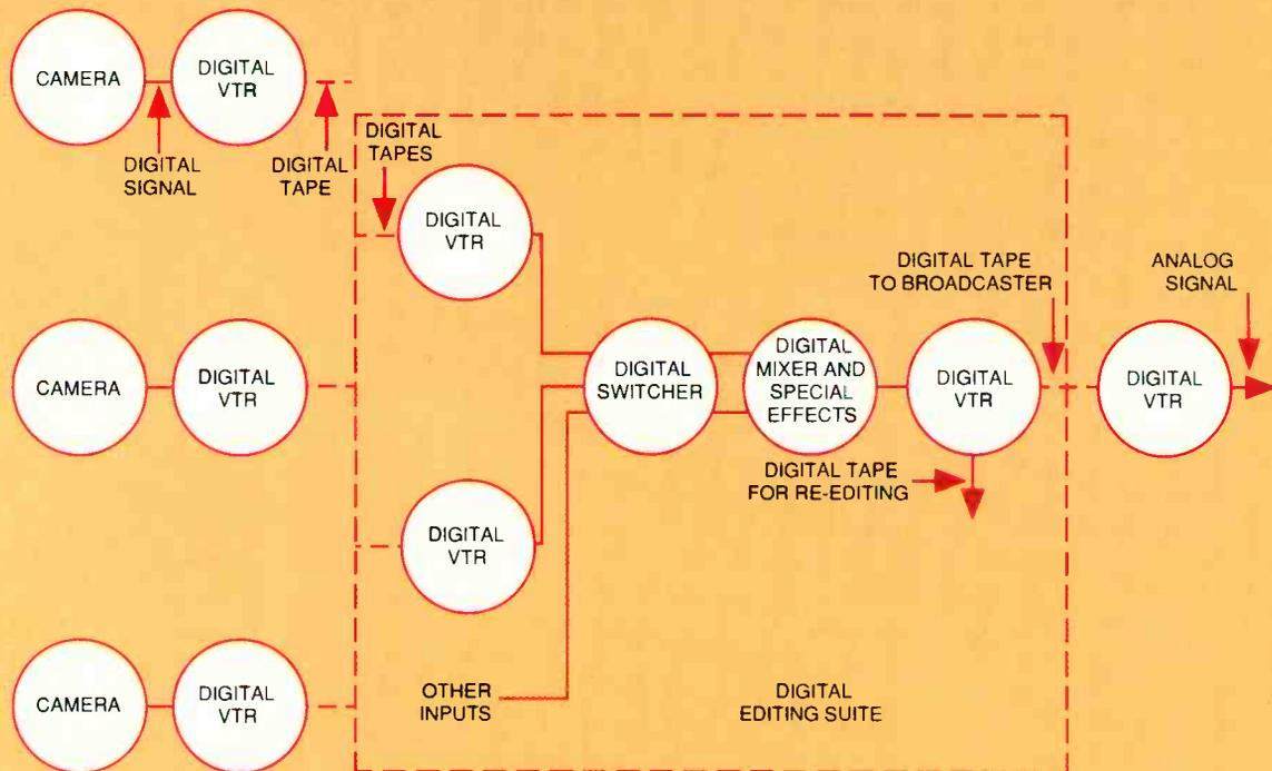
Method of signal flow in an all-digital edit system where source material is videotape from isolated cameras.
