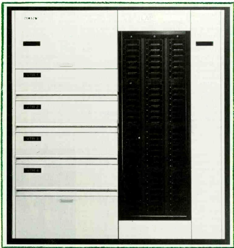
*Sony DVC-80 LMS features four D-2 digital VTRs for high-quality playback.*
