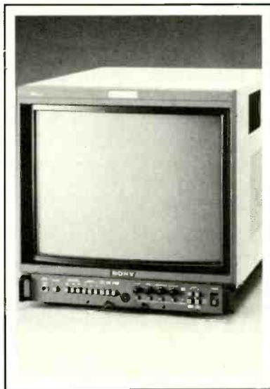
component RGB inputs, and an RGB frequency response of 100 Hz to 6 MHz. According to Sony engineering data, non-linear distortion and dynamic gain is less than five percent, and differential variations between RGB screens are less than one percent over a 500-hour period. Maximum brightness is 60 fL.
