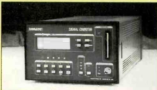
*signals. The Signal Creator's memory card unit allows creation of custom test signals for later playback.*
