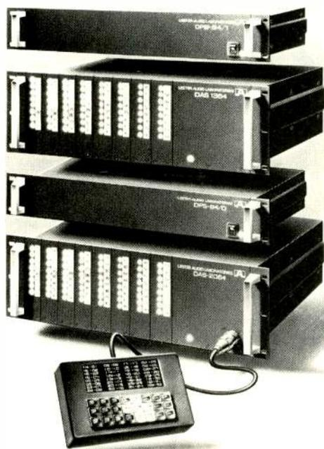
The DIGITAL AUDIO SYSTEM DAS 2000™ series from LAL is a fully integrated "smart" audio system. It provides multipoint-to-multipoint fiber optic sound transmission, distribution and routing with automated SOFT PATCH™ programmable memory control for both real time and pre-programmed changeovers.
