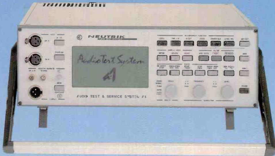
The A1 audio test system is the only instrument providing the capabilities of 7 separate pieces of equipment: sweep generator, level frequency, cross talk, noise, distortion, wow and flutter, curve tracer and an audio measurement oscilloscope. Communication and hard copy available through RS232 interface or centronics port. Accuracy and reliability that is portable for the audio lab, broadcast, manufacturing, service and studio user.
