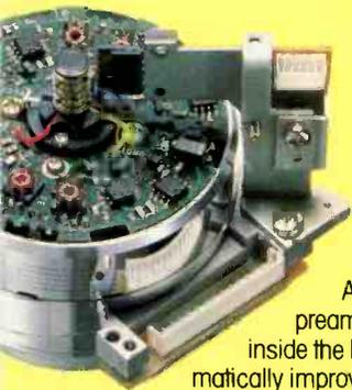
A new low-noise preamplifier mounted inside the head drum dramatically improves the signal to noise ratio and eliminates transmission loss.
