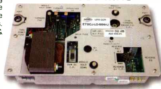
750 MHz Line Extender Upgraded to 860 MHz No Re-Spacing Required
