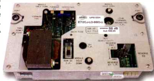
750 MHz Line Extender Upgraded to 860 MHz No Re-Spacing Required
