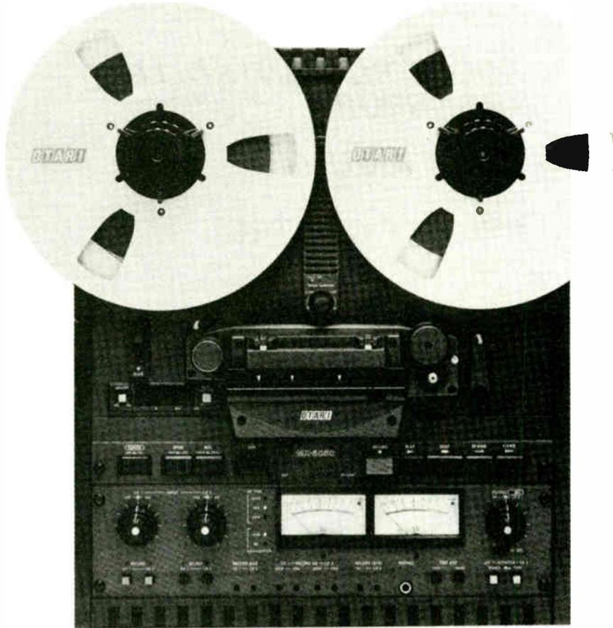
The Otari 5050 B-II is a compact recorder in the 1/4" two channel format. The optimized three head design and transformerless balanced inputs and outputs provide superior frequency response, distortion and signal-to-noise performance under professional studio conditions.
