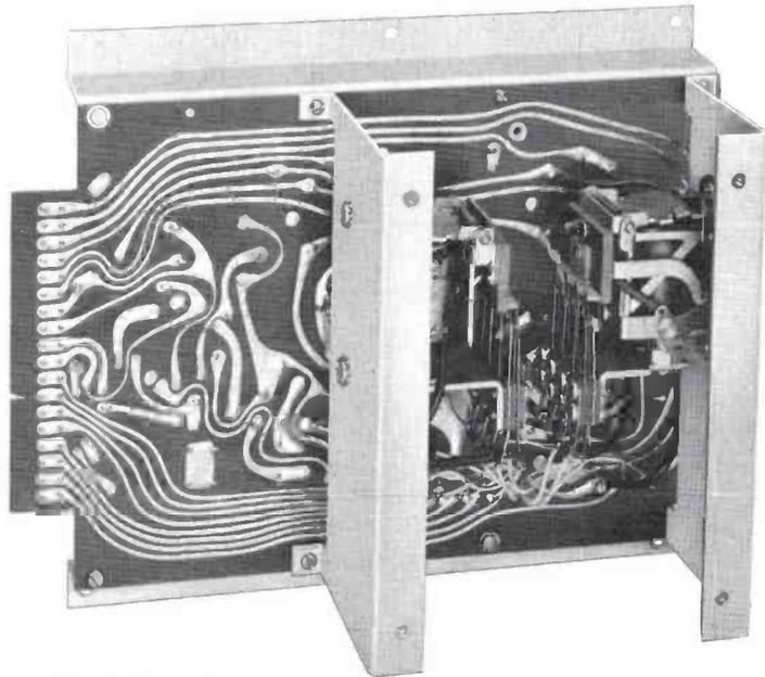
FIG. 7. The underside of the oscillator chassis is shown here. The relays are used to switch the crystals. Etched wiring simplifies servicing and also helps to improve oscillator stability.
