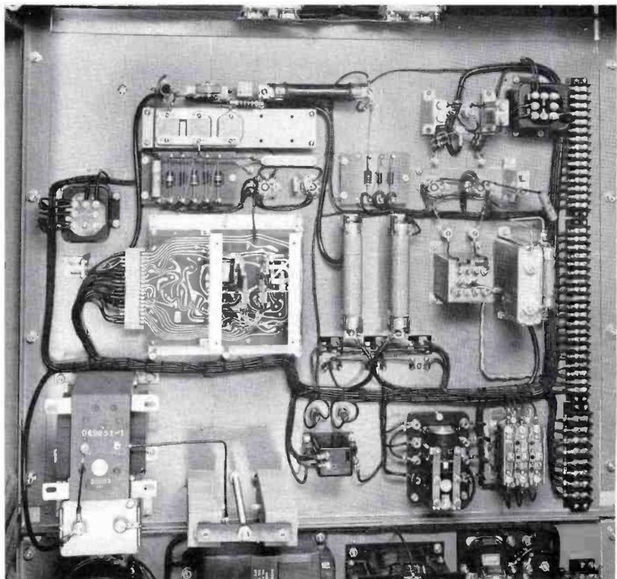
FIG. 8. The entire oscillator subassembly is shown from the rear. Vertical construction provides ease of maintenance. The oscillator chassis is easily removed with six thumbscrews. Note the convenient plug-in terminal strip on the oscillator chassis.
