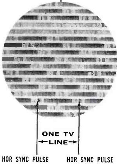
FIG. 1. Display of actual tracks as recorded by the RCA Color Video Tape Recorder.
