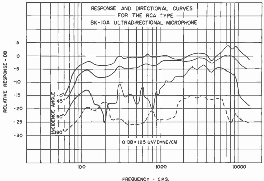
FIG. 3. The frequency response curves for the BK-10A are shown for various incidence angles of sound pickup.
