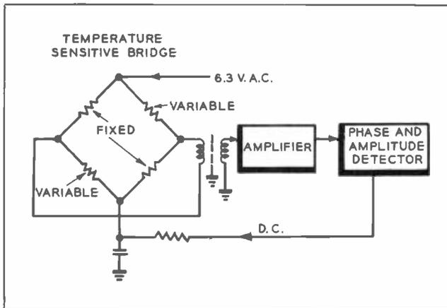
FIG. 5. Diagram of the oven-control circuit. Changes in ambient temperature unbalance the bridge and modify the power flow to keep the oven temperature constant.
