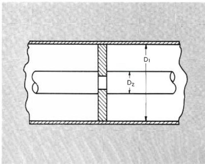
FIG. 4. Here is a cross section of an undercut insulator showing the spacing of inner and outer conductors.
