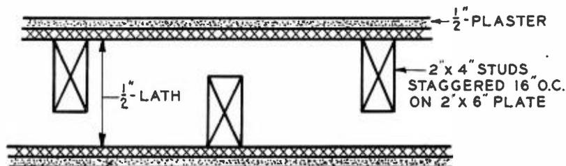
FIG. 1. This shows a cross section of a sound-insulating partition. Wooden walls should be constructed in this manner to reduce external noise.
