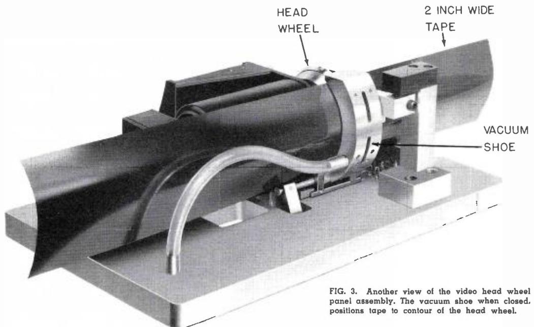
FIG. 3. Another view of the video head wheel panel assembly. The vacuum shoe when closed, positions tape to contour of the head wheel.
