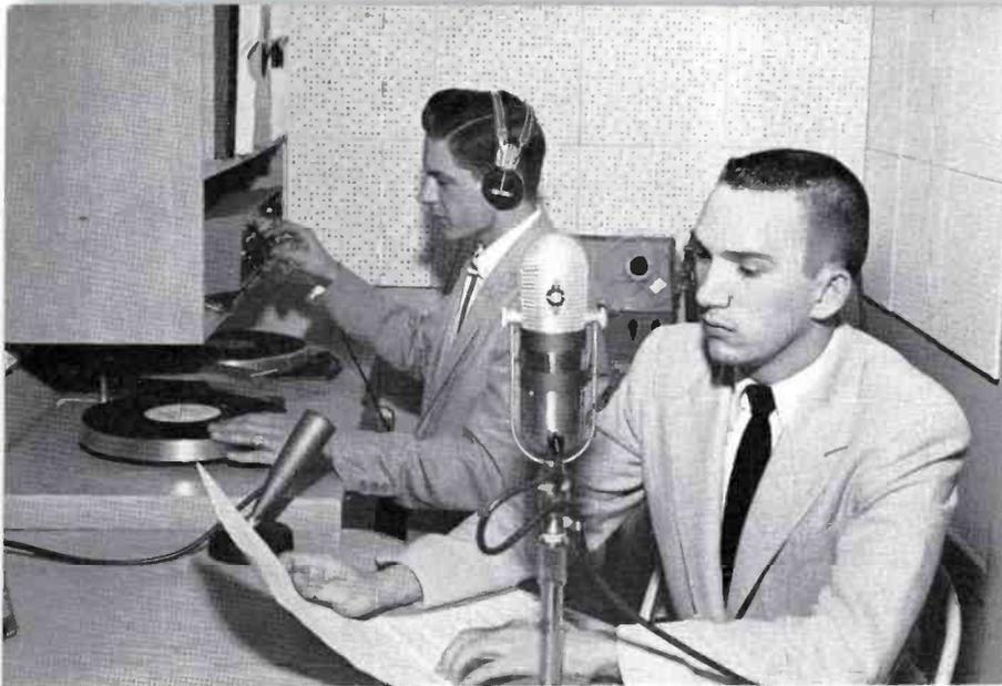
FIG. 9. Studio "B" (production studio) is being used to produce commercials and special programs. Left: Marvin Bredemier, Engineer, using Type BN-6A, 4-Channel Remote Amplifier. Right: Chuck Goodman, Newsman, recording special news features. The equipment is portable and can be taken out of the studio for special remote broadcasts, setup for any type.
