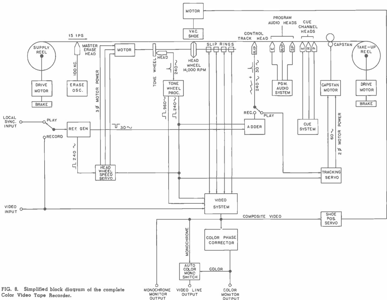
FIG. 8. Simplified block diagram of the complete Color Video Tape Recorder.
