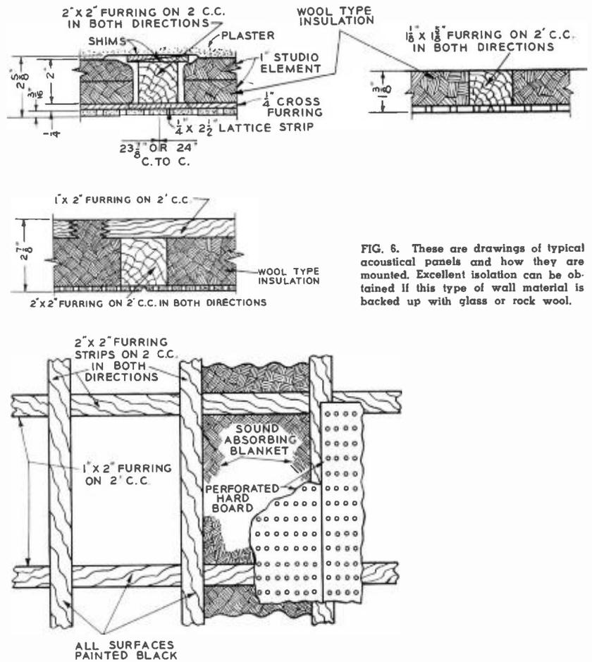
FIG. 6. These are drawings of typical acoustical panels and how they are mounted. Excellent isolation can be obtained if this type of wall material is backed up with glass or rock wool.
