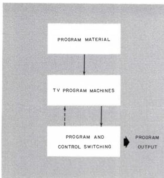
**FIG. 2. Flow diagram outlining conversion of program material to program output.**
