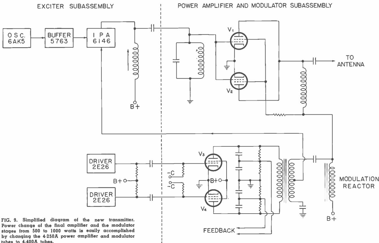
FIG. 9. Simplified diagram of the new transmitter. Power change of the final amplifier and the modulator stages from 500 to 1000 watts is easily accomplished by changing the 4-250A power amplifier and modulator tubes to 4-400A tubes.
