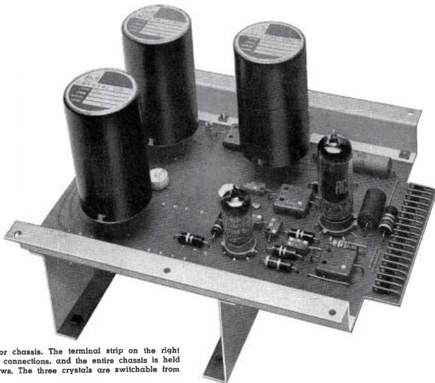
FIG. 5. This is the oscillator chassis. The terminal strip on the right contains all of the oscillator connections, and the entire chassis is held in place with six thumbscrews. The three crystals are switchable from a front panel control.
