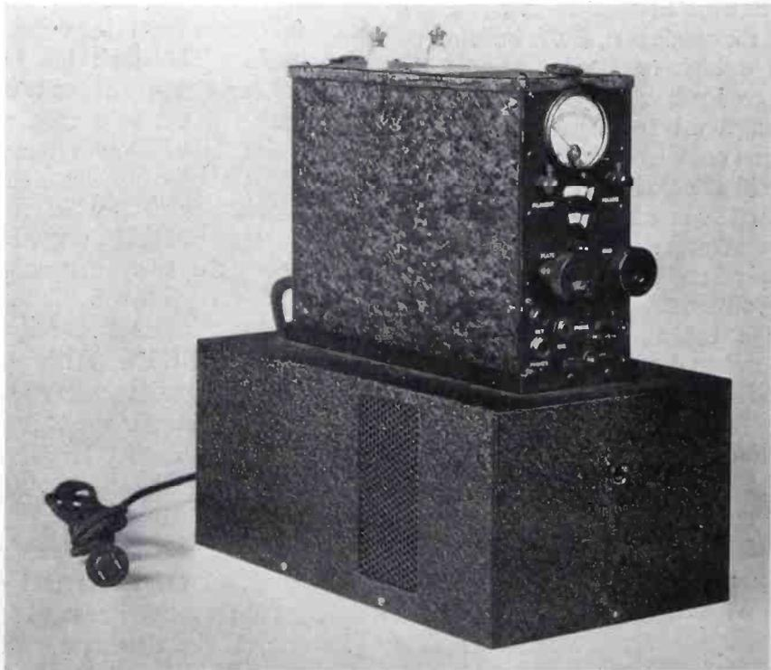
COMPACT RCA VICTOR "TERRA-WAVE" POLICE TRANSMITTER WITH POWER-SUPPLY UNIT IN BASE, AS SUPPLIED TO PORT JERVIS, NEW YORK. THESE POLICE RADIO TRANSMITTERS ARE PRODUCED IN A VARIETY OF SIZES, DESIGNED TO MEET THE REQUIREMENTS OF ANY SIZE TOWN OR CITY
