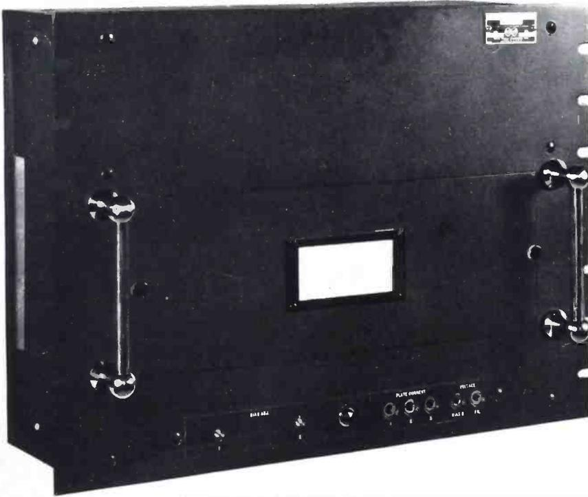
(RIGHT) REAR VIEW OF RCA VICTOR LINE AMPLIFIER, TYPE AA-4162. SHIELDING COVER REMOVED. NOTE ACCESSIBILITY OF COMPONENT PARTS
