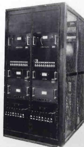
(ABOVE) A TYPICAL SPEECH CHANNEL LINEUP AT THE TOP IS THE LINE AMPLIFIER, TYPE AA-4162, IN THE CENTER IS THE TALK-BACK AMPLIFIER, TYPE AA-4164, AND AT THE BOTTOM IS THE STUDIO AMPLIFIER, TYPE AA-4163
