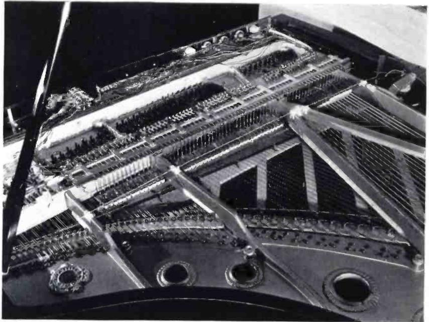
CLOSEUP OF THE INTRICATE MECHANISM OF THE MIESSNER ELECTRONIC PIANO
