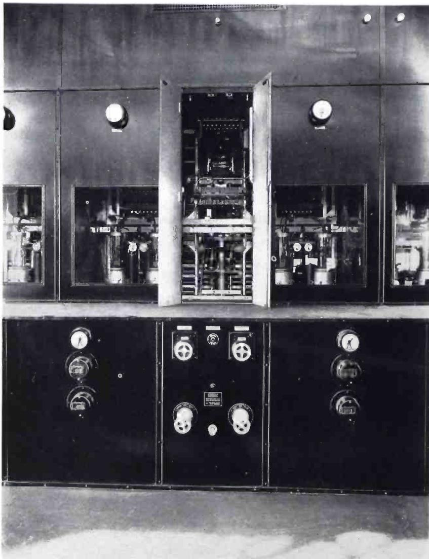
FRONT VIEW OF 170 KW POWER AMPLIFIER. THE LOWER PANEL CONTAINS THE THERMOMETER, WATER FLOW INTERLOCKS, VALVES, AND TUNING CONTROLS.
