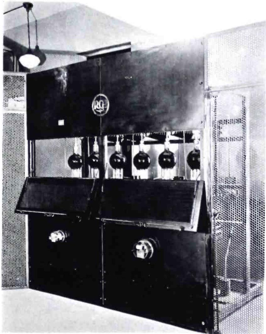
SIX TYPE UV-857 MERCURY VAPOR TUBES IN A TYPE 50-B 50 KW TRANSMITTER
