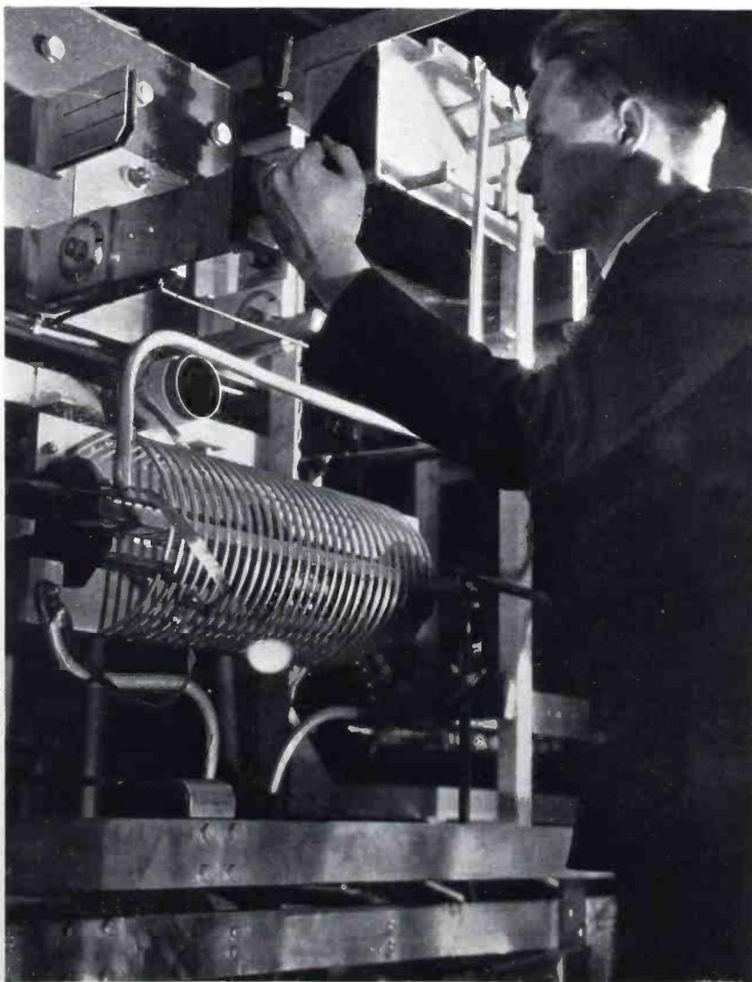
JOE CHAMBERS CLOSING A FILAMENT SWITCH IN ONE OF THE POWER AMPLIFIERS. NOTE THE GRID TANK COIL JUST BELOW HIS ARM.
