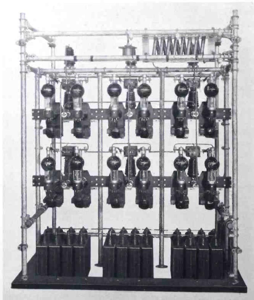
TWELVE TYPE UV-869 RCA RECTIFIER TUBES IN A TYPICAL ARRANGEMENT. THE RECTIFIER SHOWN CONSTITUTES PART OF A 40 KW SHORT-WAVE TELEGRAPH TRANSMITTER
