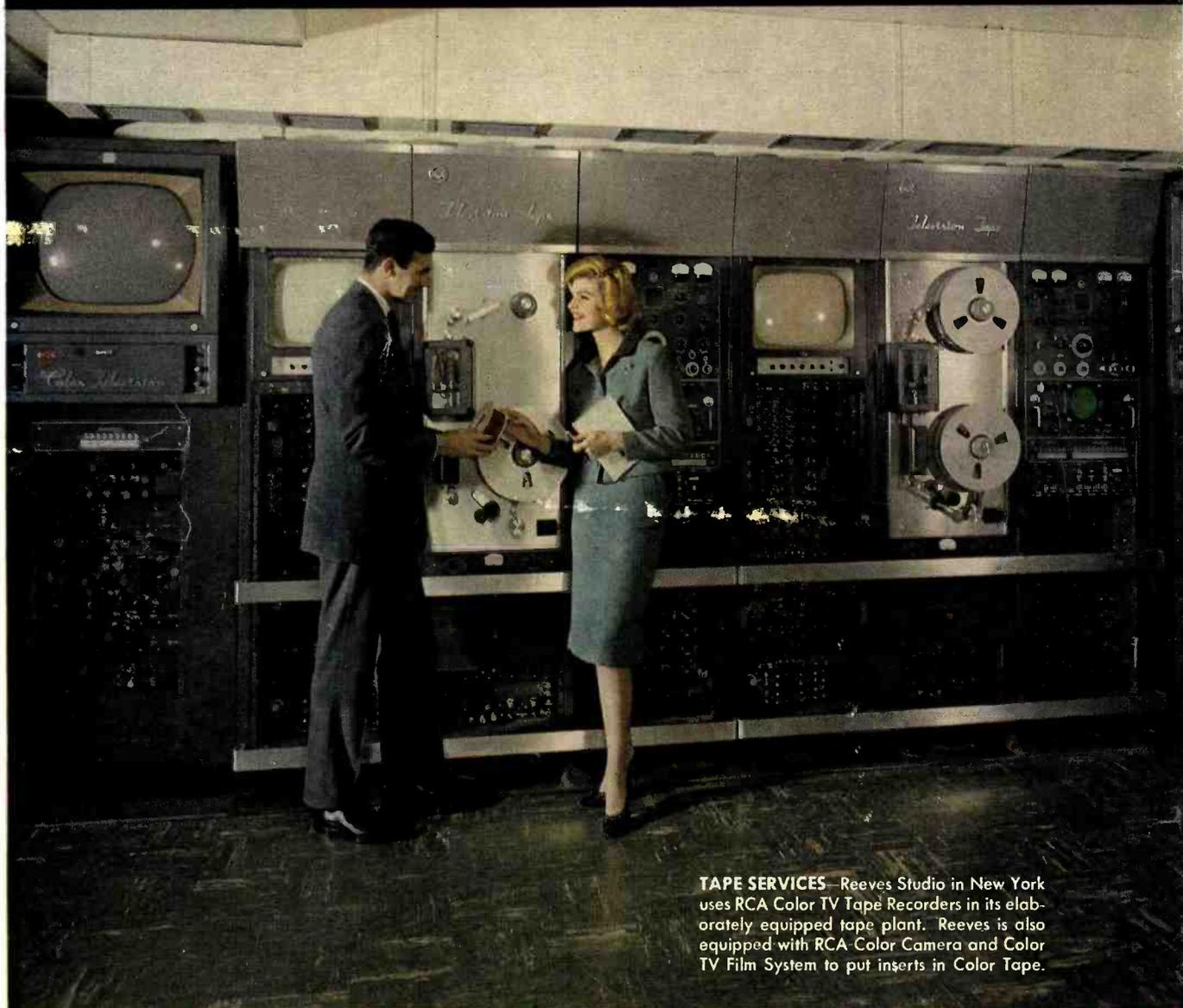
**TAPE SERVICES**—Reeves Studio in New York uses RCA Color TV Tape Recorders in its elaborately equipped tape plant. Reeves is also equipped with RCA Color Camera and Color TV Film System to put inserts in Color Tape.
