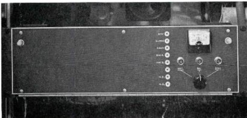
FIG. 7. The 2-speed converter panel, fully transistorized, mounts at the rear of the tape deck. Control circuitry required for conversion to 2-speed operation is an integral part of the TR-2 Recorder.
