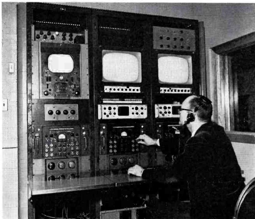
FIG. 20. WAVE-TV color control equipment for two TK-41 Live Color Cameras and one TK-26 3-V Color Film Camera. Engineer Jim Gardner is at the controls.
