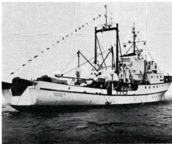
This view of Albatross IV shows two TV cameras in weatherproof housings on crossarms of research vessel's fore and aft masts.
