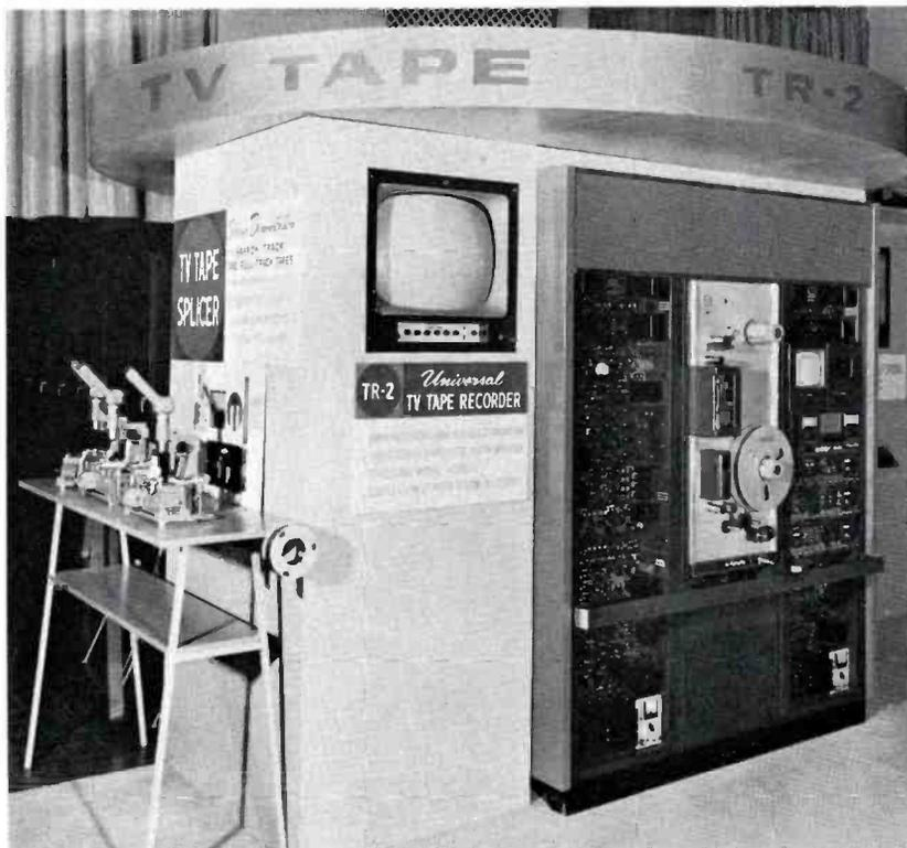
FIG. 5. A second TR-22 transistorized TV tape recorder was demonstrated in black-and-white operation at both half and full speed. Display at left provided pictorial comparisons of pixlock, automatic timing control and two-speed operation.
