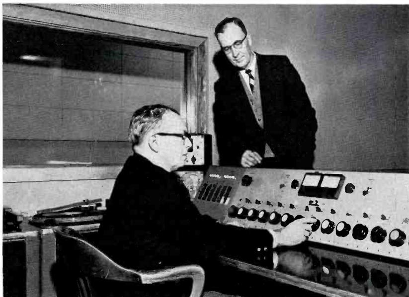
FIG. 16. WAVE-TV Chief Engineer Wilbur Hudson (standing) at audio console with Louis Lau, personnel supervisor. This dual console is one of a long list of equipments designed and constructed by the WAVE engineering department. Panel at left makes possible switching any one of six microphones to the input of each BA-21A preamp. The output of the mixers feed into BA-23A program amplifiers.
