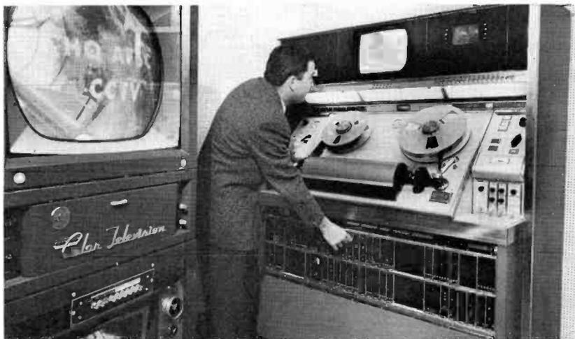
Andrews AFB video tape recording facilities include RCA TRT-1B and a transistorized TR-22 shown here.
