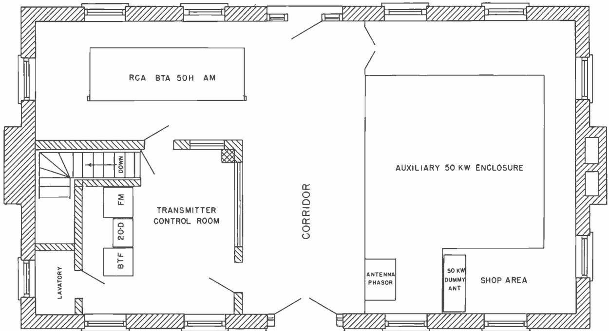
FIG. 5. WRVA-Radio transmitter building floor plan.
