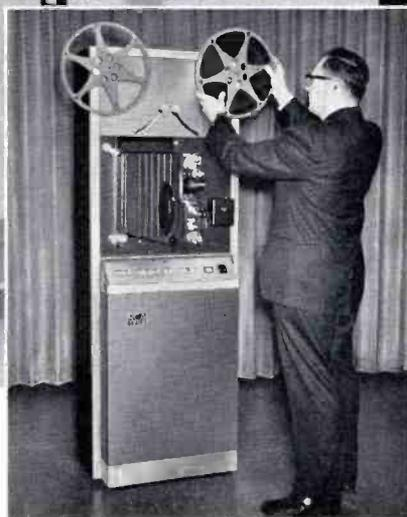
FIG. 12. Close-up of the TK-22 transistorized film camera and associated control and processing equipment. Control and processing units for two complete camera chains are mounted in the 5¼-inch rack frame shown.
