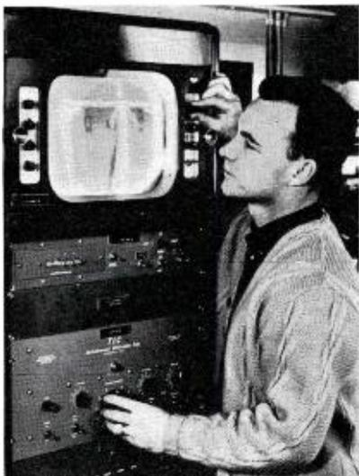
Wheelhouse control console brings in pickup from any of shipboard system's four television cameras.
