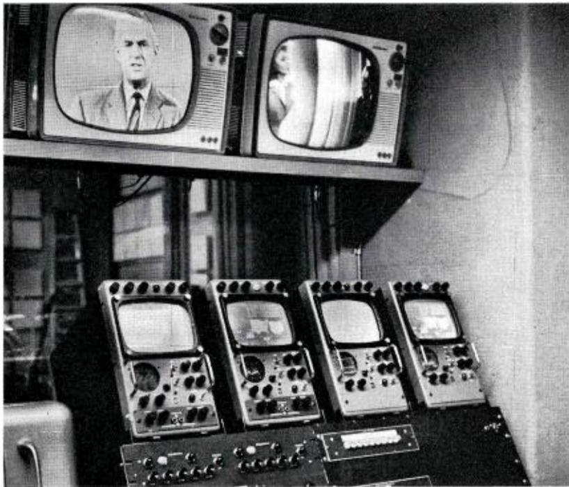
FIG. 7. Video control center, showing four TM-35 master monitors, controls for film system, and switcher-ladder.
