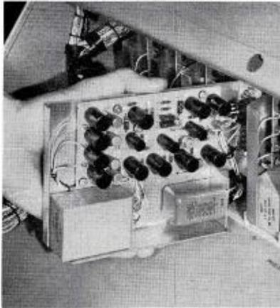
FIG. 19. Preamplifier unit.
