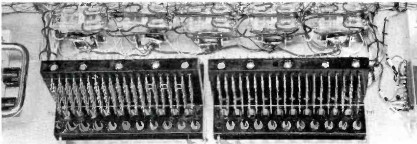
Other aids to flexibility are part of the construction of the console. Figure 17 shows the terminal block where all incoming sources are wired into the console. This type of jumper block construction simplifies wiring and facilitates inserting jacks into key circuits for patching in sound effects filters and dialog equalizers, etc. Also a control circuit delegation board, shown in Fig. 18, facilitates the delegation of muting and warning light relays for eight mixer positions.
