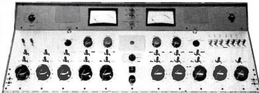
FIG. 3. Front view of consolette showing "human engineered" arrangement of controls.
