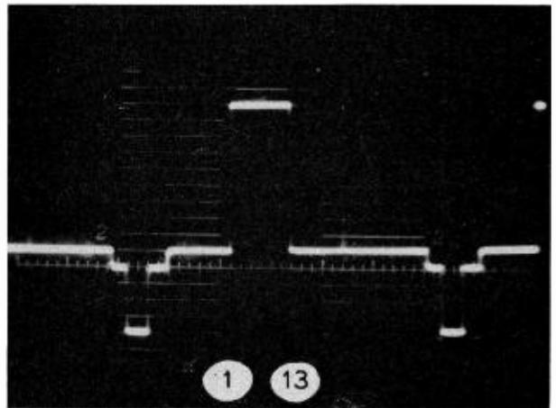
It consists of a standard white window and a pulse, both of which have sine-squared edges. The white window is primarily used for streaking tests and the pulse for ringing tests.
