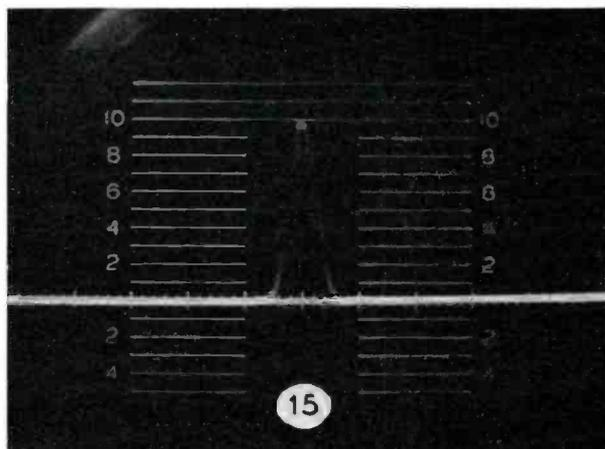
As viewed in your control rooms, the top of the window should be flat and not have excessively rounded corners. The sine-square pulse should not have excessive undershoots or overshoots.
