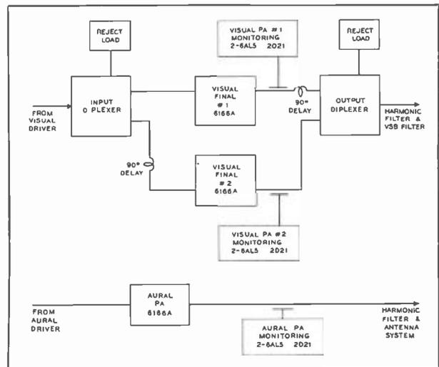
FIG. 12. Block diagram of the power-amplifier portion of the transmitter. Diplexed amplifiers increase transmitter reliability and better overall transmitter performance.
