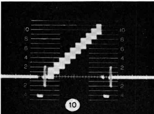
Taking waveform photos of the keyed-in test signals is no problem when using a CRO with a line selector, although it does take a little practice. However, photographing the keyed-in staircase signal after it has gone through a high pass filter is another matter. One method which works fairly well is to use the sync output from a TA-9 stab amp and drive the CRO externally.
