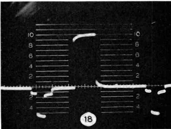
Both of these are excessive and indicate trouble. The slides we have just shown represent positive streaking (excessive lows). The next two slides are just the reverse of the last two slides and show negative streaking. (Slide Nos. 19 and 20.)
