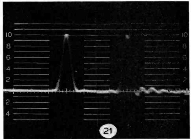
The easiest way to measure the pulse distortion is to adjust the CRO vertical gain and centering until the pulse is between zero and 100 on the IRE scale (Slide No. 22). Then adjust vertical centering until the most negative excursion is at zero and measure the top of the most positive excursion. The measurement will then be in per cent. (Slide No. 23). Photos taken for submission to Telco or your network representative should be centered as in Slide No. 22.
