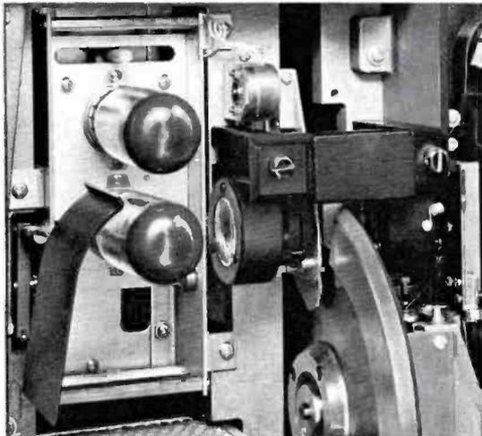
The projection lamps have a wafer stem keyed socket somewhat similar to an octal base tube socket. Easy access is provided for convenient and speedy replacement of lamps, even while the machine is running. The keyed base and socket assure proper alignment of the lamp upon replacement.
