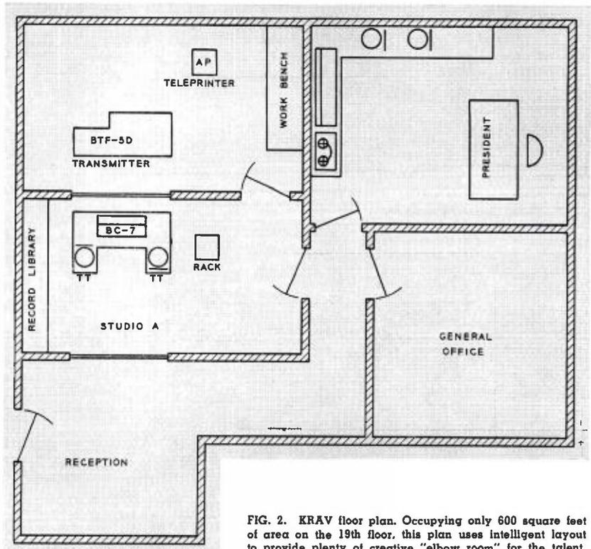
FIG. 2. KRAV floor plan. Occupying only 600 square feet of area on the 19th floor, this plan uses intelligent layout to provide plenty of creative "elbow room" for the talent.
