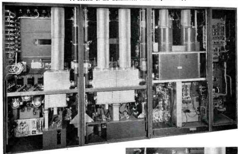
have to be replaced. This feature helps reduce operating costs and also reduces the possibility of lost air time. High-voltage transformer failures have resulted from mercury-vapor tube faults. This type of transformer failure is eliminated by the use of silicon diodes.
