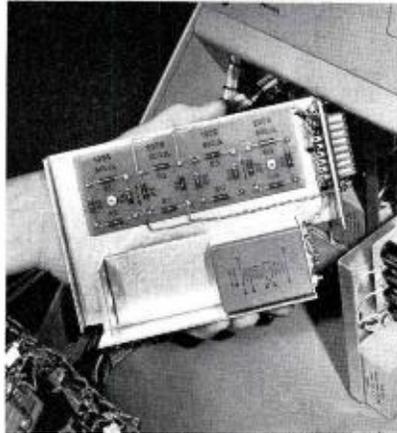
FIG. 20. High level isolation unit.
