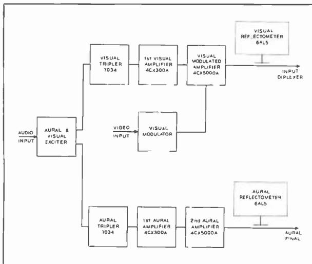
FIG. 11. Block diagram of the TT-25DH driver system. Capable of a full 5-kw visual output, the driver operates at approximately 60 per cent of capability in normal operation.
