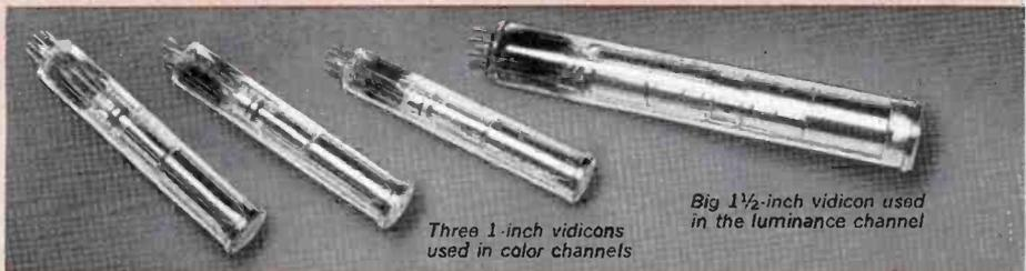
The 1½-inch vidicon in the luminance channel of RCA's color film camera provides a 50% larger image—50% larger than any used in other cameras. This gives improved signal-to-noise ratio, high resolution capability. Result: Unusually sharp reproduction of color films and slides.
