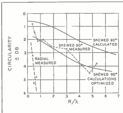
FIG. 14. Curves of circularity vs  $R/\lambda$ .
