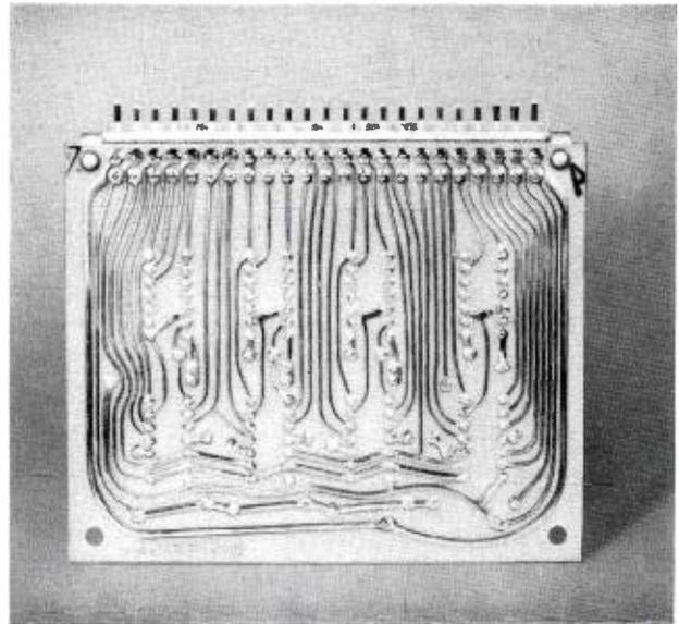
FIG. 7. Wiring interconnections on rear of circuit board.
