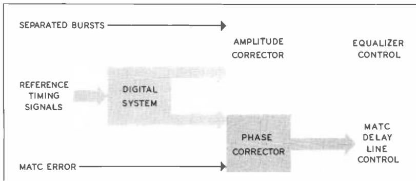
FIG. 8. Block diagram showing principal functions of CAVEC.
