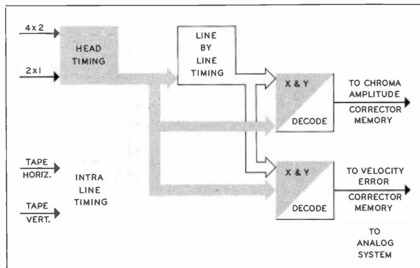
FIG. 12. Block diagram of digital switching system.
