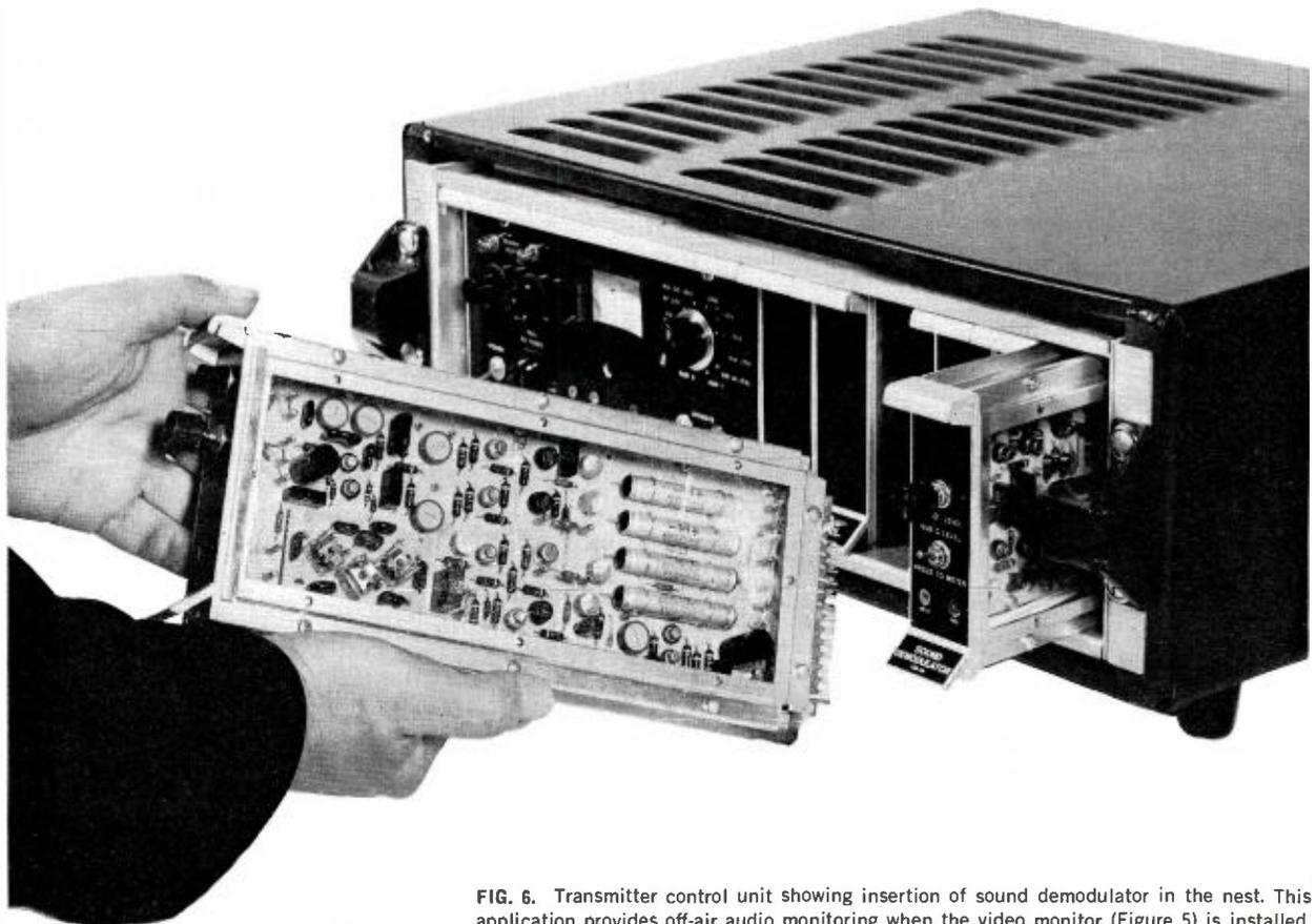
FIG. 6. Transmitter control unit showing insertion of sound demodulator in the nest. This application provides off-air audio monitoring when the video monitor (Figure 5) is installed.
