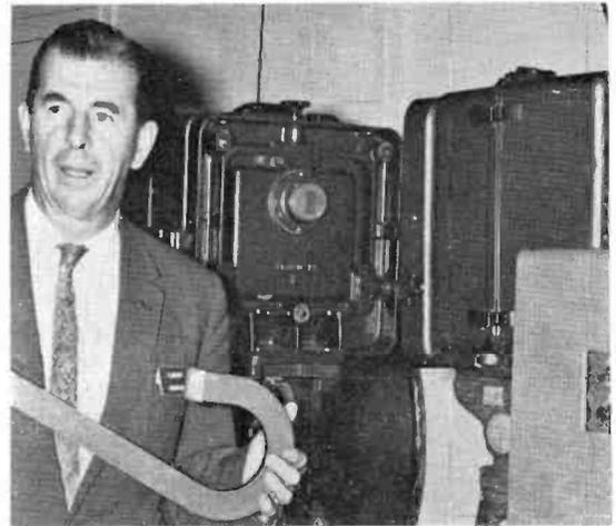
FIG. 13. Placement of "see yourself" PK-301 remotely controlled vidicon camera used for training instructors in improved teaching.
