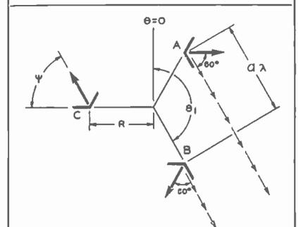
FIG. 5. Three skewed panels.  $a=n+\Delta$ ,  $\Delta=0, 1/3$  or  $-1/3$ ;  $n$ =integer,  $\psi$ =skew angle.
