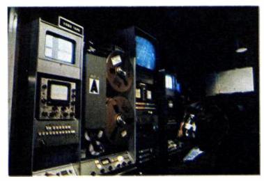
The Video Tape center in the MTS van is located behind the Audio Control and is equipped with two TR-61 VTR's plus tape editing facilities.
