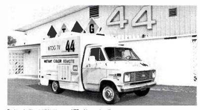
Equipped with portable cameras, VTR, video and audio switching, this compact mobile unit extends TV-44's production capability for covering field assignments.
