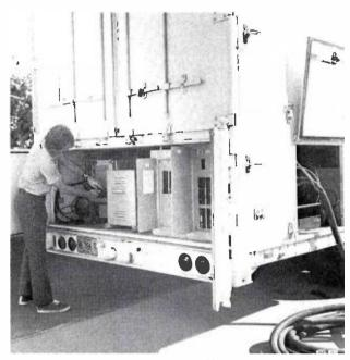
Mounted at the rear of the trailer, behind the video compartment is the power control equipment, including the power input panel; transformers and voltage regulators.
