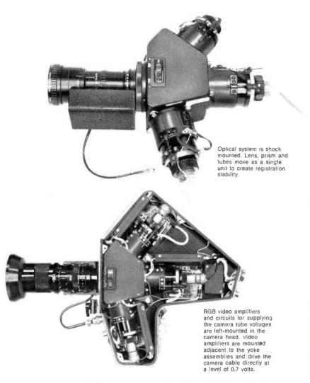
system. In the new TKP-45 camera, the deflection power has been reduced to 12 percent by utilizing a novel horizontal deflection drive circuit.
