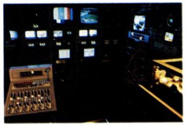
Video Control equipment is housed in the rear compartment. This master engineering center contains all electronic support facilities: joy stick controls for all six color cameras plus video patching, control and monitoring equipment.
