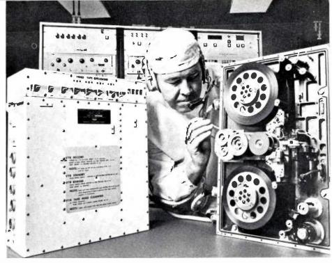
SPACE RECORDER—technician Everett Ware makes an optical alignment check on the color video tape recorder system that flew on the Apollo-Soyus space-docking mission.
