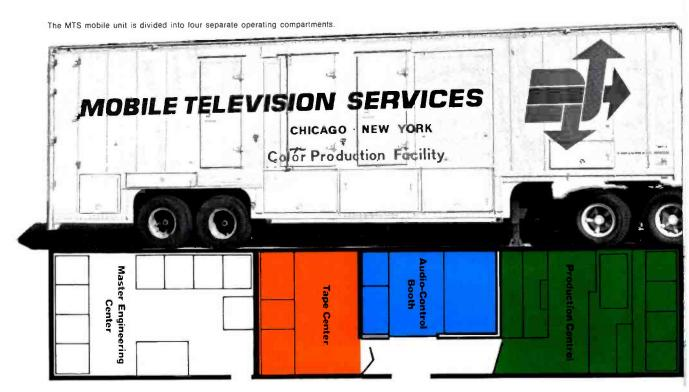
Mobile Television Services' 40-foot mobile unit is a fully equipped video production center.
