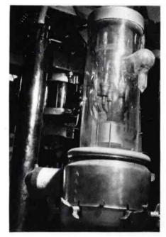
A closeup of a 100 KW tube used in the 50 KW transmitter.
