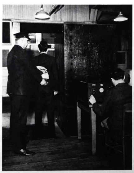
An RCA gun detector or automatic "frisker" which reveals the presence of ferrous metals.
