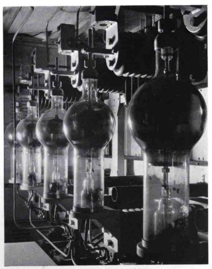
Lineup of rectifier tubes in the 50-C.
