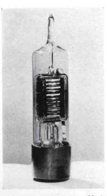
Figure 6. Tube used in first Trans-Atlantic broadcast—1915.
