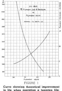
in life when operating a tungsten filament at reduced temperatures.
