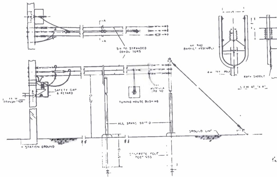
Diagram of the six wire transmission line.
