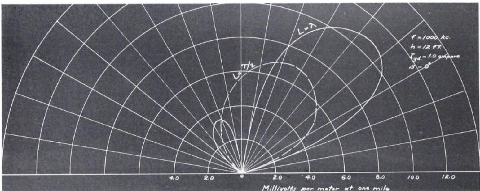
foot, for a number of transmission line heights, with  $I_{gd}$  equal to one ampere. We see that as the transmission line is placed closer to the earth, the current density increases directly below the line, but drops off quicker in a lateral direction.
