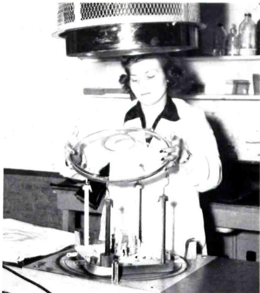
9. The spherical mirror which forms the main "lens" in the reflective optical system is shown here before aluminizing. It is a salad-bowl shaped piece of glass 14 inches in diameter with a 4-inch hole in the center. The inner surface is ground to a true spherical shape on a standard optical grinding machine.
