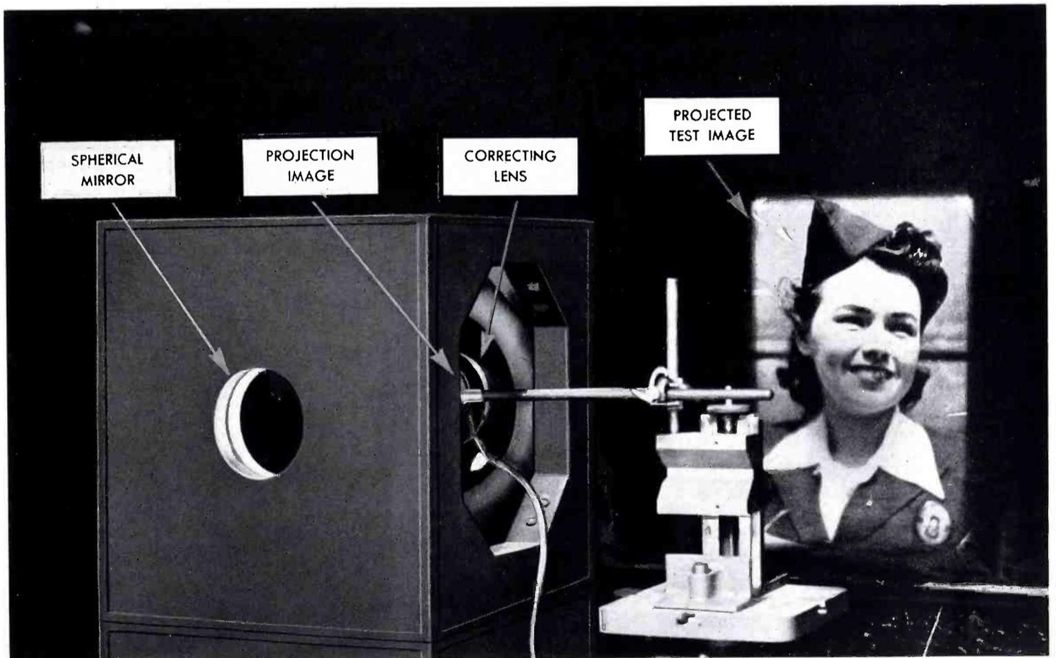
2. In this view, one of the molded correcting lenses has been placed in the correct relative position on the front of the box (the far side). The picture, as will be seen, is now very much sharper and brighter. (In these two views certain details of the test box have been retouched, but in neither case has the projected picture been retouched at all.)
