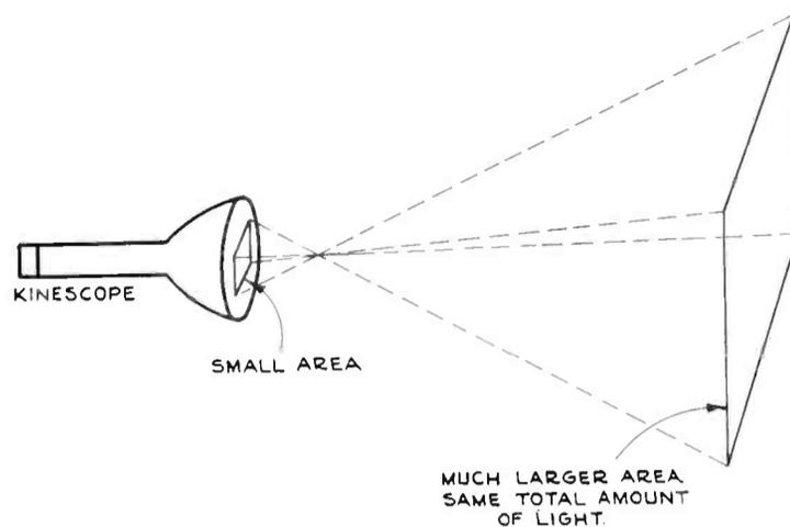
trons in the beam (i.e., the beam current). Both entail difficulties. Increasing the voltage requires greater spacing and better insulation within the tube. Increasing the current requires higher emission cathodes.
