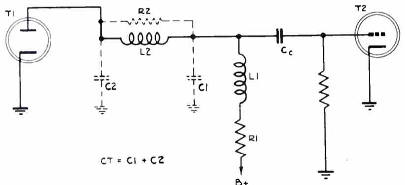
FIG. 11. Combination peaking stage.
