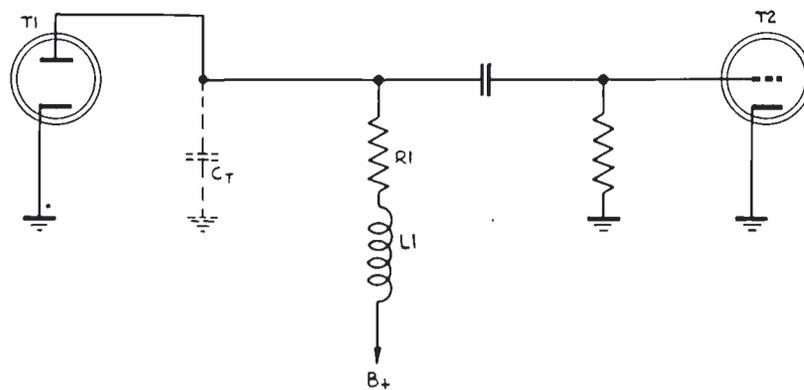
FIG. 7 Shunt peaked stage.
