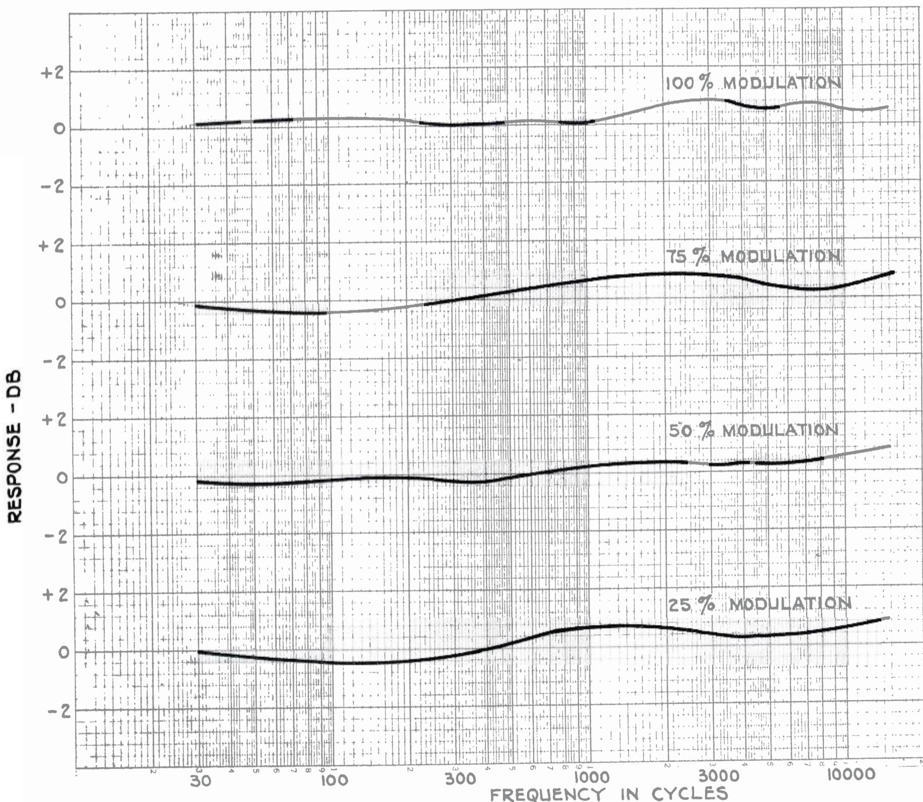
FIG. 3. Frequency response curves of an FM system for several percentages of modulation. A set of curves similar to these must be filed in answer to Par. 6(a) of Form No. 320.
