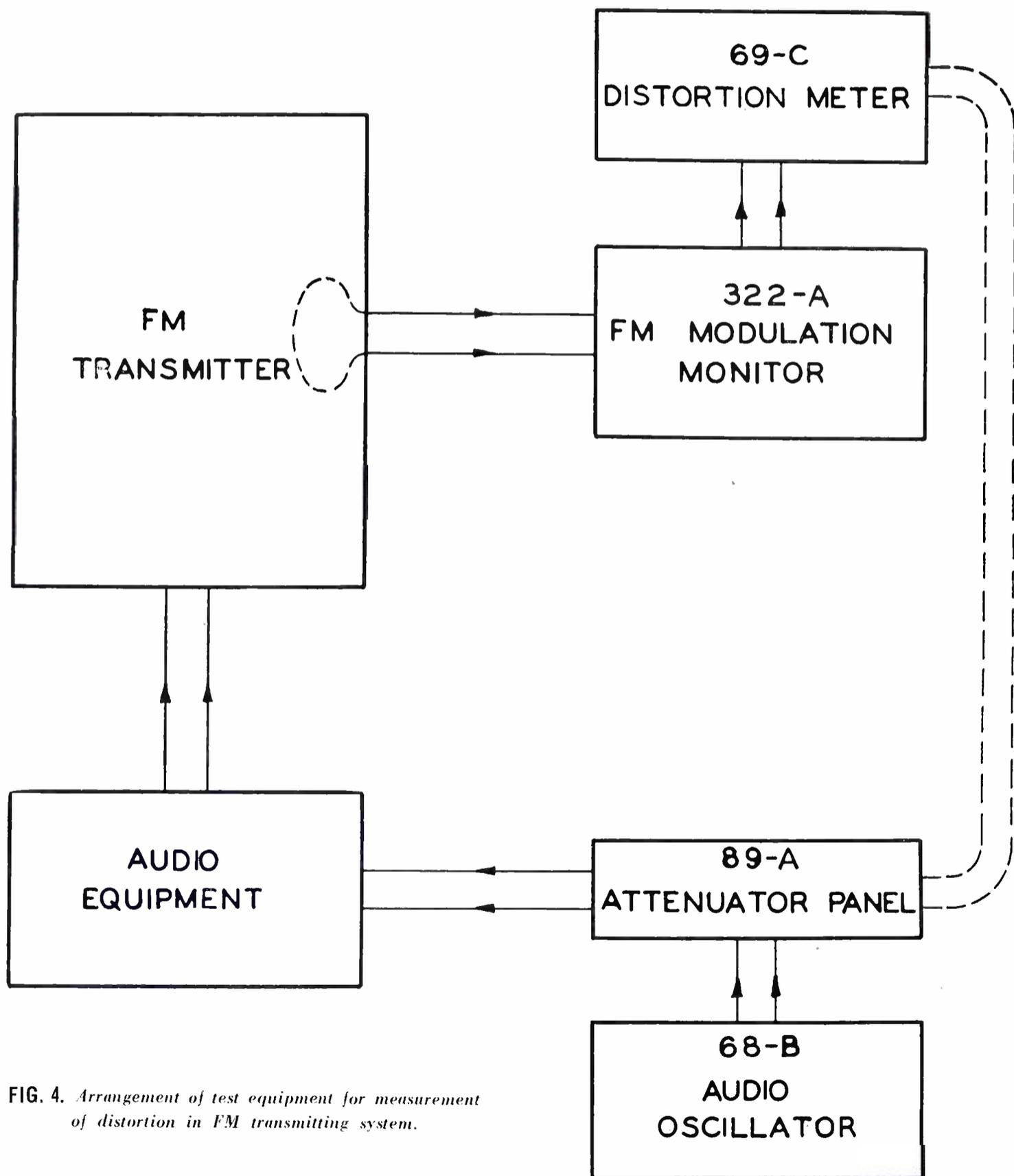
FIG. 4. Arrangement of test equipment for measurement of distortion in FM transmitting system.
