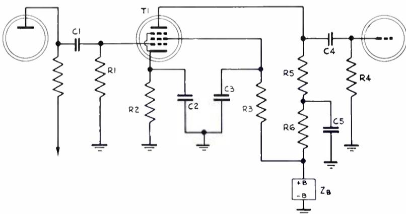
FIG. 5. Amplifier stage with low frequency correction network ( $R_6-C_5$ ).
