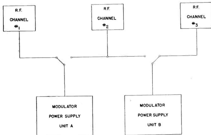
FIG. 5. Simplified block diagram of transmitter switching circuit in use at OWI-CBS International transmitting plant located at Wayne, N. J. It illustrates how r-f channel #1 can be energized from modulator "A", and r-f channel #3 from modulator "B"; whereas r-f channel #2 can be switched to either modulator "A" or modulator "B".
