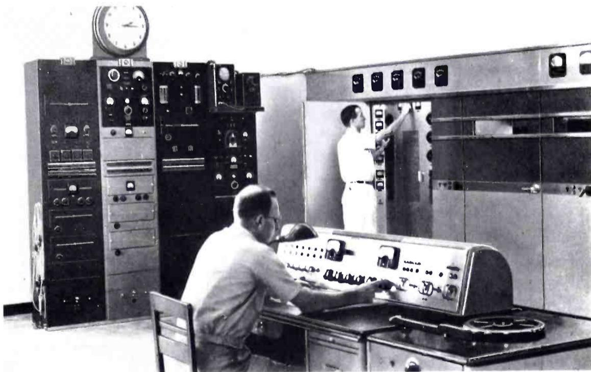
FIG. 3. RCA operating console, r-f section of RCA 50 KW transmitters and RCA test equipment racks.
