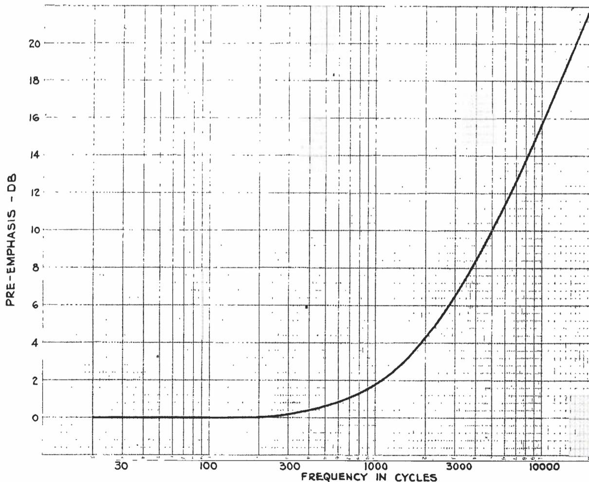
FIG. 1. RMA Standard Pre-emphasis Curve which is incorporated in FM Transmitting Systems
