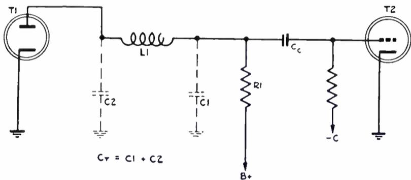
FIG. 9. Series peaking stage.
