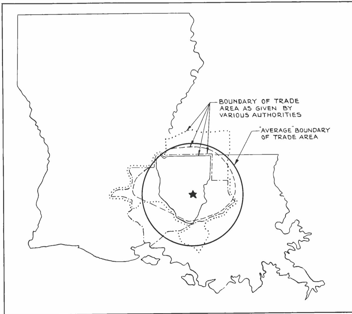
FIG. 7. Outline map made by tracing the important boundaries of the map in Figure 6 and drawing in a curve corresponding approximately to the average of the four trade area boundaries. This "average boundary" is the area which the station should be designed to serve.
