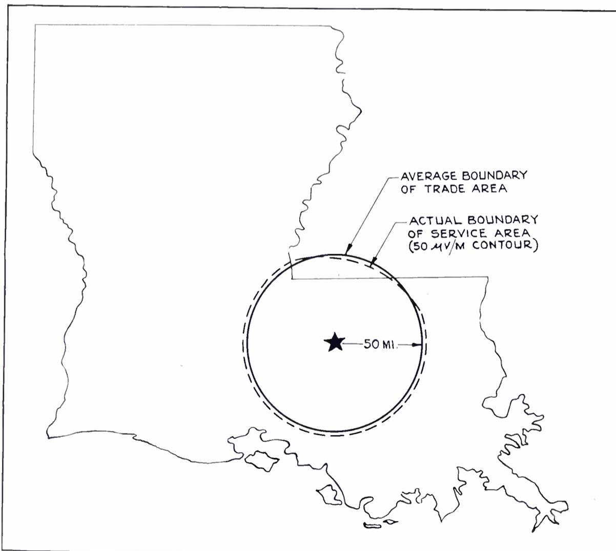
**FIG. 1.** The power and location of an FM station should be such that the 50 microvolt contour coincides as nearly as possible with the "service area."
