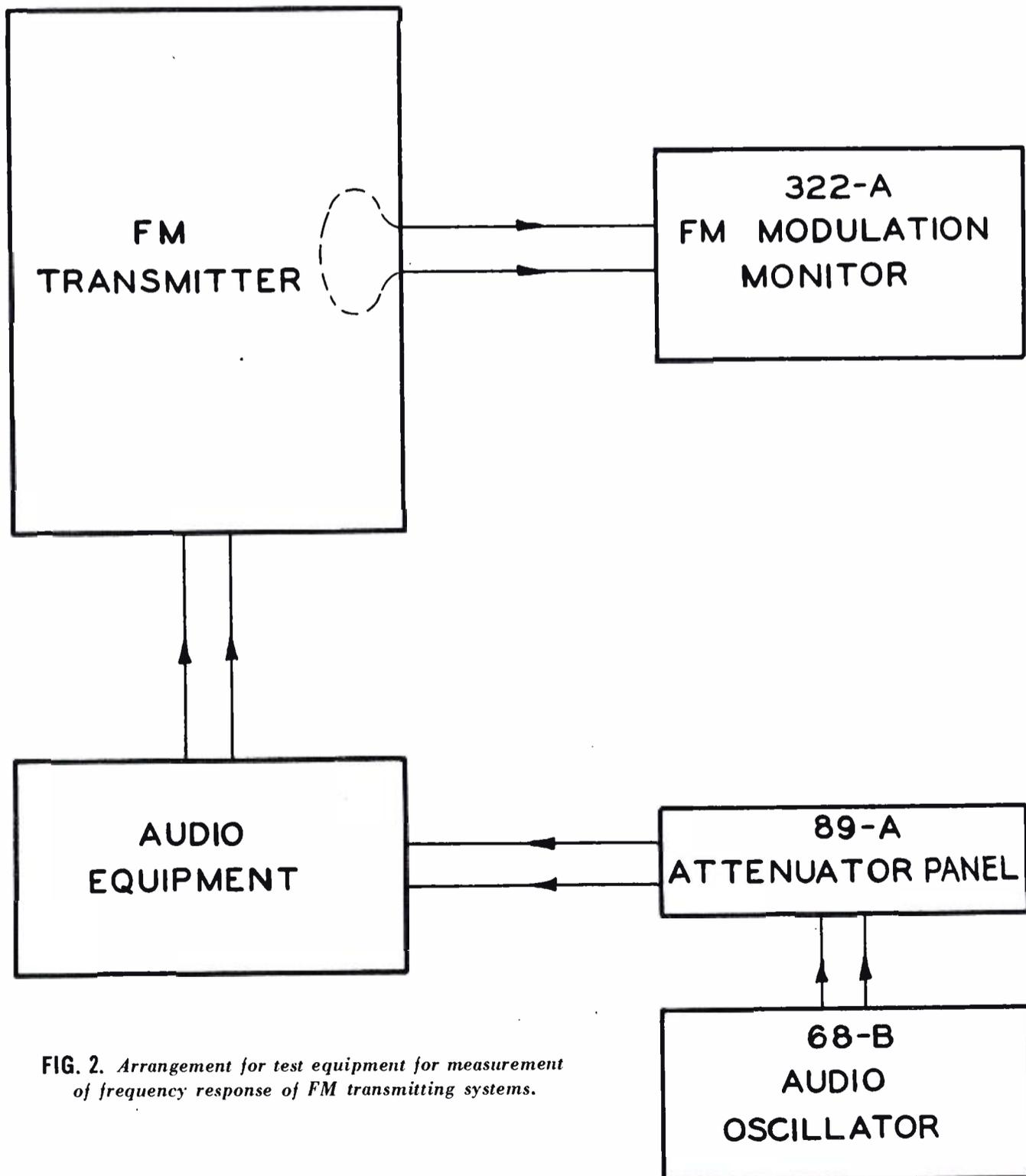
FIG. 2. Arrangement for test equipment for measurement of frequency response of FM transmitting systems.
