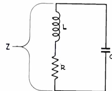
FIG. 6. Basic shunt peaked network.
