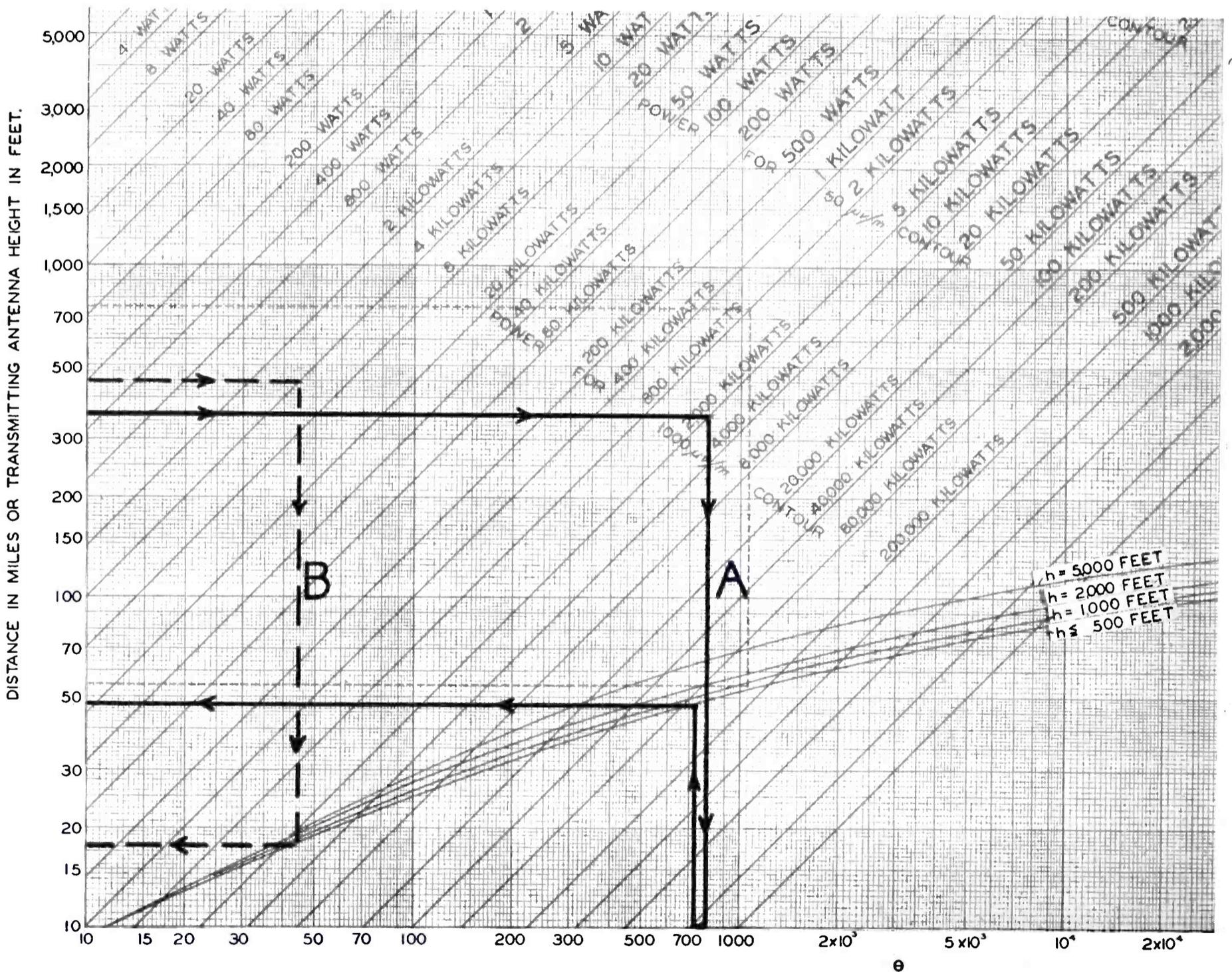
FIG. 4. Part of the FCC chart "Signal Range for High Frequency Broadcast Stations." Using this chart the distance to the 50 microvolt line for a given elevation and power can be determined as shown by the solid line with arrows (see text). Distance to 1000 microvolt line is determined as shown by the dotted line with arrows.
