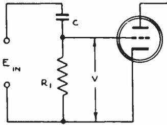
FIG. 3. Grid coupling network.
