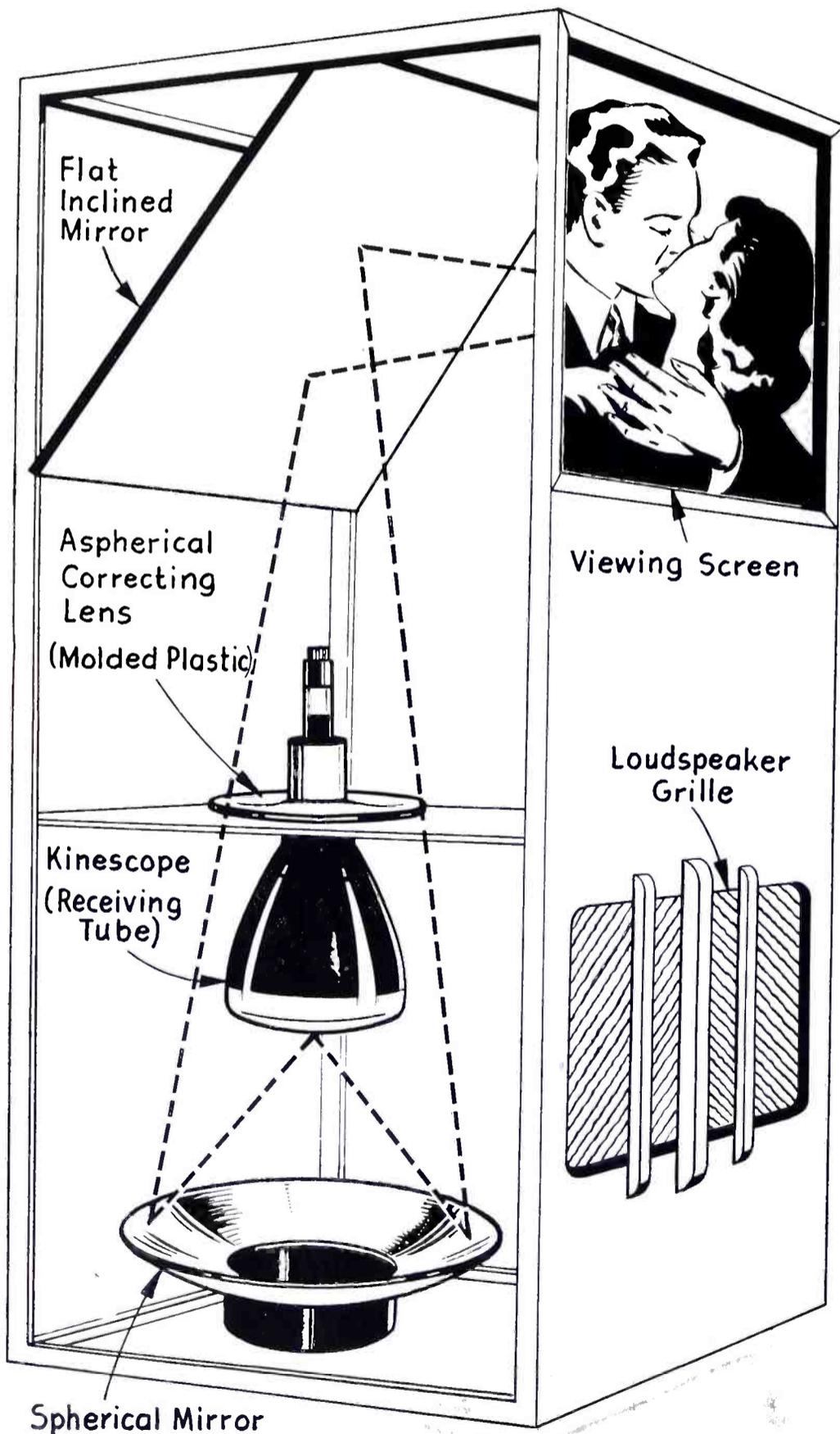
The projection receiver illustrated on the preceding pages is a self-contained unit containing all elements of the system from antenna lead-in to viewing screen. In this respect it differs radically from most of the proposed projection receivers in which the picture is usually intended to be projected onto a wall or screen some distance away.
