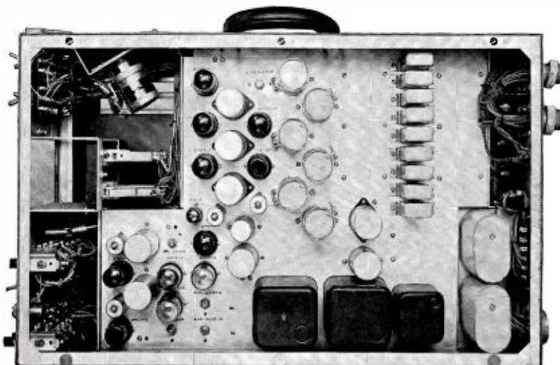
FIG. 12. The switching unit with left side cover removed. Intercom switching circuits are mounted in upper part of unit; video switching circuits in lower part.
