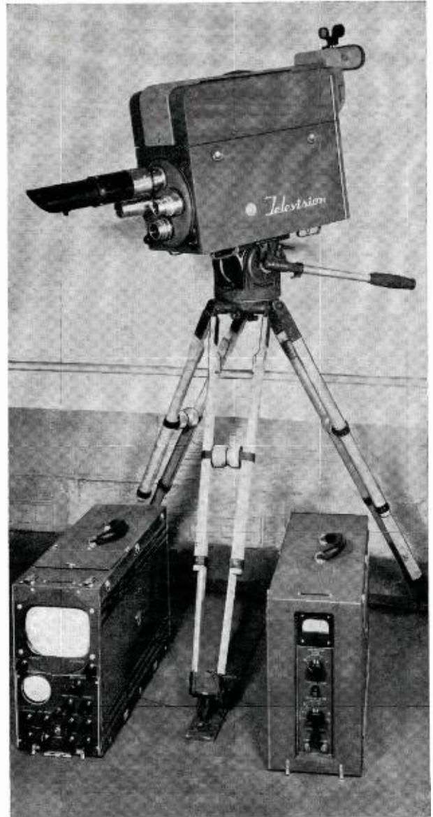
**FIG. 5.** (Above) Illustrated here is a complete Type TK-30A Camera Equipment. This grouping, often referred to as a "camera chain," is a complete operating unit in itself (except that it must receive synch signal from an external source). When a three-camera setup is desired the equipment units shown above must be added to the equipment grouping shown in Figure 1. For a four-camera setup, two complete groupings, as shown above, must be added.
