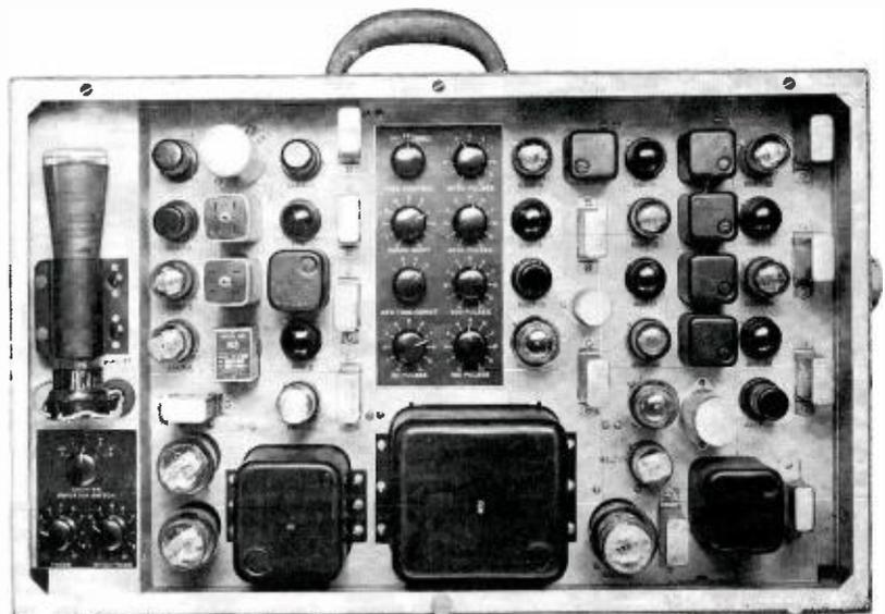
FIG. 10. The pulse shaper unit (of the Synchronizing Generator) with left side cover removed. The small cathode-ray tube at left is used in making initial circuit adjustments.
