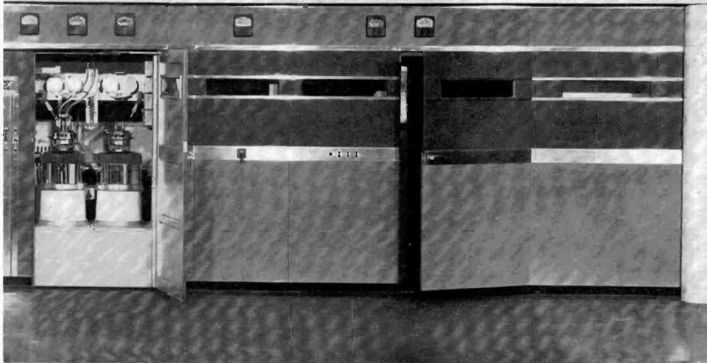
**FIG. 1.** (Above) *The streamlined, unified front of the 50-F contains wide, full-length doors which provide direct, non-hampered access to the low-power r-f modulator and power amplifier compartments. The door at the right is the entrance to the non-interlocked area which contains the control and distribution unit and the main switchboard unit (see diagram on following page).*
