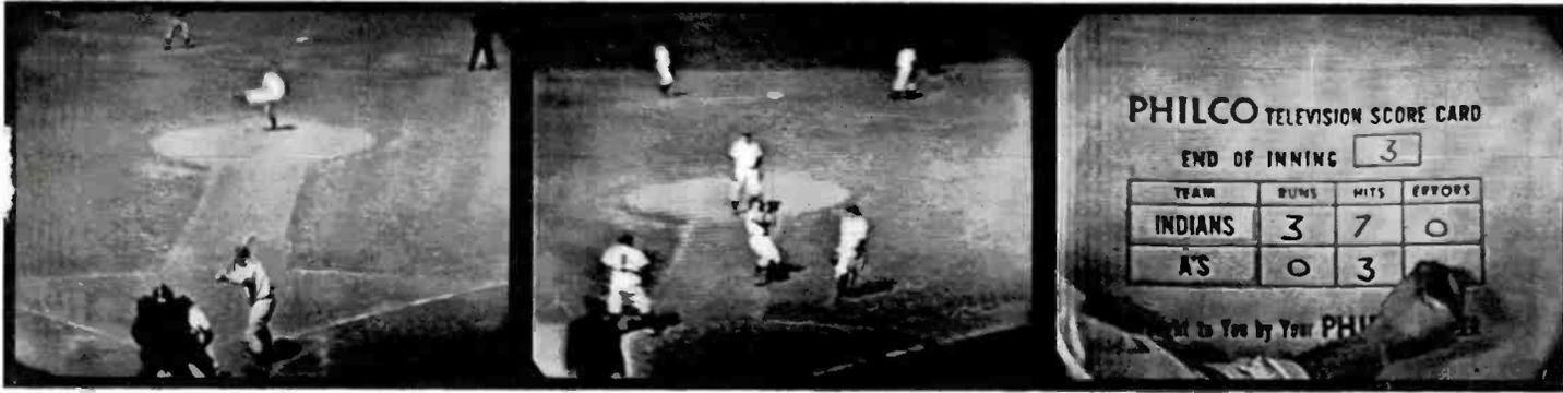
135MM lens was being used when the above three photos were made. This lens, which has a 13 degree angle, is the workhorse of baseball television. It has a 10 to 15 foot field width at the plate (depending on distance away), with depth sufficient to take in both homeplate and 2nd base. It provides reasonable size pic-
