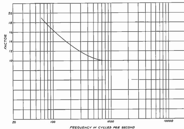
FIG. 5. Reverberation time-frequency ratio.
