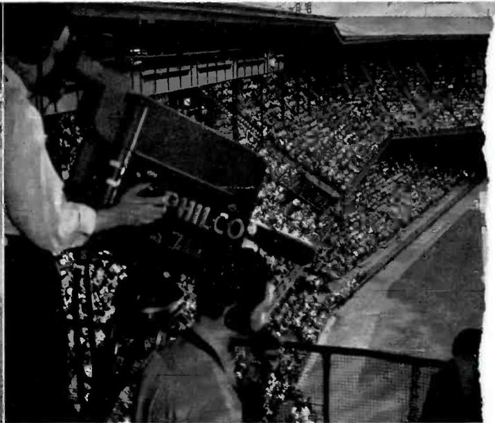
WPTZ, Philadelphia (A's and Phillies) uses two RCA TK-30A Cameras. Both are behind homeplate just a few feet to the right of the pitcher-batter line. No. 1 camera is in a cage hung from the upper deck (left, above). No. 2 camera in the press box some forty feet higher (right, above).
