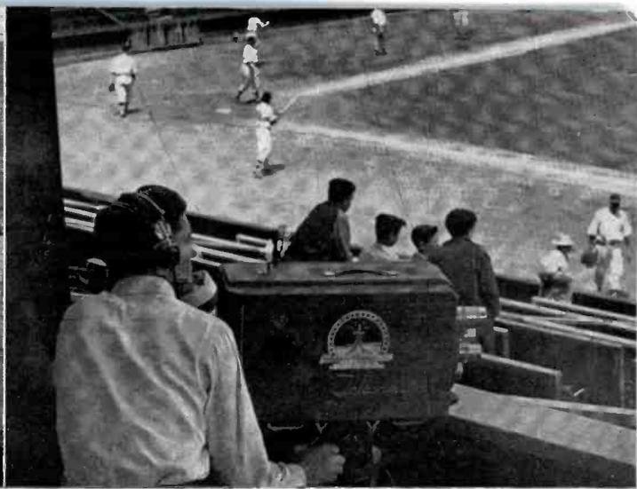
KTLA, Los Angeles (Coast League) uses two RCA TK-30A Cameras. The No. 1 camera is located directly behind homeplate in the lower stands (lower left corner of the lefthand view, above). The No. 2 camera is just off 1st base, also in the lower stands, but with sufficient height to follow action in the field. Excellent closeups on all bases are available from this camera position. No. 1 camera picks up the pitched ball as it comes over the plate, with No. 2 following the ball into the infield
