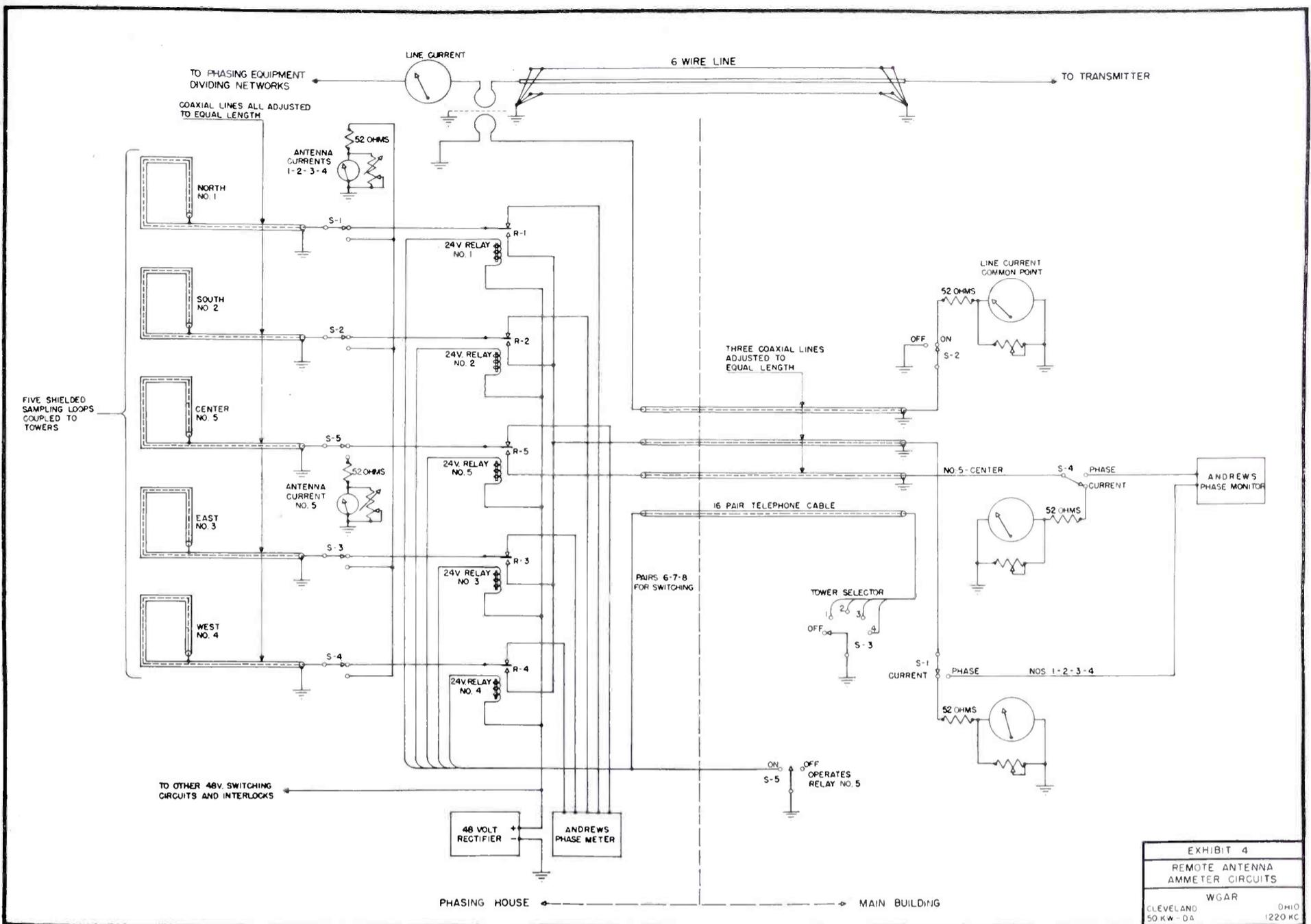
FIG. 13. Sampling loops coupled to each of the five towers feed coax lines which terminate in the center tuning house. Three coax lines from the center house to the transmitter room, together with a suitable switching arrangement, provide a means whereby the current and phase in any tower may be monitored at the transmitter. The diagram above shows the circuits involved.
