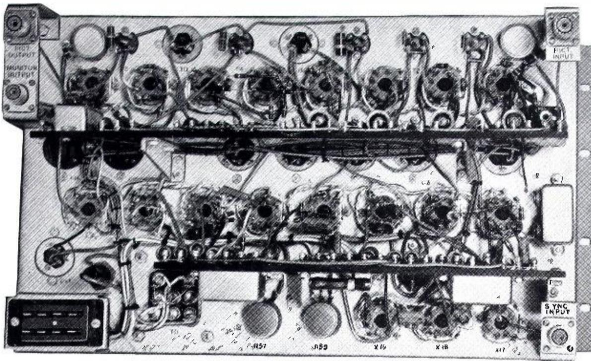
FIG. 7. Rear view of the TA-5B Stabilizing Amplifier. Video connections are made through the coaxial receptacles at the corners of the chassis.
