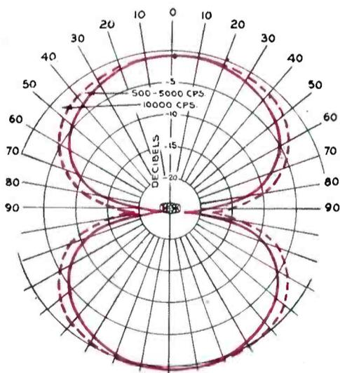
**Directional characteristics of a typical KB-2C microphone.**
