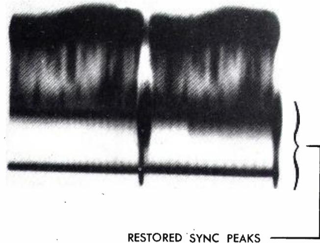
**FIG. 12.** An oscillogram of the signal obtained from the TA-5B after feeding the composite signals of Figures 9, 10, and 11 into the Stabilizing Amplifier. Note the increase in both sync-picture ratio and signal-to-noise ratio in the sync. Also the hum has been completely eliminated. A 30-cycle sweep frequency was used here.
