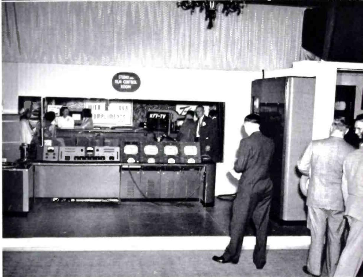
FIG. 4 (right, lower). Operator on duty at the video console in the control room had three program sources to select from: the "studio," the film projection room, and a monitor receiver on the local television station.
