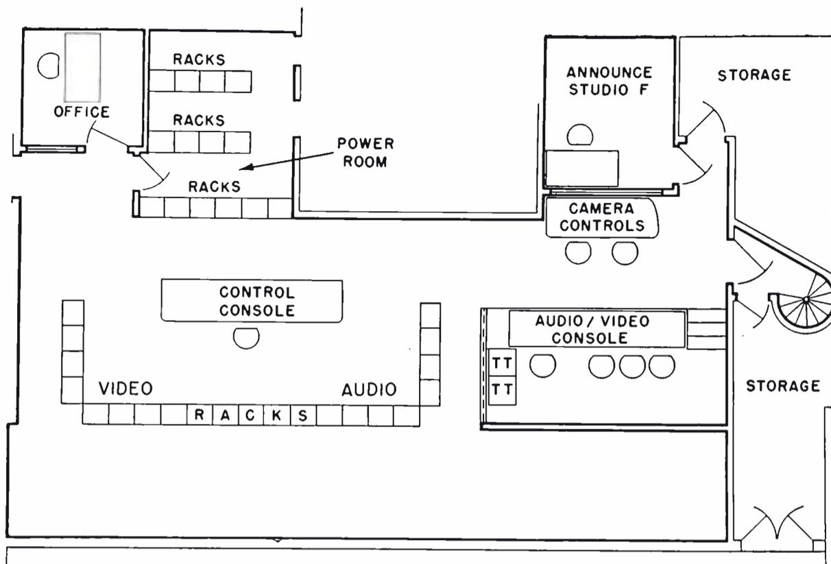
FIG. 10. Arrangement of equipment units in the master control room. The adjacent film control setup and Announce Studio F. This area is located on the second floor directly above the control room of Studio A and the Telecine Studio. This arrangement keeps the length of video cables to a minimum. Note circular stairway providing quick access to floor below.
