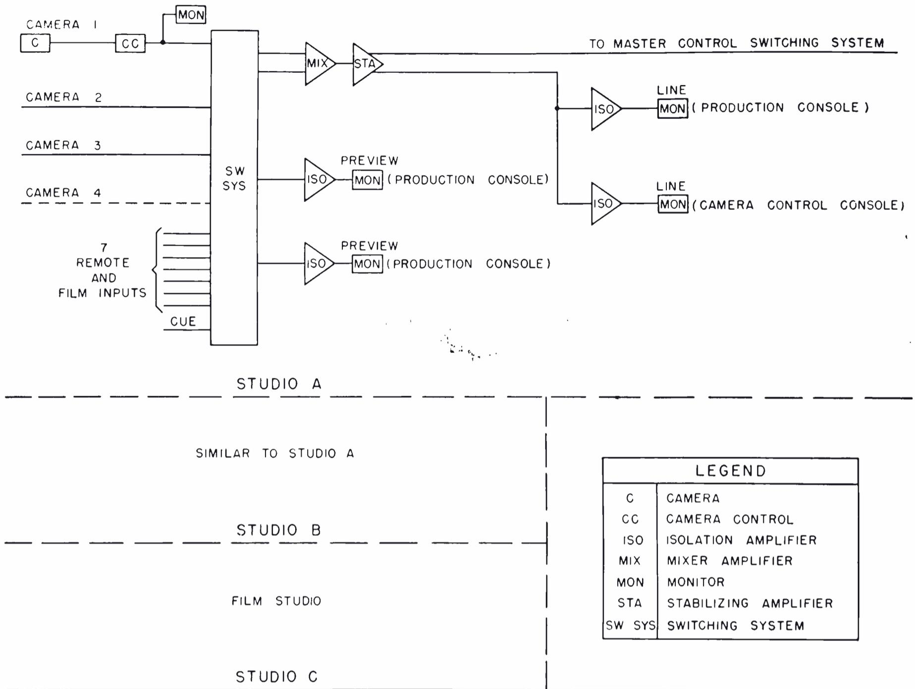
FIG. 8. Simplified block diagram of the video facilities for Studio A. Video units for Studios B and C are similar.
