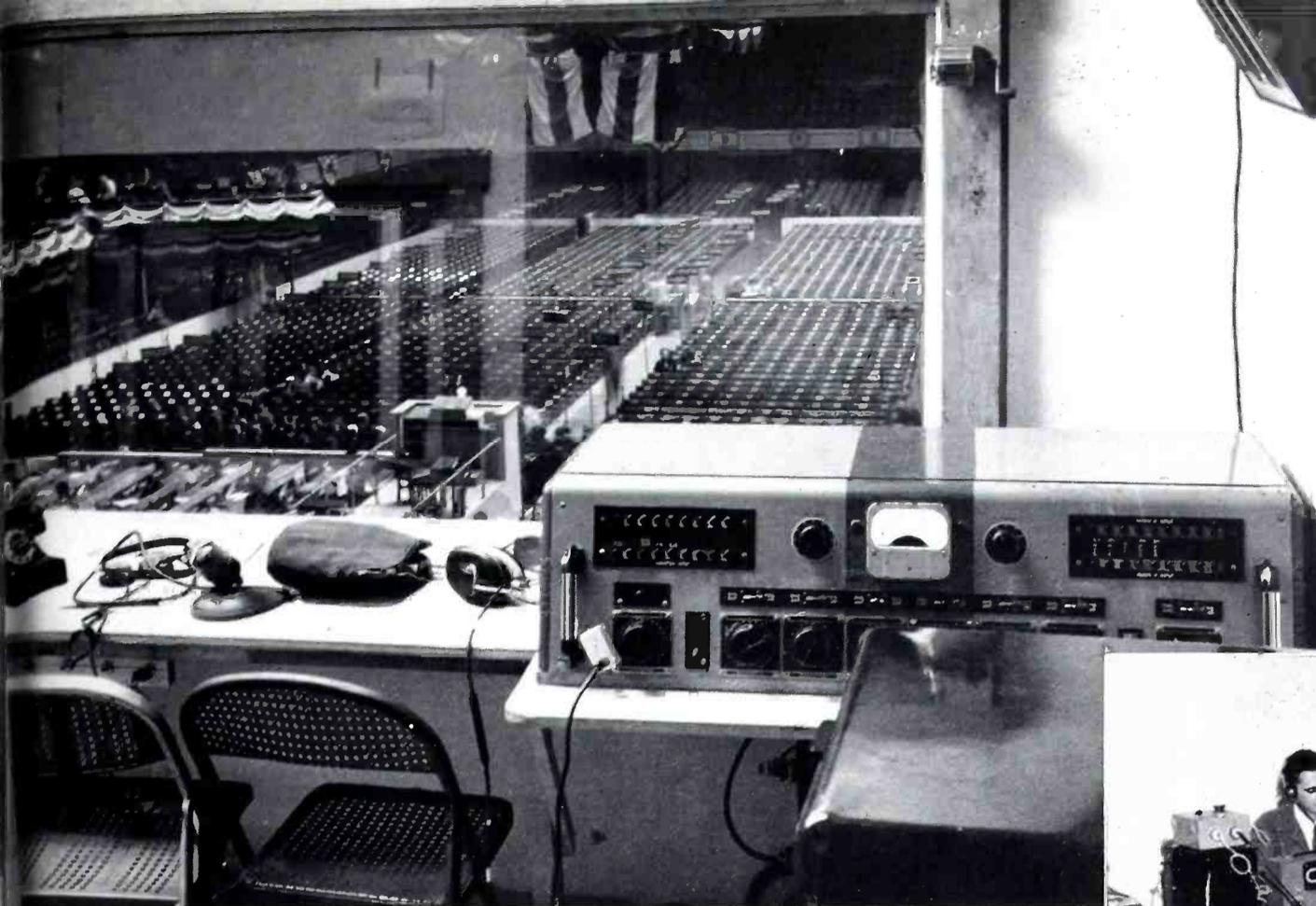
CBS's CONVENTION HALL AM FM CONTROL BOOTH is pictured at the left. Audio mixing and control is provided by the RCA 76-B2 Console. Audio inputs are from floor pickup, from news room, from microphones on table in front of window and from remote points.
