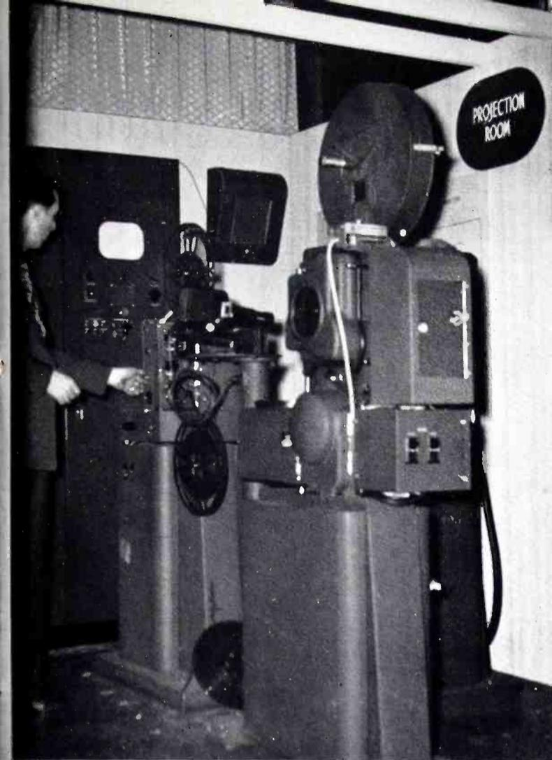
FIG. 6. The film projection room of the NAB display. In the foreground are 16mm and 35mm projectors. A multiplexer unit, between the projectors, allows the picture from either to be projected into the film camera (behind the 35mm projector in this view).
