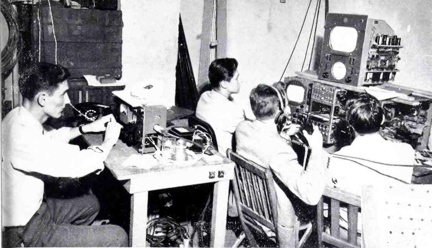
NBC's HOTEL CONTROL ROOM is shown at the left. Video units (at right of picture) include two RCA TK-30A Camera Control Units, with a TS-30A Switcher between, and a TM-5A Master Monitor on top. Audio position, at left, features on OP7.
