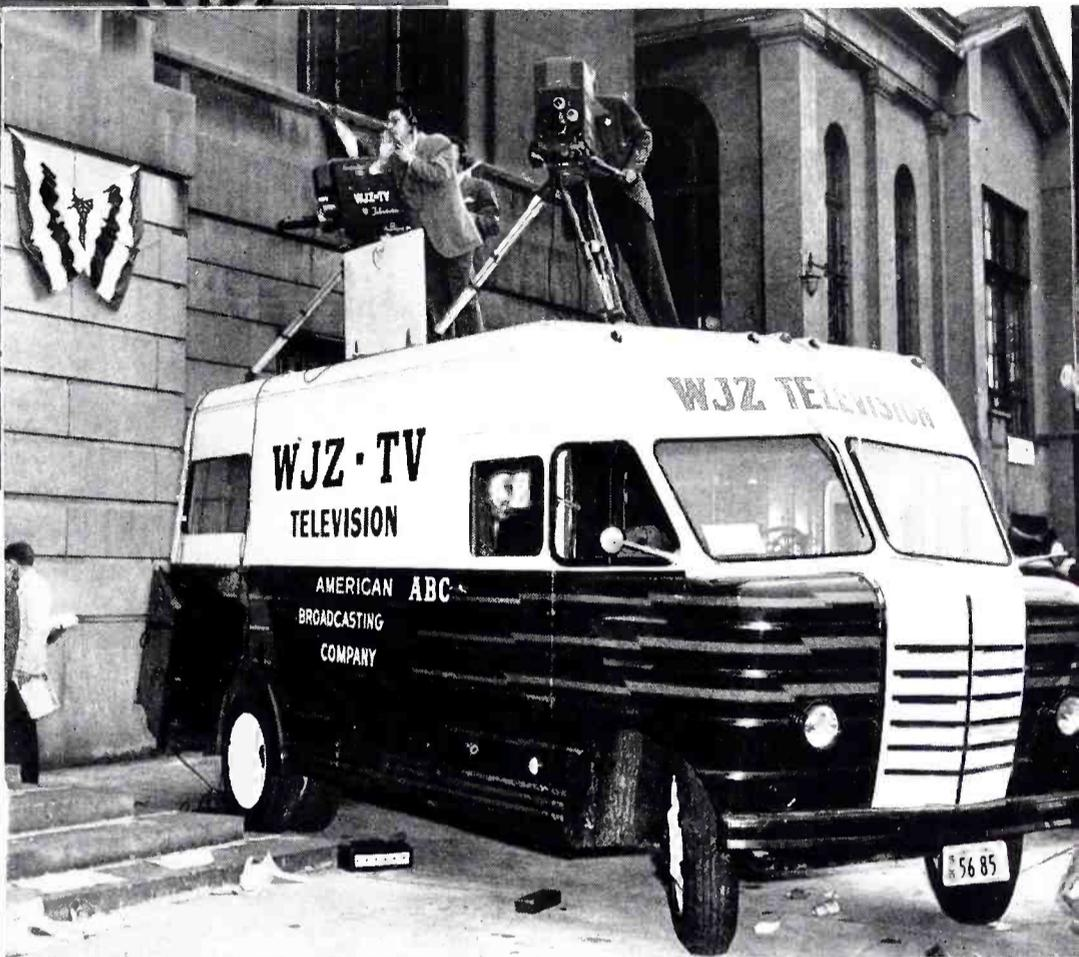
NO. 5 CAMERA POSITION (at right) was on a mobile TV unit just to the right of the main entrance. This was used just before meetings to show delegates arriving. Truck is an RCA Type TJ-50A Mobile Unit; Cameras are RCA TK-30A's. Equipment was furnished by ABC and operated, for the pool, by ABC technicians.
