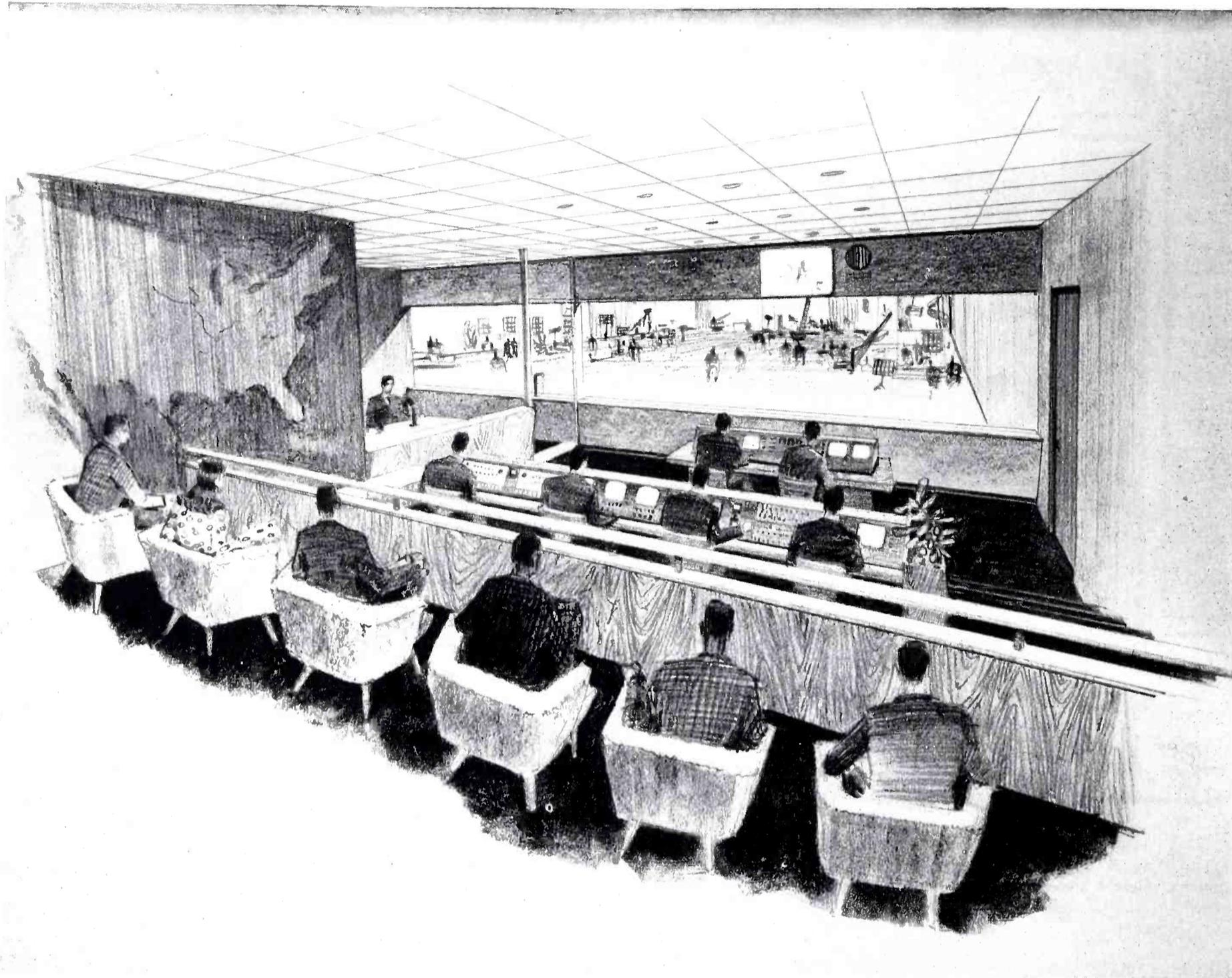
FIG. 6. Artist's sketch of one of the large-studio control rooms. Note the unobstructed view into the main studio and the announce studio (left center). An unusual feature of these control rooms is the provision of seating space for clients on an elevated platform at the rear.
