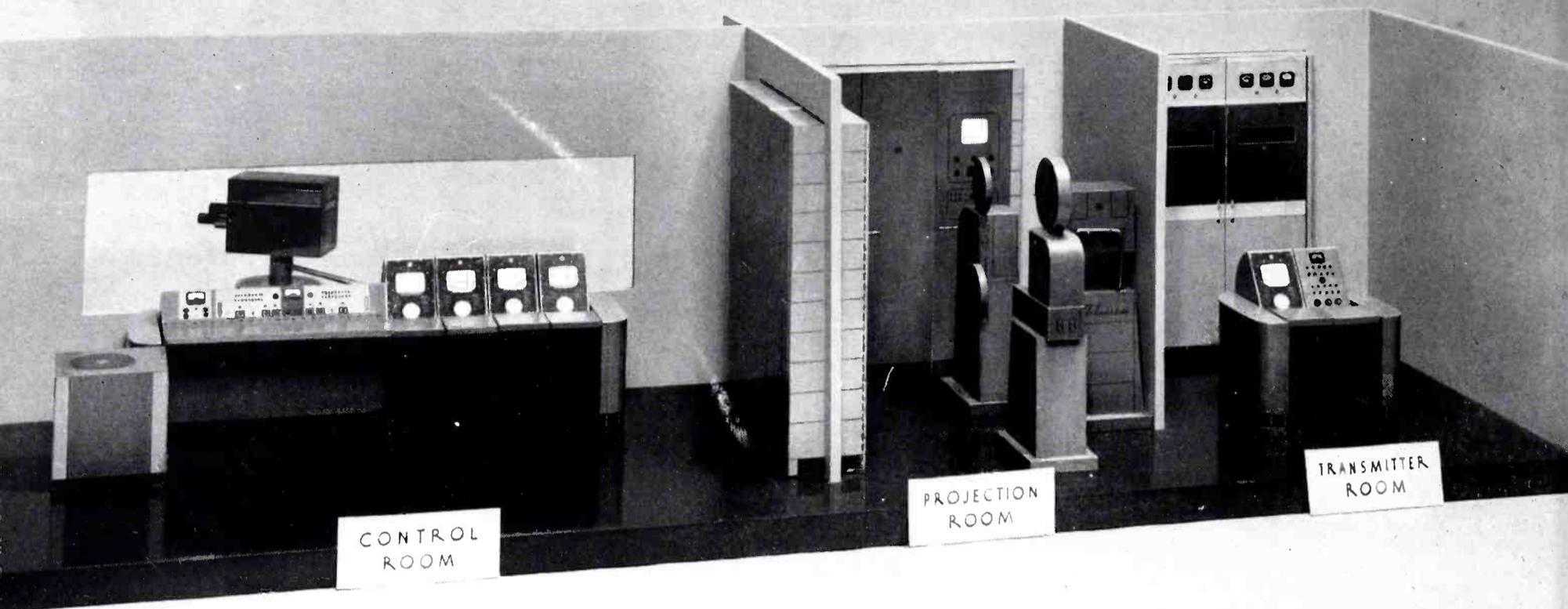
FIG. 1. This is a scale model of the "complete television station" displayed at the NAB Convention. Room at the left is a typical studio control room, room in the center is the film projection room and the room at the right, the transmitter room.
