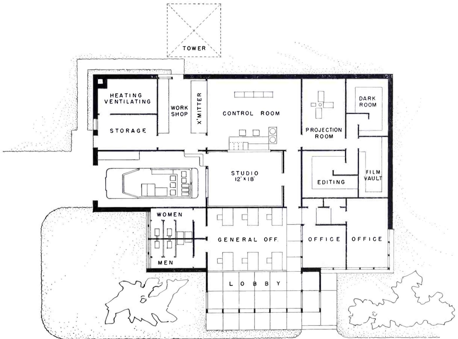
FIG. 14 (above). Floor plan of the small station building. No permanent video equipment is provided—operation of the studio for live talent shows requires use of the truck equipment.
