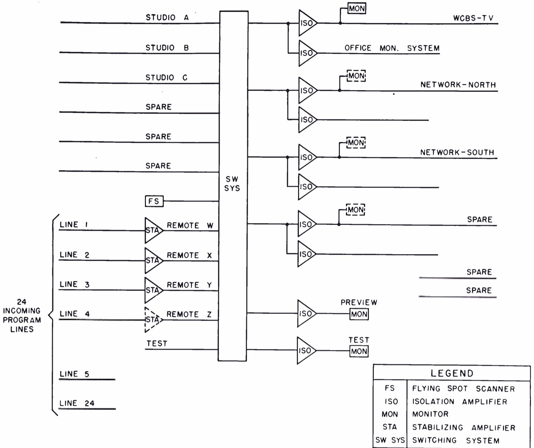
FIG. 11. Simplified block diagram of the video master switching arrangement. Provision of additional units is indicated by broken lines.
