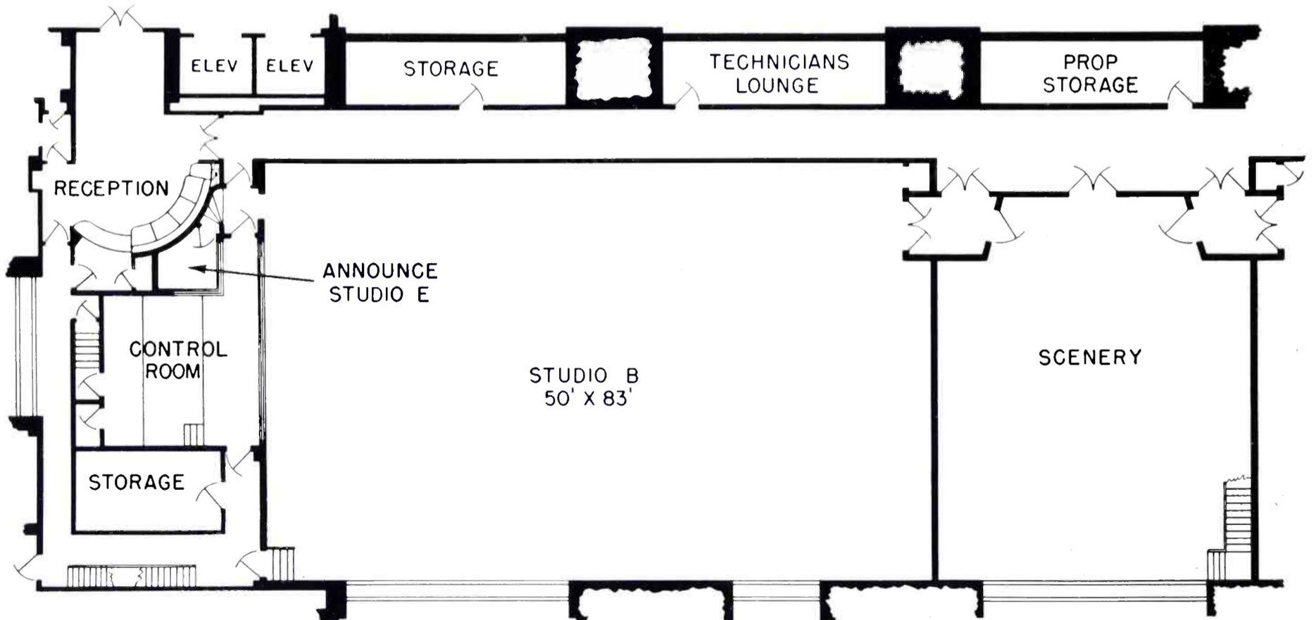
FIG. 4. Floor plan of Studio B showing position of Control Room B and Announce Studio E. Note the conveniently located areas for prop storage, scenery, etc. Arrangement of equipment in the control room and the announce studio is shown in detail in Fig. 5 (opposite page).
