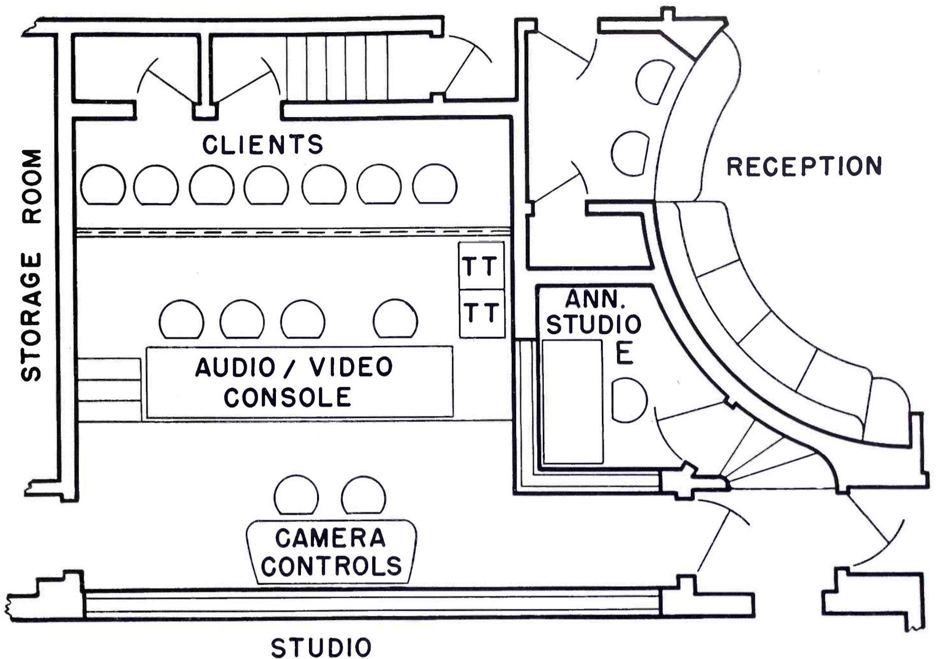
FIG. 5. Arrangement of the control room associated with Studio B (that for Studio A is similar). Video operators sit at camera controls directly in front of studio window. Just behind, and slightly above, is a console at which sit the program director, the assistant program director, a video "switcher" and the audio technician. In a third row is a space for clients or other special guests.
