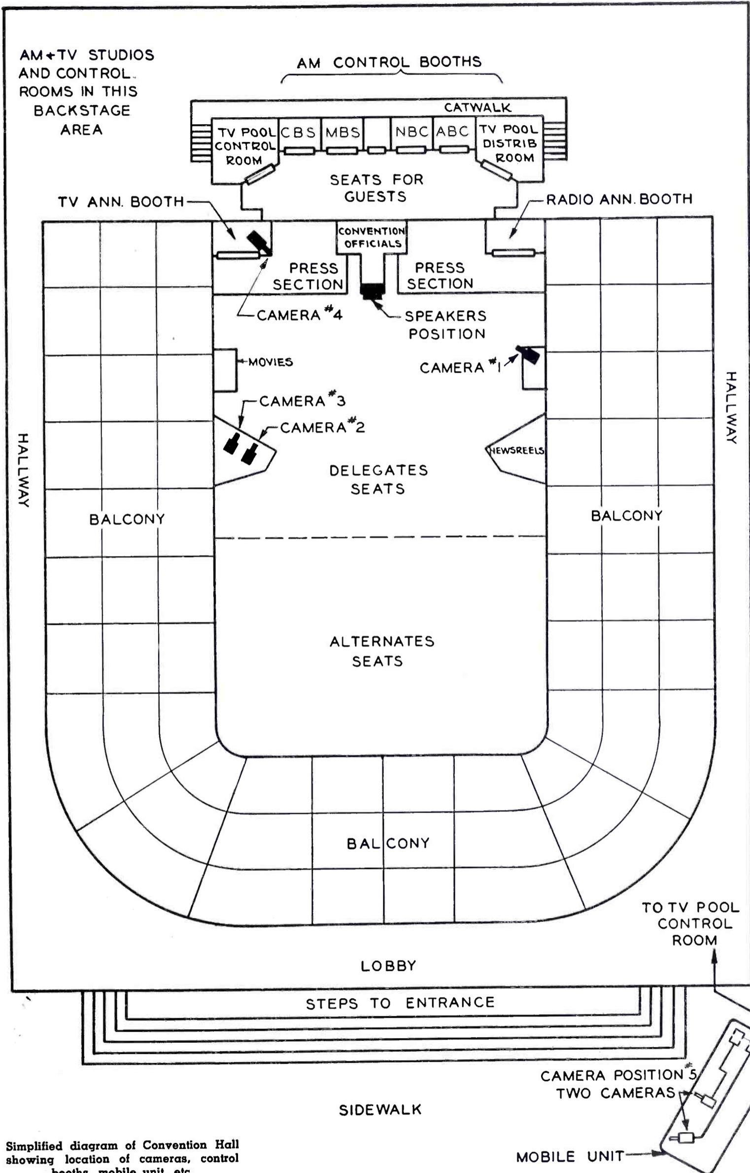
Simplified diagram of Convention Hall showing location of cameras, control booths, mobile unit, etc.
