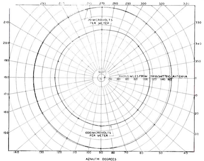
FIG. 15 (below). Curve for eight-section Pylon illustrating close-in radiation strength versus distance. In this case, the Pylon is erected on top of a very steep 5000 foot mountain.
