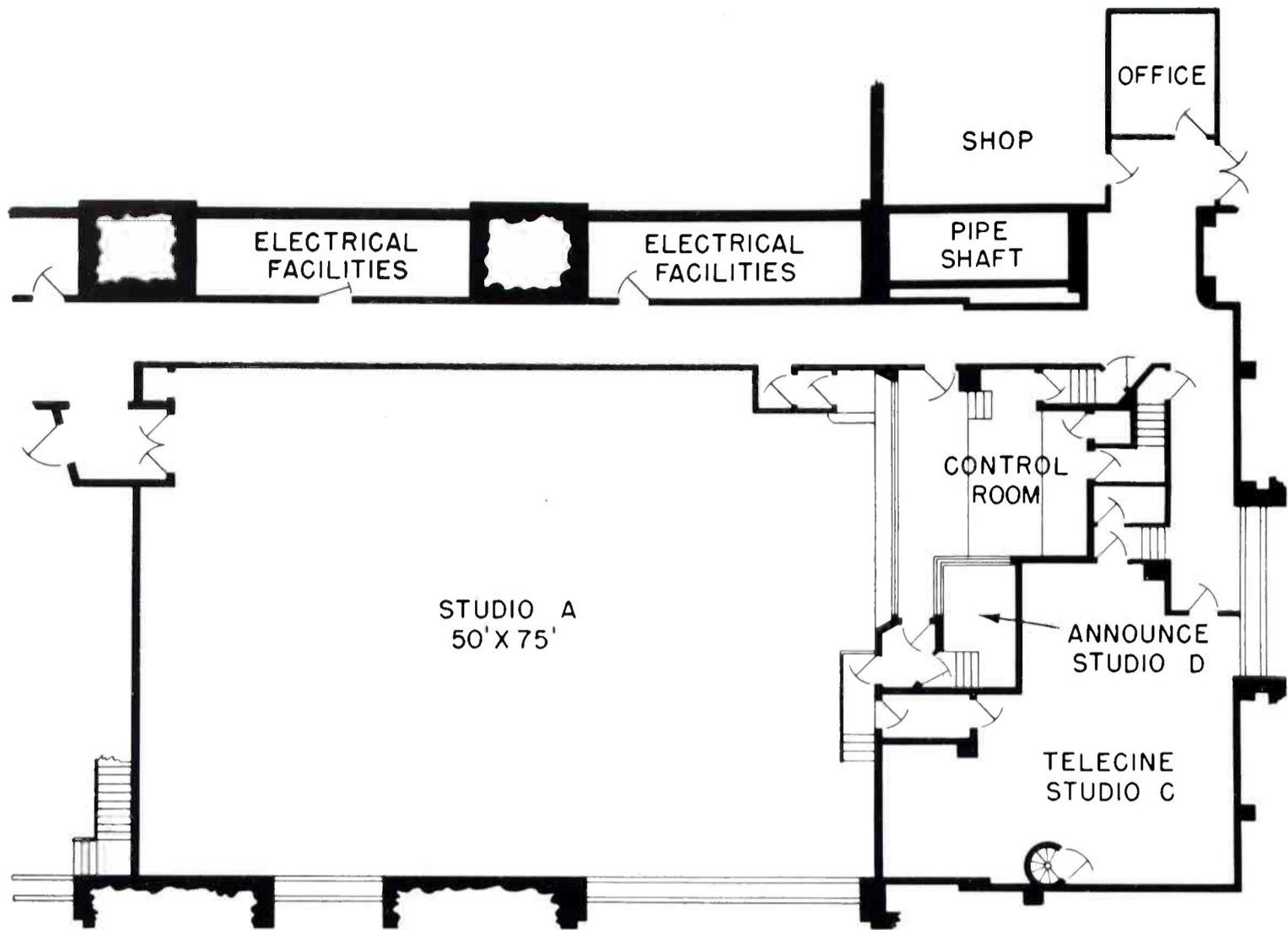
FIG. 3. Floor plan of Studio A showing relative position of Control Room A, Announce Studio D, and Telecine Studio C. Equipment in the control room is arranged on three levels in same relative manner as that of Control Room B (see Fig. 5). Arrangement of the equipment in the Telecine Studio C is shown in Fig. 9.
