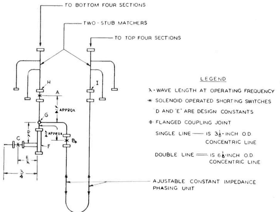
connected at junction "F" during four-section operation thus causes negligible change of input impedance and power loss. The input impedance to the antenna system is thereby maintained at very nearly  $51.5 + j0$  ohms during four- or eight-
