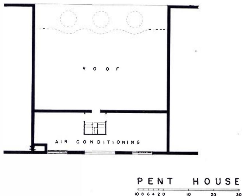
FIG. 5 (right). This is a suggested design for the "penthouse" of the large TV building. Space for air-conditioning equipment is provided in addition to certain details which are added solely for decorative effect.
