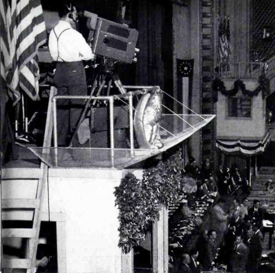
NO. 4 CAMERA POSITION (at left) was on top of the booth built for the TV commentator. This elevated position, at the left front of the stage, commanded an exceptional view of the whole hall (approximately the same view as that shown in the illustration at the bottom of page 59). It was particularly useful when it was desired to show overall activity on the floor of the hall. Camera is an RCA TK-30A, furnished by NBC and operated, for the pool, by an NBC cameraman.
