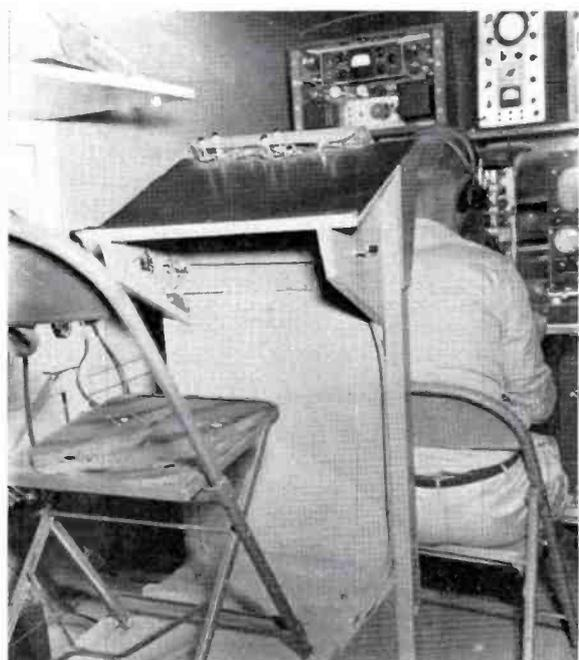
Unusual feature of the KING-TV mobile unit is a "producer's podium" (above) located directly behind camera control position. Note two buttons on floor of podium used for switching cameras. (Look Ma, no hands!)
