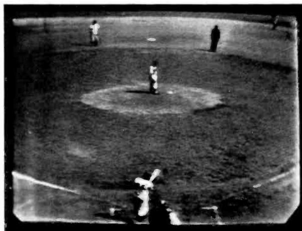
**5** With a man on 2nd base this shot, obtained with Zoomar full out, is used. It corresponds roughly to the field of view obtained with a 90mm lens.
