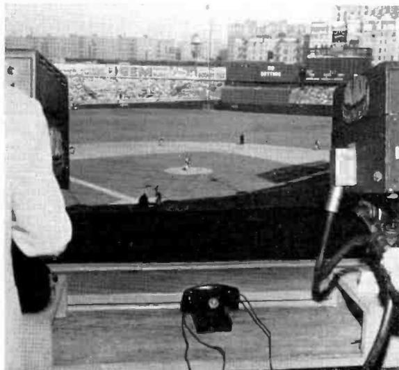
WABD's No. 2 and No. 3 Cameras are 40 feet high just a little to right of pitcher-batter line. Locating all three cameras at same horizontal helps orientation on fast camera switches.
