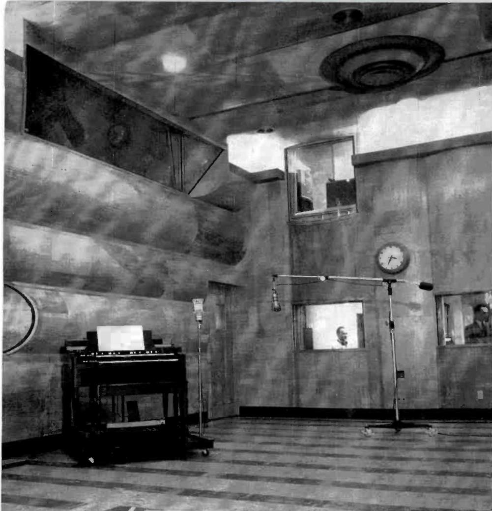
FIG. 6 (left). Interior of Studio A, largest in the KTBS group. Built to accommodate programs which require large casts, as well as live audiences, the studio will seat up to 75 persons. At top left is the studio's observation booth; at center are twin control rooms which sit atop each other; while at far right a partial view of the announcer's studio is shown. RCA 44-BX and 77-D microphones are used in the studios. 88A's in the control rooms.
