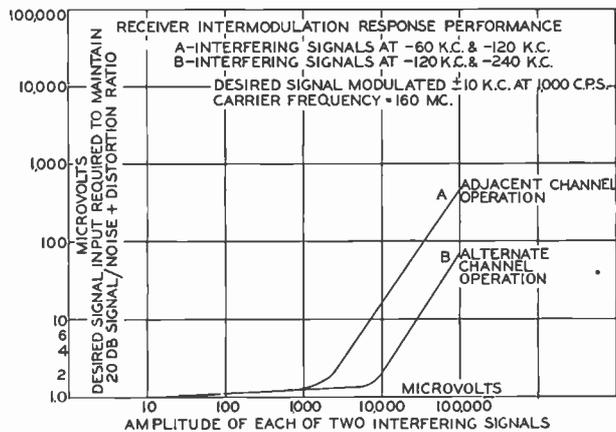
FIG. 16. Receiver intermodulation rejection.
