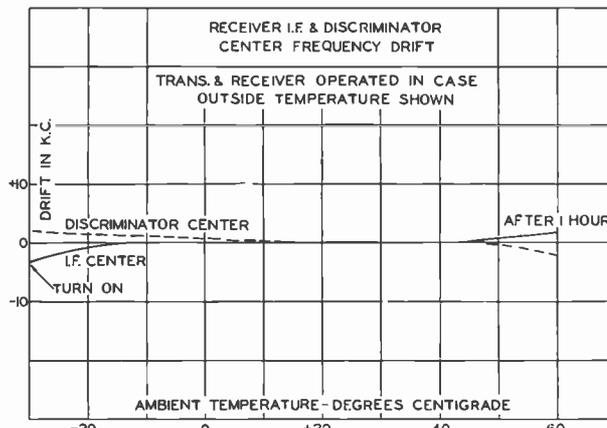
FIG. 17. Receiver intermediate-frequency drift.
