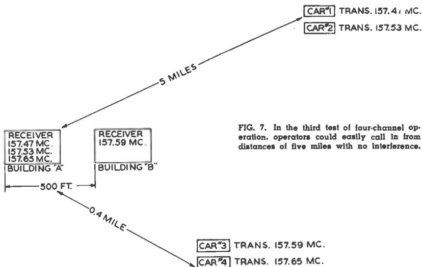
FIG. 7. In the third test of four-channel operation, operators could easily call in from distances of five miles with no interference.
