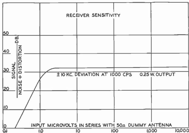
FIG. 14. Receiver sensitivity.
