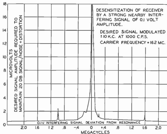
FIG. 15. Receiver spurious response rejection.
