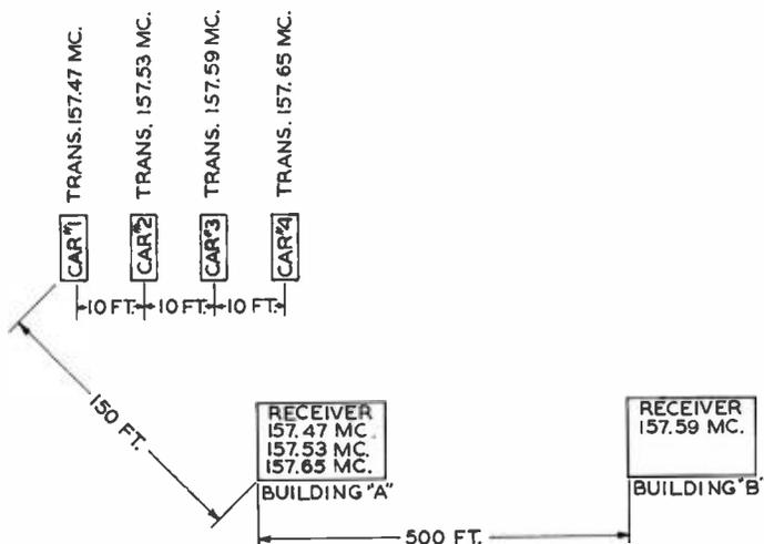
FIG. 6. During the second test of four adjacent channel operation with RCA mobile car radios on air, signals heard in each car were free of interference.
