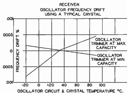
FIG. 18. Receiver oscillator stability.
