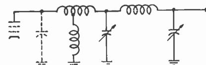
FIG. 20. Transmitter output filter circuit.
