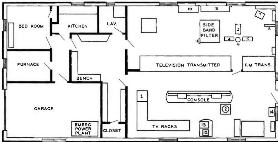
Diagram above is a floor plan layout of the WJAC-TV transmitter building. The transmitter console combines FM, TV and program control functions as described in the text.
