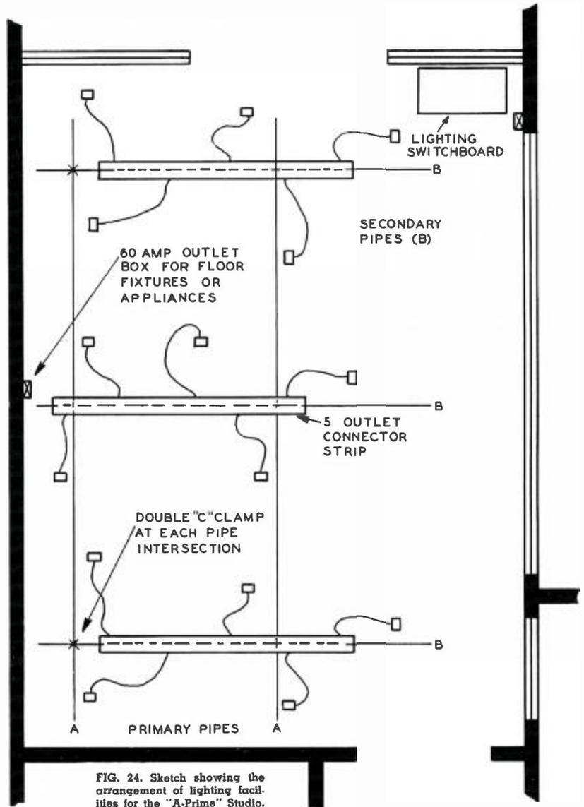
FIG. 24. Sketch showing the arrangement of lighting facilities for the "A-Prime" Studio.
