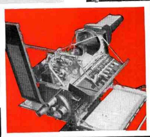
New accessibility puts every component at your fingertips. One latch opens both hinged sides and top. Dual bar handles provide better grip and easier carrying.
