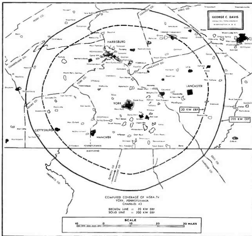
FIG. 3. Coverage map at the signal strengths of 20-KW ERP and 200-KW ERP.
