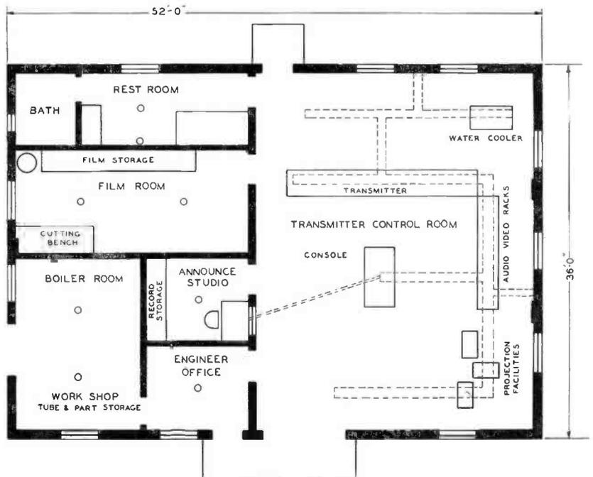
FIG. 4. Floor plan showing WKNB-TV's transmitter layout and facilities.
