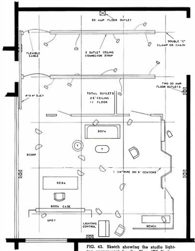
FIG. 43. Sketch showing the studio lighting arrangement for the Plan "B" Station.
