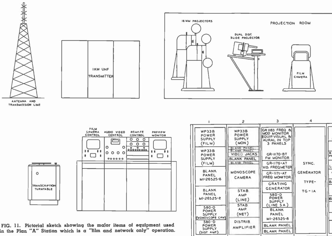
FIG. 11. Pictorial sketch showing the major items of equipment used in the Plan "A" Station which is a "film and network only" operation.
