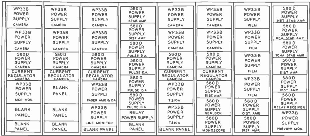
FIG. 50. Rack layout of the power supply equipment for Plan "C".
