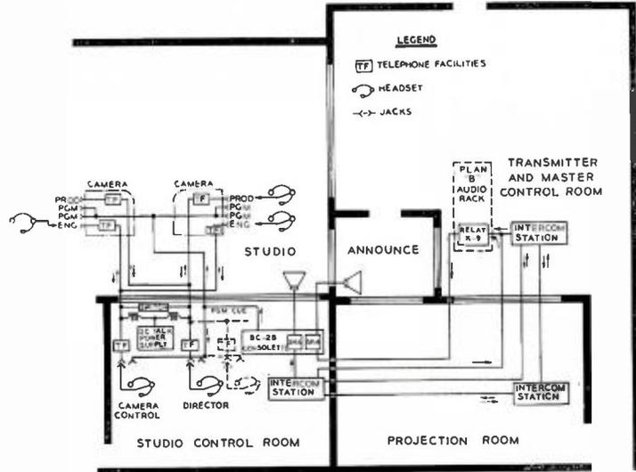
FIG. 42. "Intercom" "flow" diagram for Plan "B" Station.
