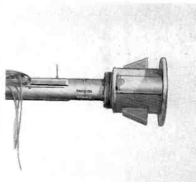
FIG. 10. Side view of Flange Pedestal Adapter fastened to base of UHF Pylon. Note hole in adapter near antenna base through which transmission line passes.
