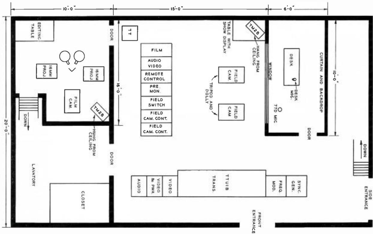
FIG. 2. Floor plan showing transmitter layout of WSBA-TV facilities.
