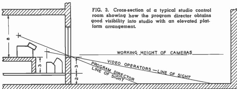
FIG. 3. Cross-section of a typical studio control room showing how the program director obtains good visibility into studio with an elevated platform arrangement.
