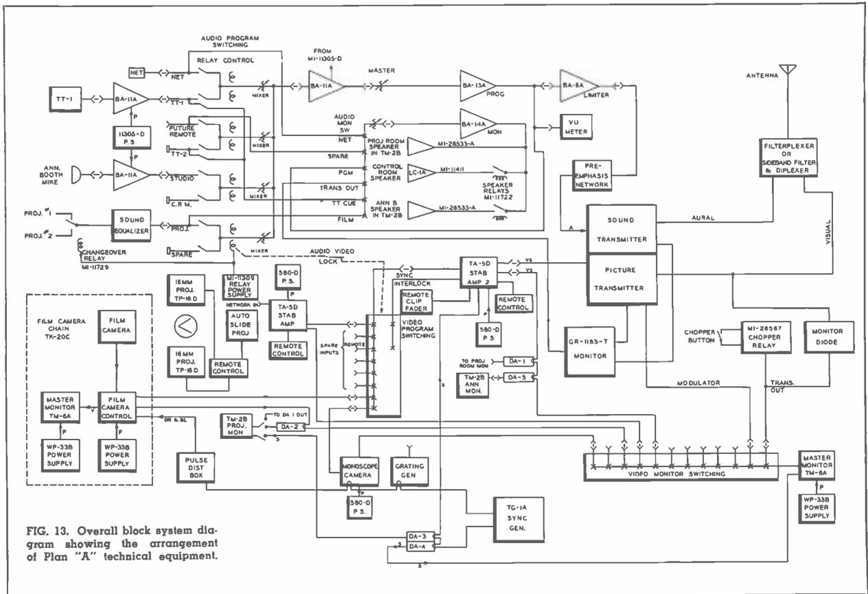
FIG. 13. Overall block system diagram showing the arrangement of Plan "A" technical equipment.
