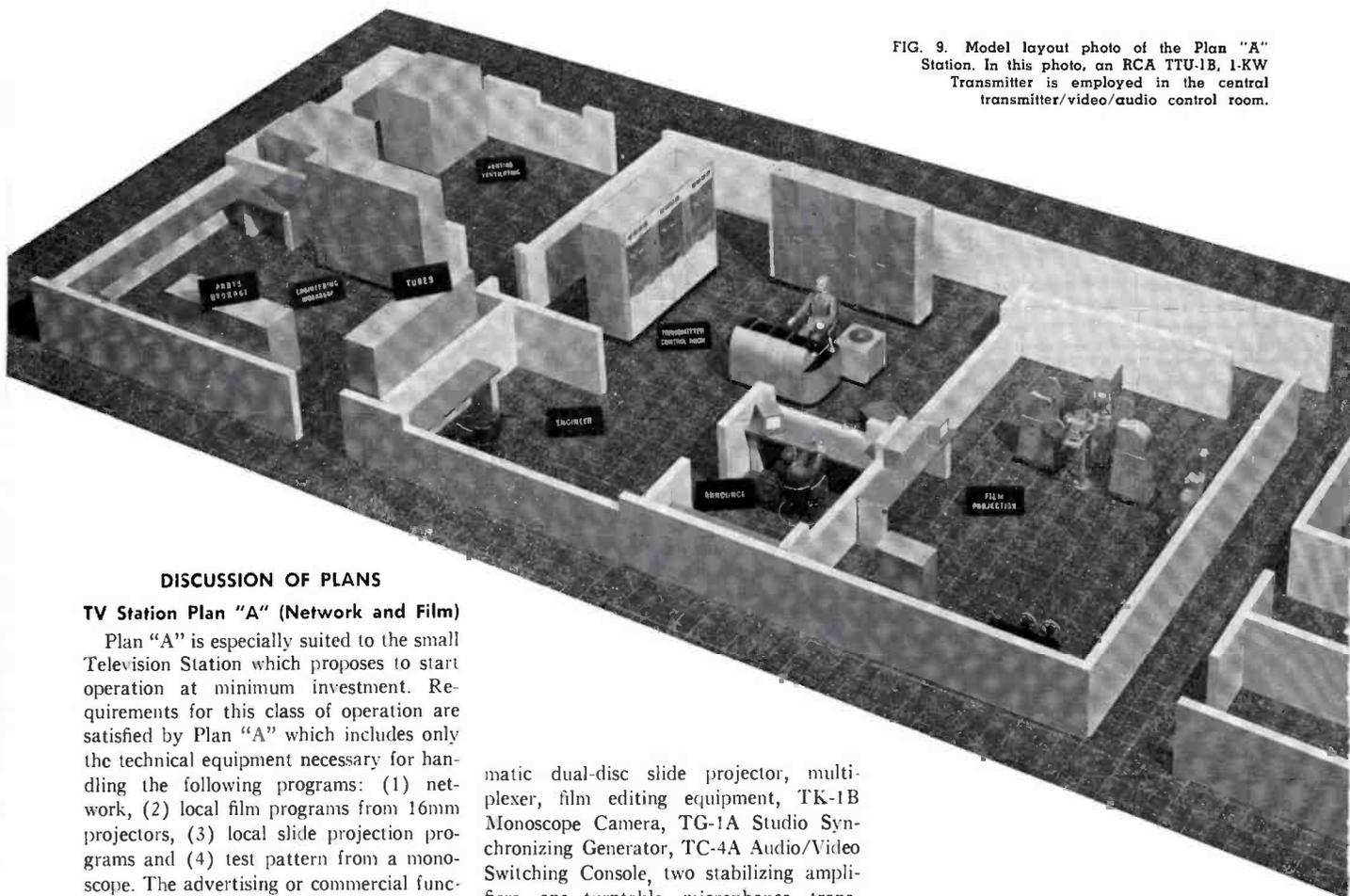
FIG. 9. Model layout photo of the Plan "A" Station. In this photo, an RCA TTU-1B, 1-KW Transmitter is employed in the central transmitter/video/audio control room.
