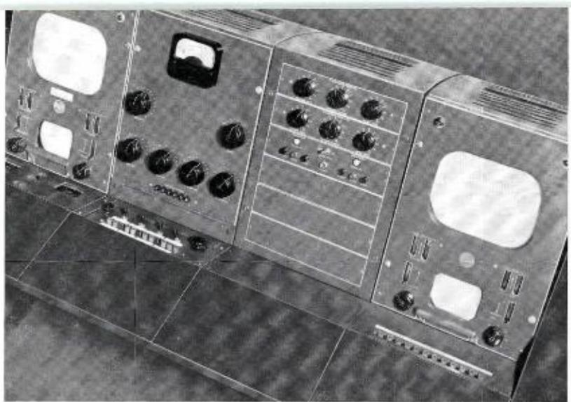
FIG. 4. Closeup of the four console sections which are used as the basic "building block" for the combination transmitter/master control rooms in all four plans.
