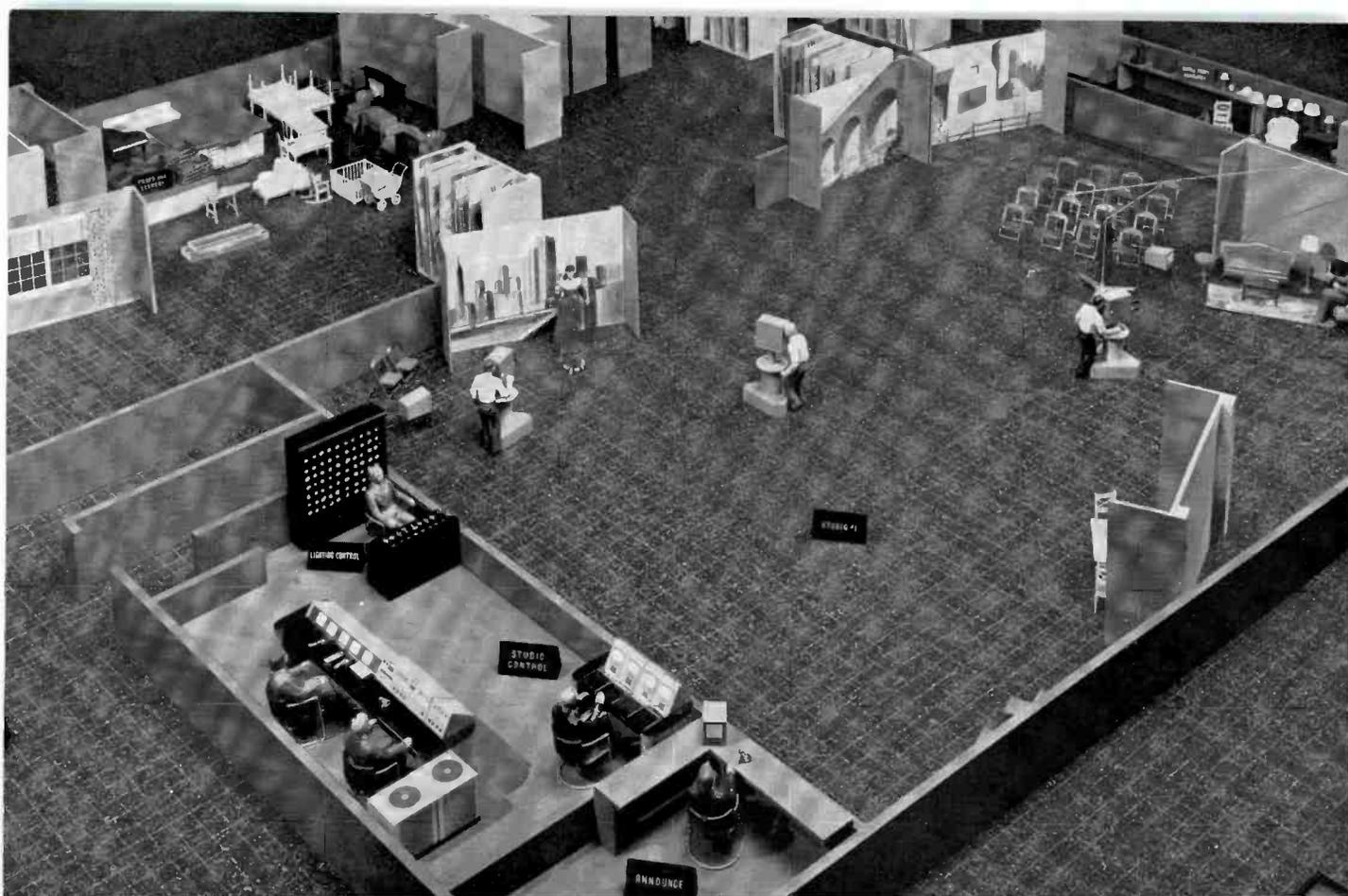
FIG. 52. View of large Studio #1, companion control room and the nearby "prop and scenery" storage area. Note that, in this setup which uses the TC-5A Program Director's Console, the video monitors have been located away from the control room window. The program director and audio operator are at a second level, with the lighting control operator and his equipment plus the video monitors at a lower level. (Actually these camera controls could be located in a different room.)
