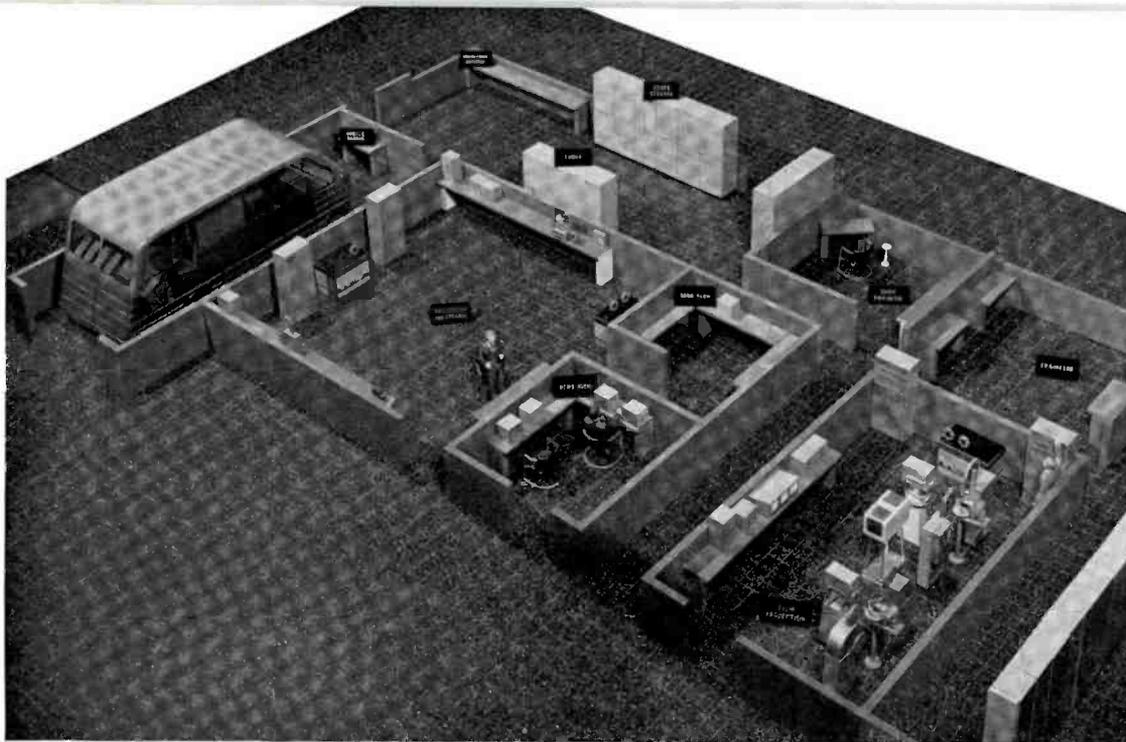
FIG. 45. Closeup showing the "left-hand" portion of the Plan "C" Station, including mobile unit, film editing and storage, news room, dark room, parts storage, film projection room, engineering workshop and engineers' offices.
