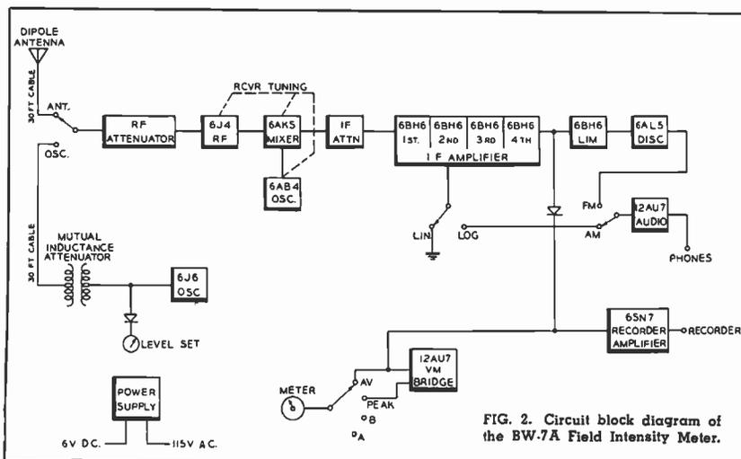
FIG. 2. Circuit block diagram of the BW-7A Field Intensity Meter.
