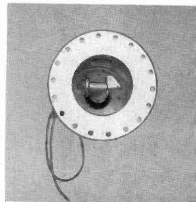
FIG. 11. Lower-end view of Flange Pedestal Adapter showing mitre-elbow in position for connecting with external transmission line.
