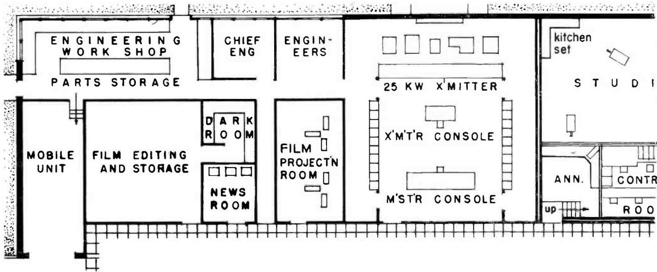
FIG. 46. Floor plan layout showing the technical facilities for the Plan "C" Station.
