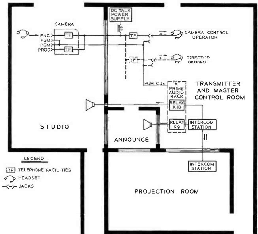
FIG. 22. "Intercom" "flow" diagram for the "A-Prime" Station.
