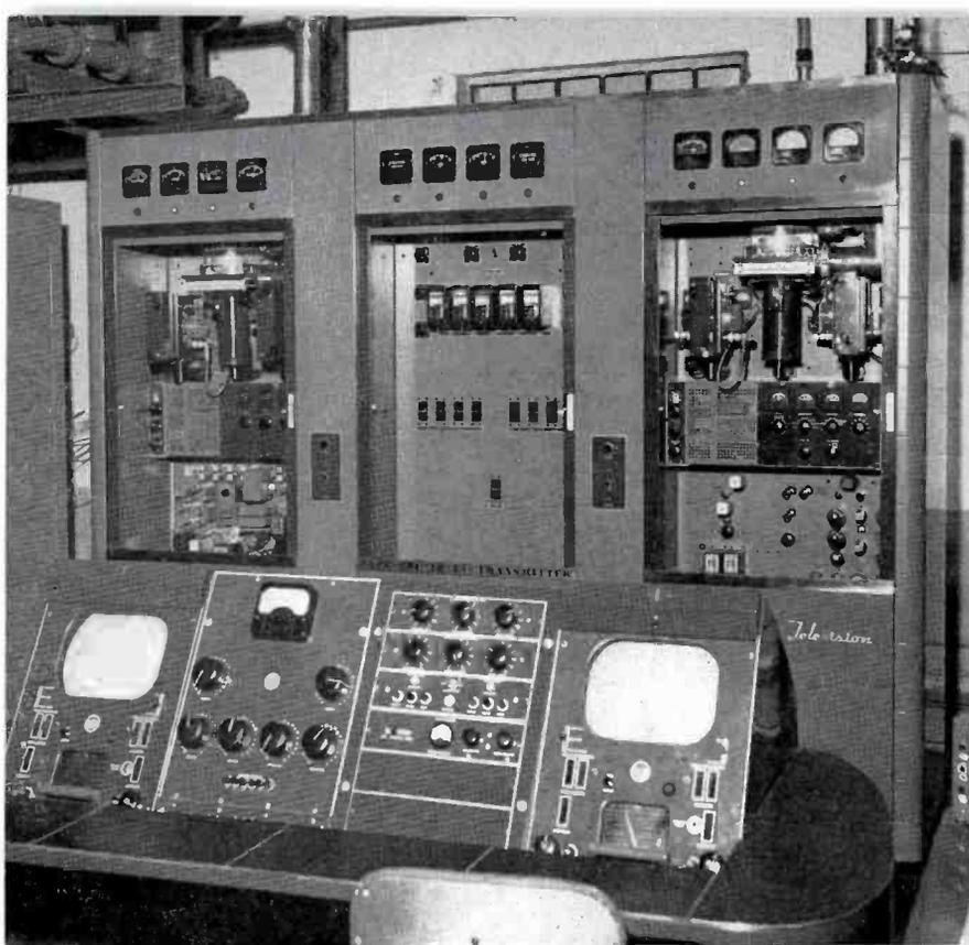
FIG. 4. Closeup of the RCA TTU-1B UHF television transmitter and TC-4A "Basic Buy" console—two excellent performers for UHF television broadcasting.
