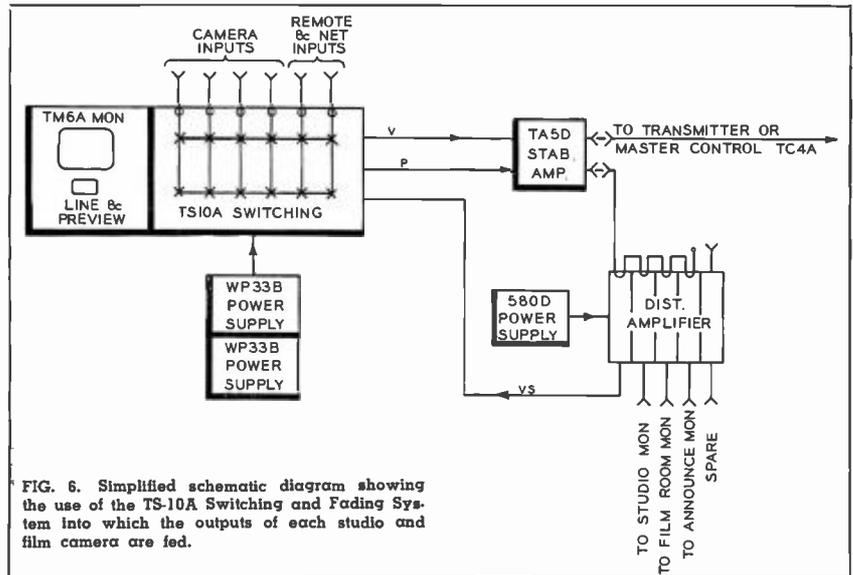
FIG. 6. Simplified schematic diagram showing the use of the TS-10A Switching and Fading System into which the outputs of each studio and film camera are fed.
