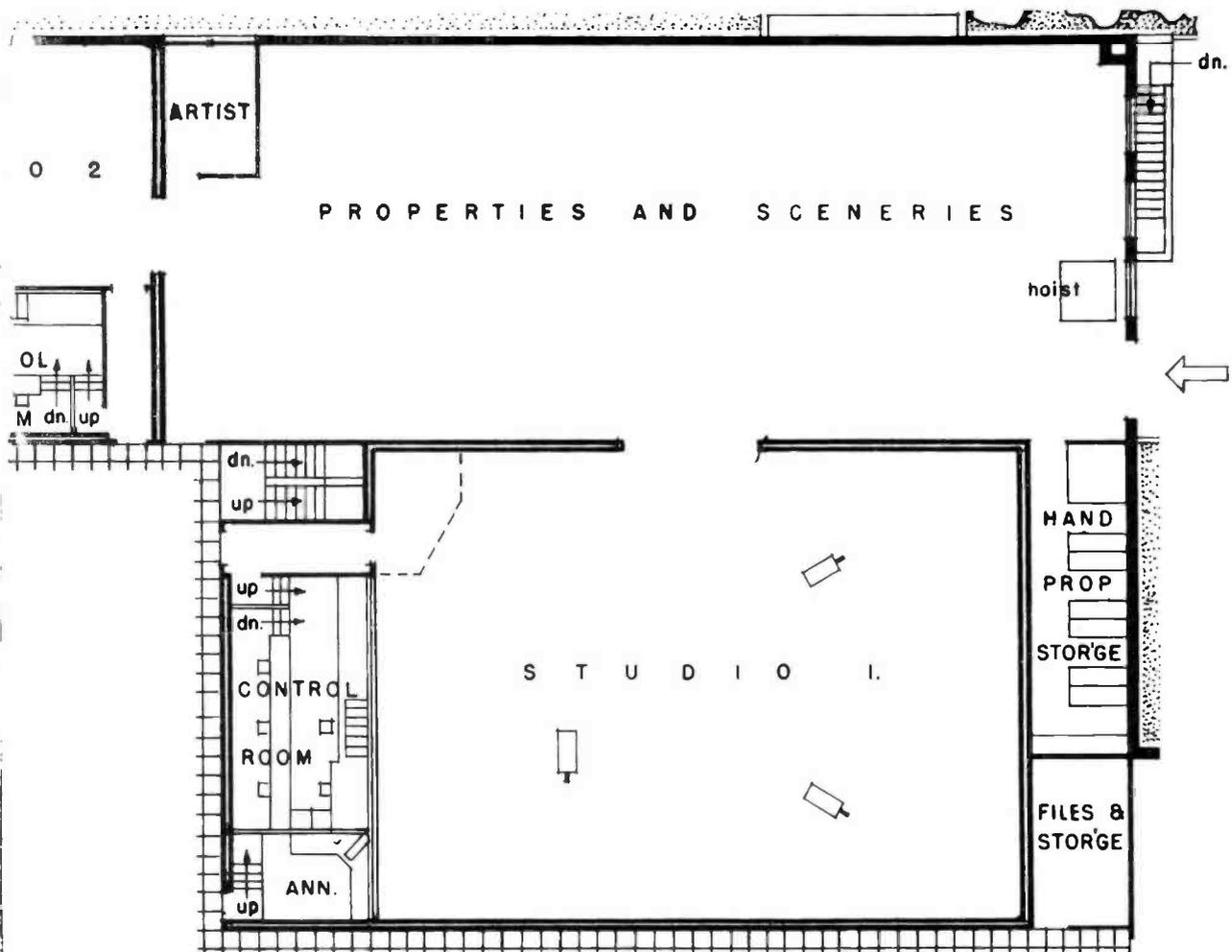
FIG. 48. "Right-hand" portion of the Plan "C" layout showing the two studios (#1 and #2), their associated control rooms and the properties and scenery space required. Note that an artists' room is located adjacent to the "prop" space.
