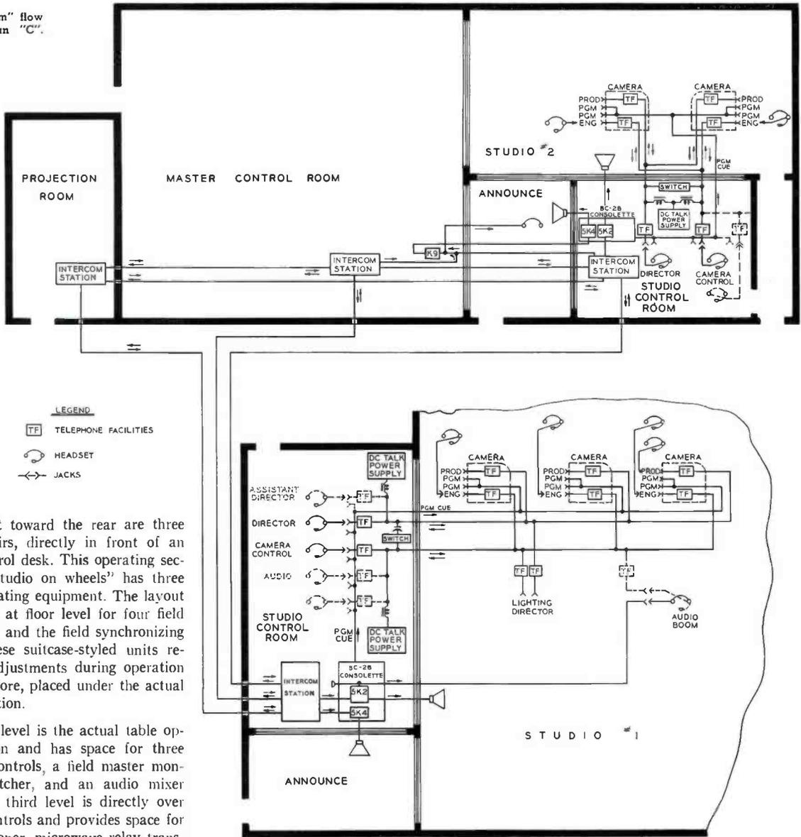
Director. Next toward the rear are three cushioned chairs, directly in front of an operating control desk. This operating section of the "studio on wheels" has three levels for operating equipment. The layout provides space at floor level for four field power supplies and the field synchronizing generator. These suitcase-styled units require a few adjustments during operation and are, therefore, placed under the actual operating position.
