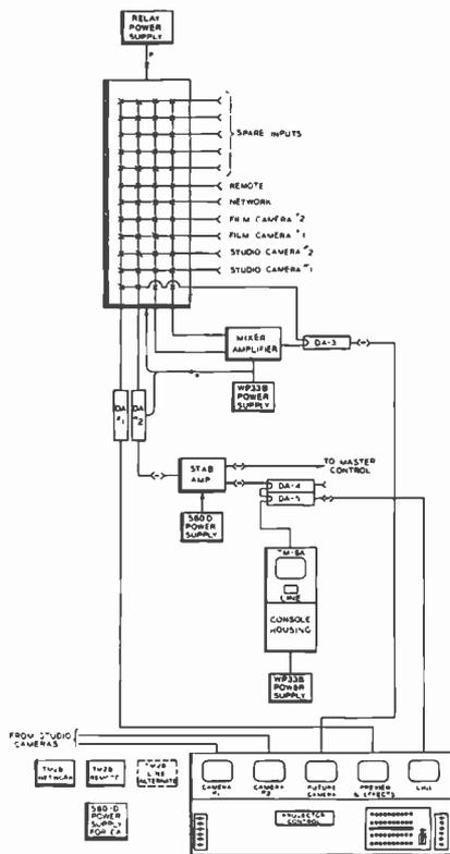
Some systems planners feel that further economy is necessary and, therefore, provide an inexpensive monitor on the outgoing lines and make the switchable one a TM-6A master monitor type, which has a high quality video system and a waveform monitor.
