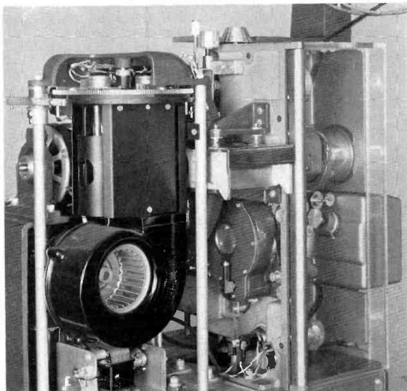
lamp change problems. The entire operation, from the failure of one lamp to the automatic replacement of a new lamp, takes place *in less than one second*. The effect when viewed on the monitor screen is negligible.
