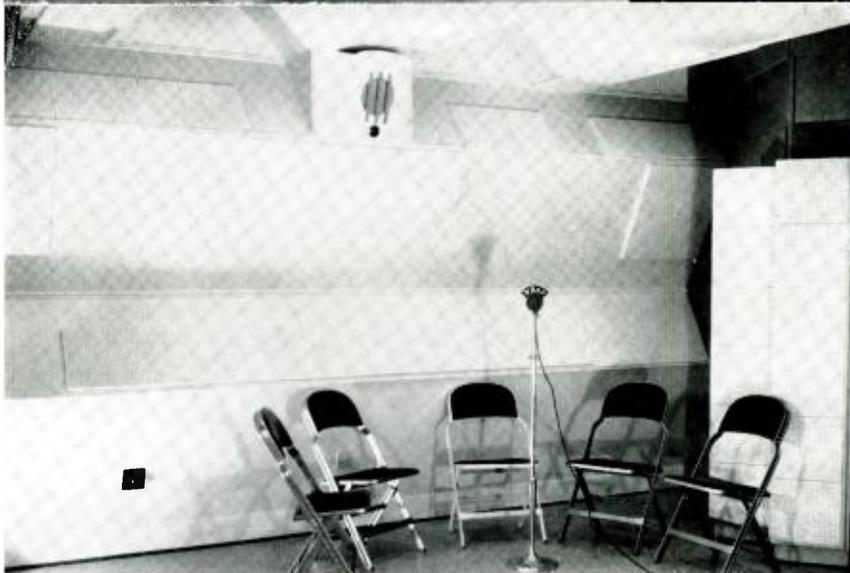
FIG. 29 (right). A corner of AM-FM Studio C which, like Studio D with which it is identical, is 17 feet by 26 feet by 11 feet high. In these studios, as in Studios E and F, acoustical treatment consists of splayed flat surfaces on walls and ceilings plus a calculated amount of acoustical absorbing material in irregular patches.
