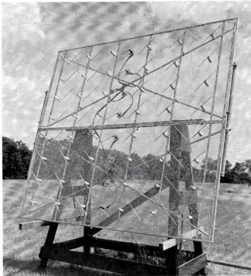
FIG. 12. This is a closeup view of the zig-zag receiving antenna before installation on the water tower shown in Fig. 2. It has a measured beam width of 16° (both vertical and horizontal) and a gain of 20.5 db.
