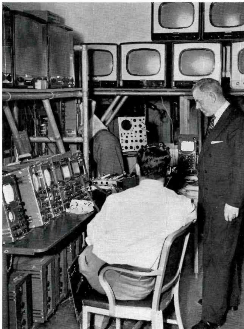
FIG. 1. Richard H. Hooper, RCA's Promotion Manager, shown inspecting equipment at control center before recent closed-circuit demonstration for American Telephone and Telegraph Company. Note standard broadcast equipment including field camera controls, field switchers and oscilloscope used in operations. TV receivers above served as large screen monitors for the program director.
