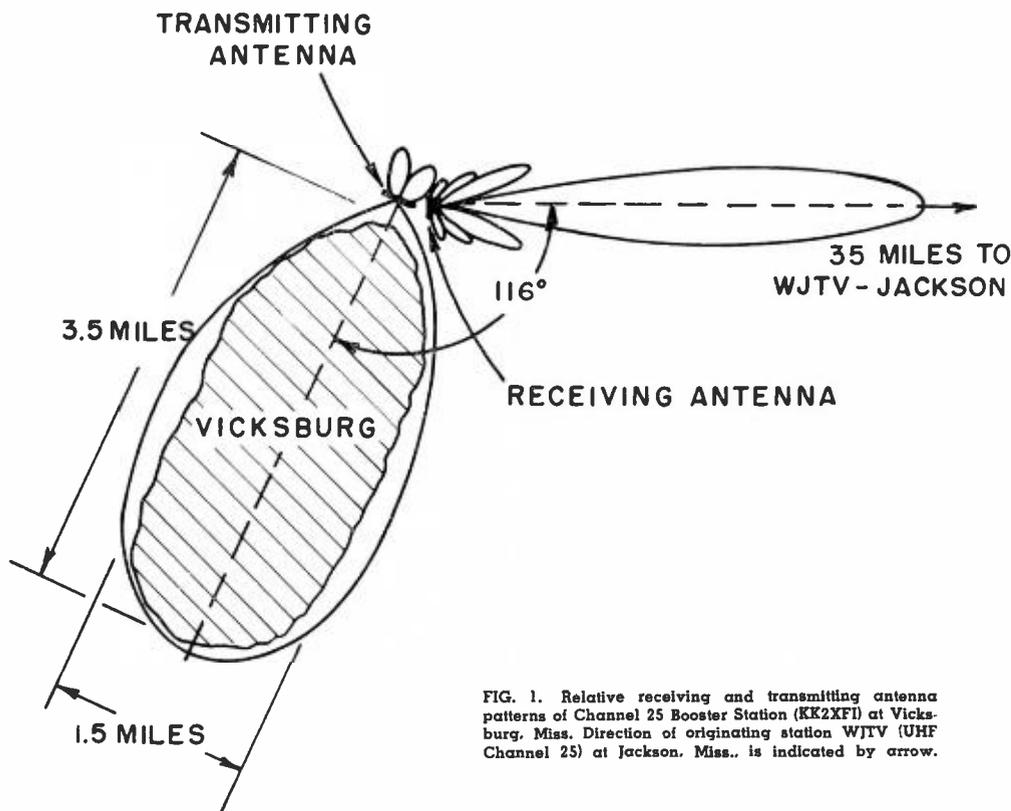
FIG. 1. Relative receiving and transmitting antenna patterns of Channel 25 Booster Station (KK2XFI) at Vicksburg, Miss. Direction of originating station WJTV (UHF Channel 25) at Jackson, Miss., is indicated by arrow.
