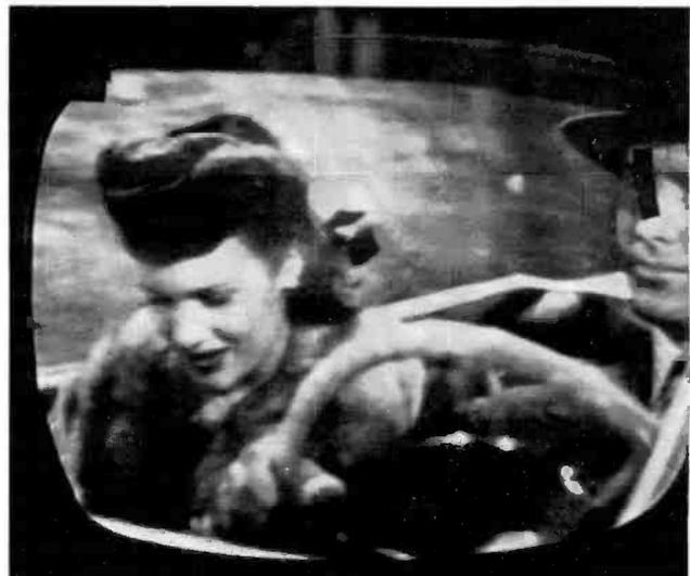
FIG. 4 (right, center). Picture received from booster station KK2XFI with the bow-tie antenna shown in Fig. 2 directed toward booster.
