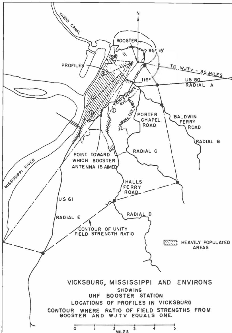
FIG. 3 (left). Map of Vicksburg and surrounding area showing the location of the booster station, profiles along which measurements were made, and approximate contour of equal field strengths (KK2XF1 and WJTV).
