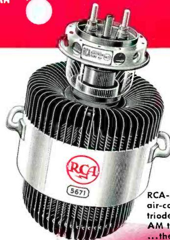
RCA-5671—forced-air-cooled power triode for 50-KW AM transmitters...the power tube with thoriated-tungsten filament.
