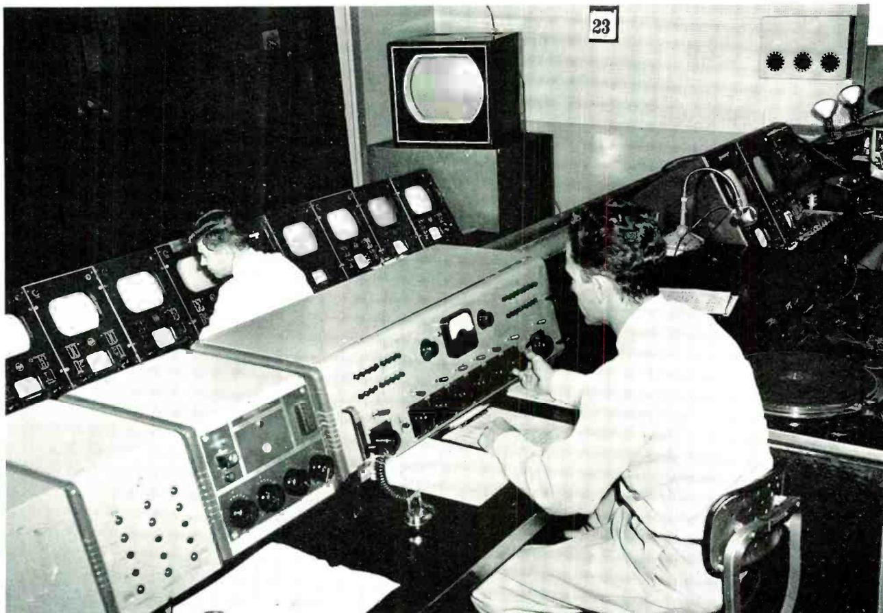
FIG. 11. WKY-TV's Control Room B. On lower level are camera control units for monochrome cameras in both B and C studios. On upper level is the audio console (foreground), the program director's position (center) and the master control position (upper right).
